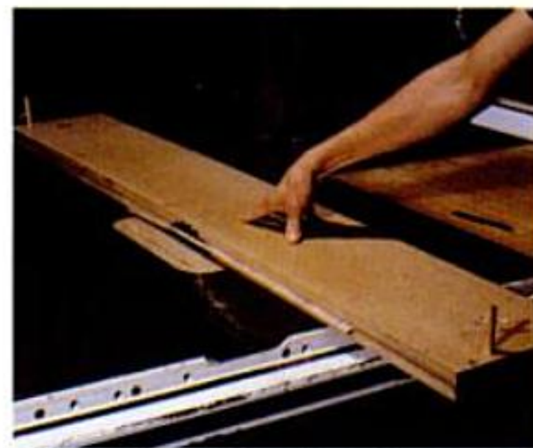
Ripping it straight. The author's jig rips straight edges on stacked sheets of veneer. A wood runner on the bottom of the jig rides in the tablesaw's miter groove.
