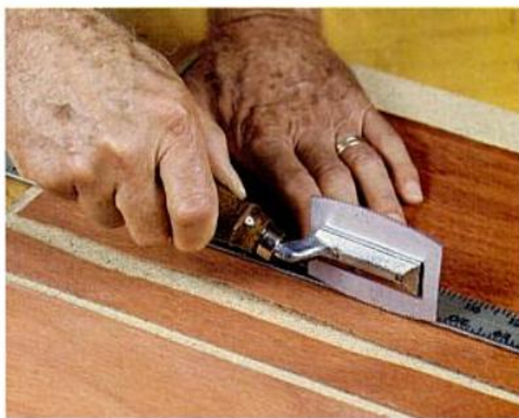
Sawing to size. A veneer saw will rip and crosscut veneer to size quickly and cleanly.
