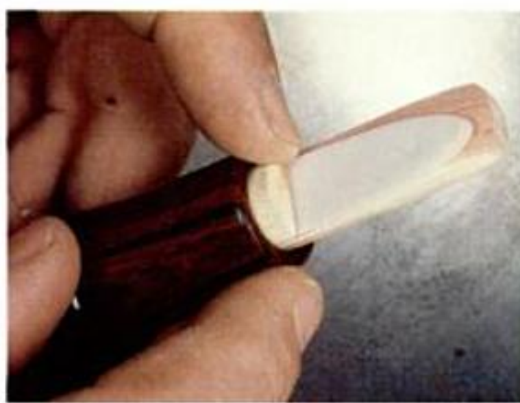
Assembling the call. The reed covers the sounding block's groove and is sandwiched between the block and the wedge. All three parts fit snugly in the tapered tube.
