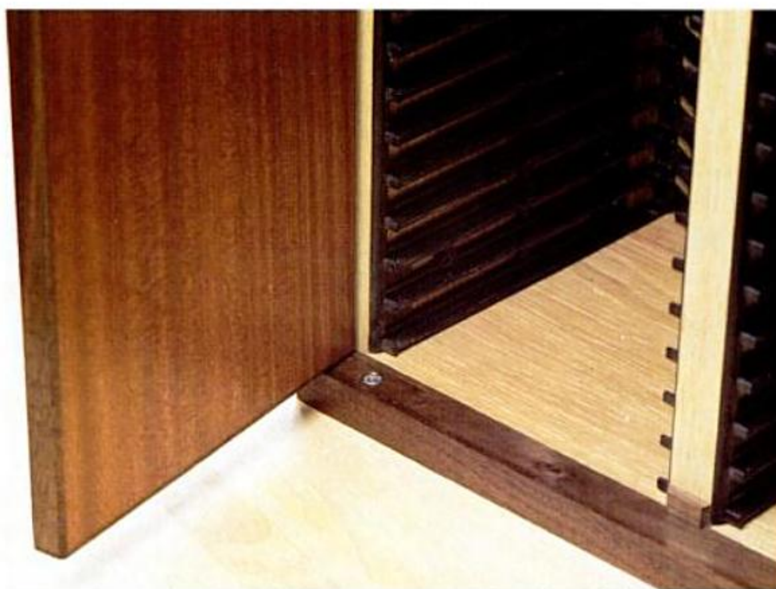
Shop-made knife hinges. A single screw secures the walnut blade of this unobtrusive hinge to a routed slot in the bottom edge piece.
