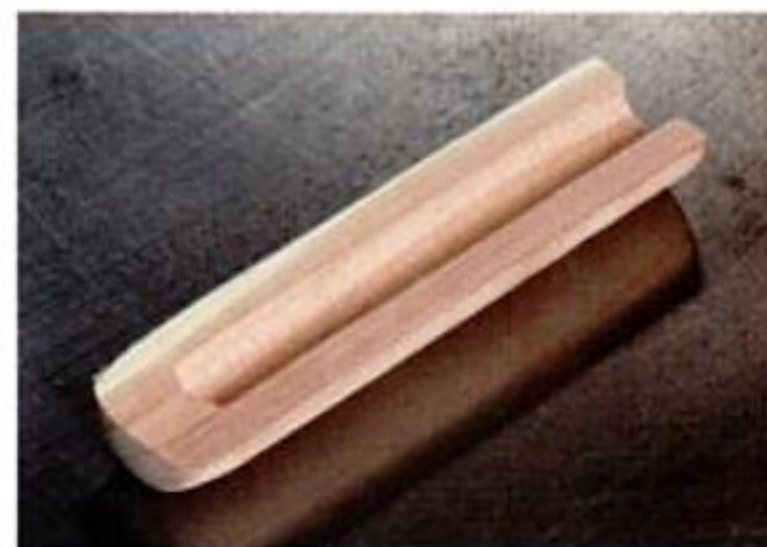
Halving the sounding block. Left, secure the blank to a V-block with tape, and guide the block's edge against the bandsaw's rip fence to make the cut. Above, the finished sounding block has a stopped groove and a slightly rounded end.
