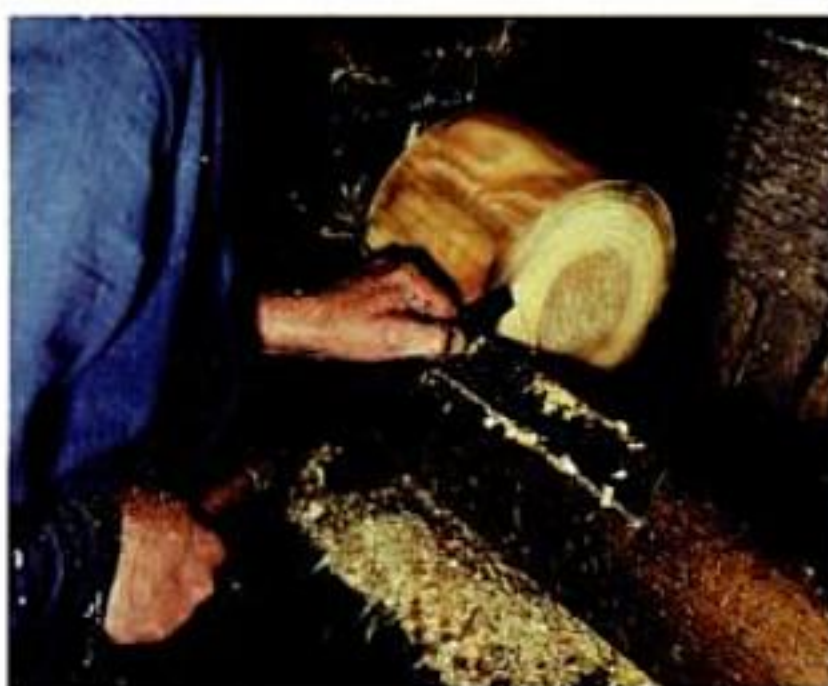
Starting with a tree. The blank is a knot-free wet spruce log, about 1 ft. long, mounted in a special ring chuck. The turner first shapes the delicate contours of the animal's legs and underside.
