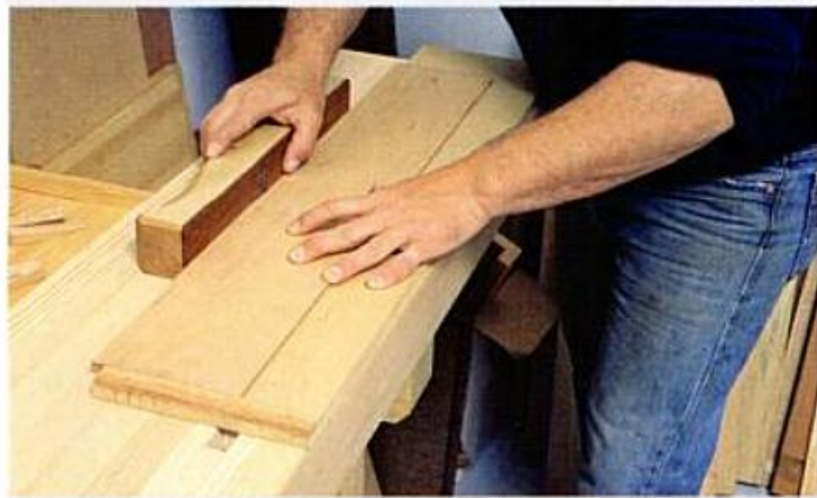
Shootin' straight. Janofsky straightens and squares the edges of his veneer with a homemade plane and a simple shooting board.
