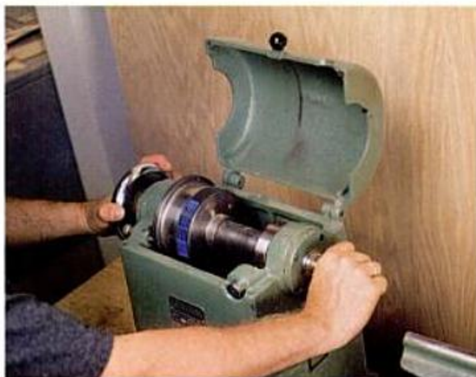
Wiggle the shaft. Play in the shaft is a sure sign of worn bearings. To check for play, grab the inboard and outboard ends and wiggle. If you detect play, or a "clunk," there's a problem.
