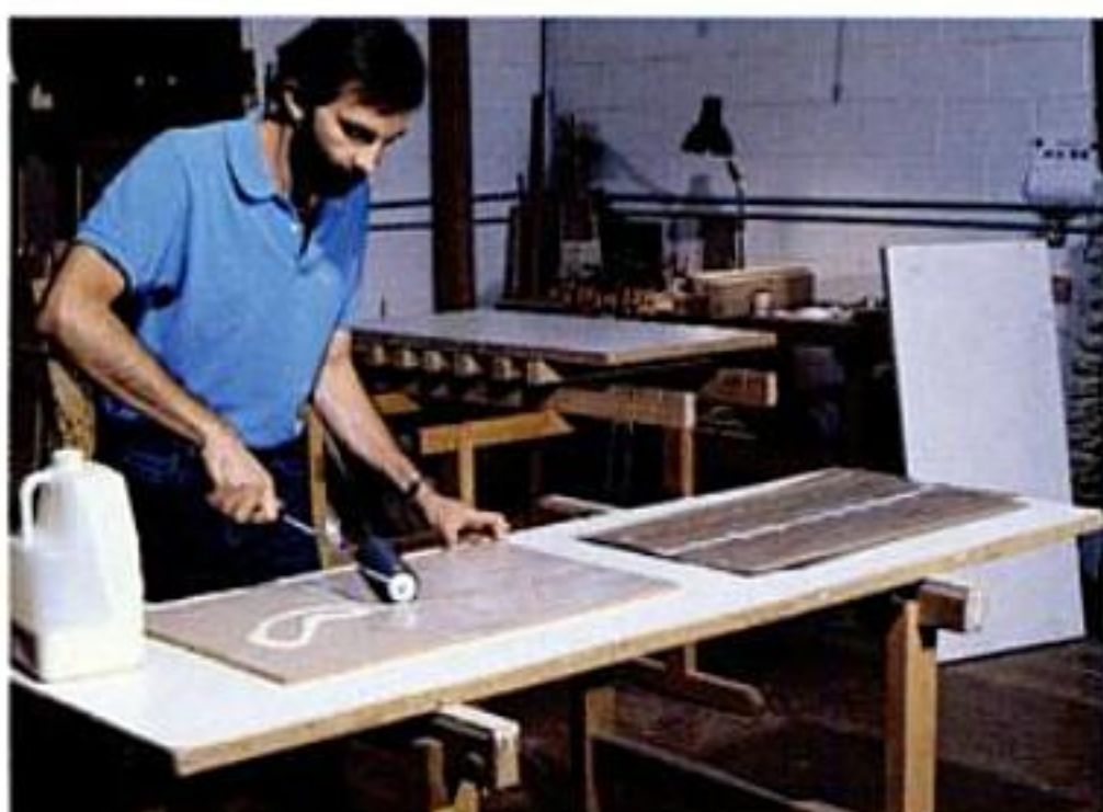
Glue-up. The author uses a foam roller to coat the substrate. In the background, Ghaffari's press awaits the veneered panel.
