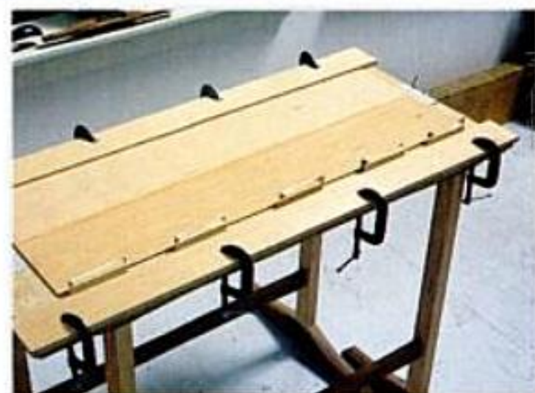
Wedging it together. Tapping pairs of wedges together creates enough pressure to glue veneers edge-to-edge.
