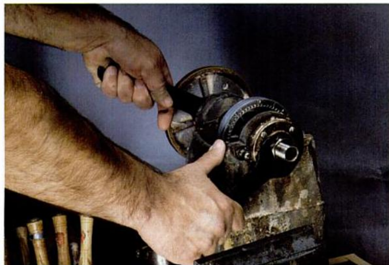
Taking the play out. On lathes with tapered bearings, spindle-shaft play can often be eliminated by tightening the load nut slightly.
