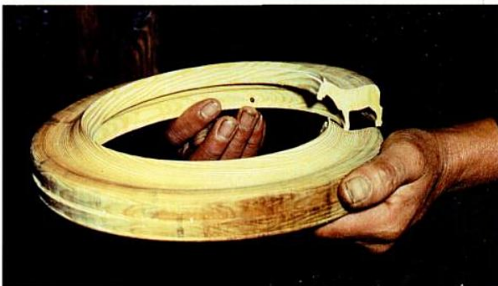
Horses in a ring. Split with a sharp knife, the finished profile reveals the turner's skill. This ring will yield 40 to 60 animals.
