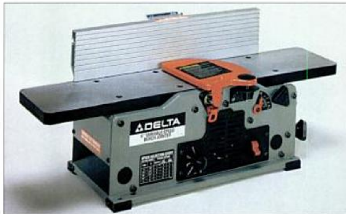
Portable and affordable. A benchtop jointer has a shorter bed but is less expensive and more portable than a floor model.
