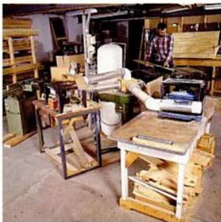
Improving dust collection efficiency. Left: Ductwork distances are short when the dust collector is positioned centrally, as in this basement shop. Center: A custom-made collection hood, like the one for this radial arm saw, increases the efficiency of your dust collector where it counts most—near the cutting edge. Right: Charlie Mastro's adjustable, drop-down hood serves as a combination dust collector and tablesaw blade guard. The clear plastic creation slides up and down inside a ceiling-mounted plywood box that is hooked up to the collector.
