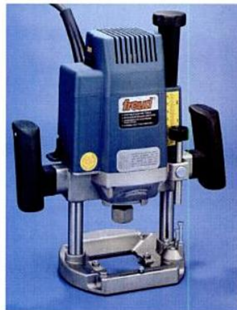
Taking the plunge. A pair of plunge posts are common to all plunge routers. These machines can lock at any point on their plunge range. A three-step turret, combined with a depth-control rod mounted above it, facilitates plunge cuts to different depth settings.
