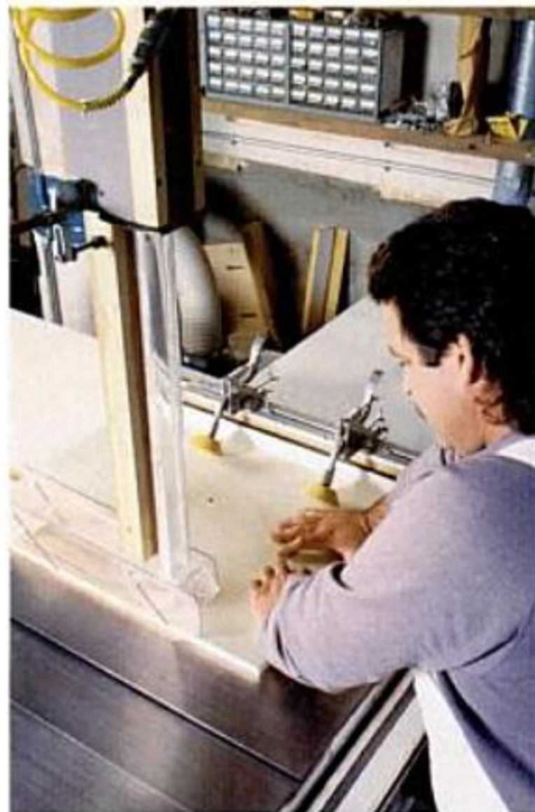
Improving dust collection efficiency. Left: Ductwork distances are short when the dust collector is positioned centrally, as in this basement shop. Center: A custom-made collection hood, like the one for this radial arm saw, increases the efficiency of your dust collector where it counts most—near the cutting edge. Right: Charlie Mastro's adjustable, drop-down hood serves as a combination dust collector and tablesaw blade guard. The clear plastic creation slides up and down inside a ceiling-mounted plywood box that is hooked up to the collector.
