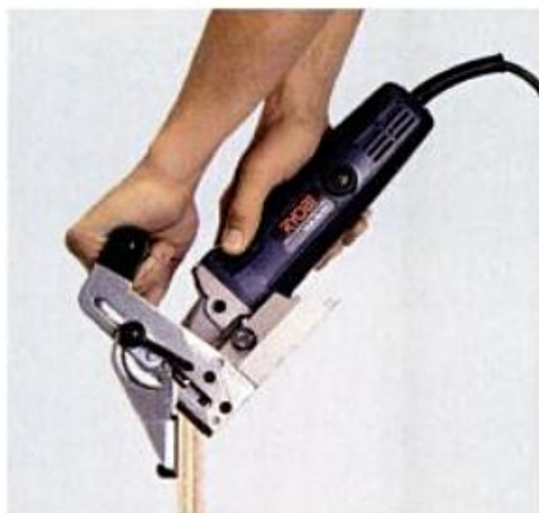
Fence-angle adjustments. Biscuit-joiner fences work in different ways to align cuts in miter joints. At left: A fixed 45° fence registers against the inside face of the work. Center and right: Adjustable fences capture the beveled edge of the miter.
