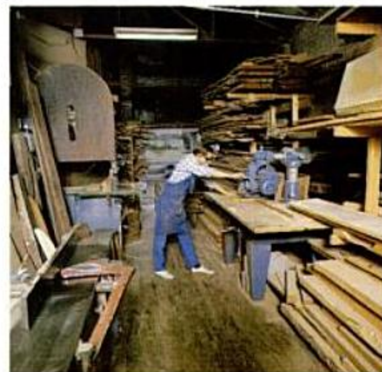
An efficient corridor. Not far from where lumber is off-loaded and stored, Kelly Mehler has work stations for dimensioning boards on their way to becoming furniture. Stock is cut to length on the radial arm saw, resawn on the bandsaw, and face-planed and jointed on the jointer.
