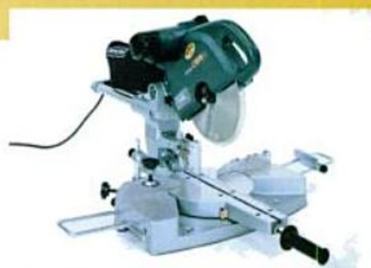
Sliding compound-miter saw. On a sliding compound-miter saw, the blade swings, tilts and pivots like a compound miter saw but also slides to cut wider stock.
