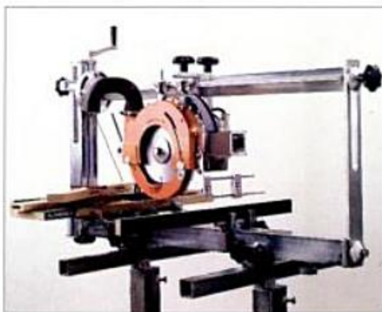
A closed-frame saw. On the Eumenia 811, a vertical bar provides greater upper-arm rigidity.
