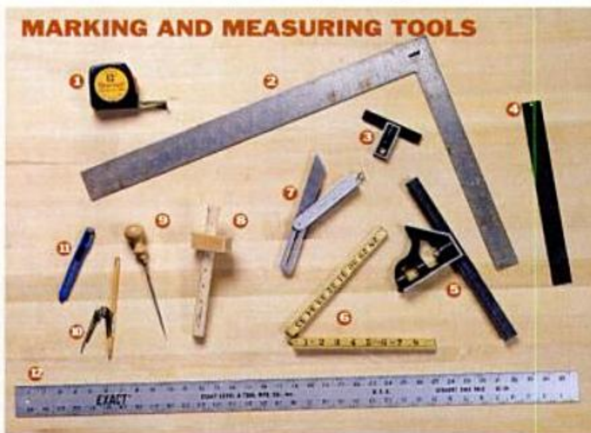
1: 12-ft. tape measure. 2: Framing square. 3: 4-in. sliding-blade square. 4: Cork-faced steel ruler. 5: 12-in. combination try square. 6: 3-ft. wooden folding ruler. 7: Adjustable sliding bevel. 8: Marking gauge. 9: Awl. 10: Pencil compass. 11: Marking knife. 12: 3-ft. straightedge.
