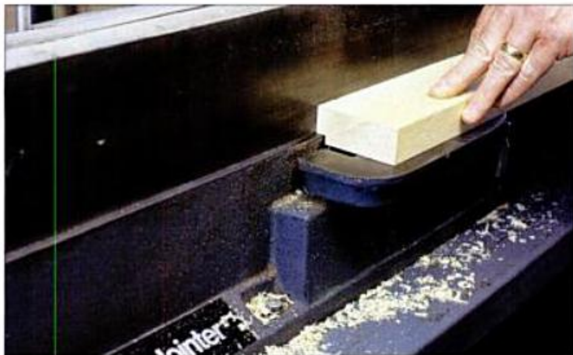
Rabbeting on the jointer. Rabbits and tongues can be milled on jointers equipped with a rabbeting ledge.
