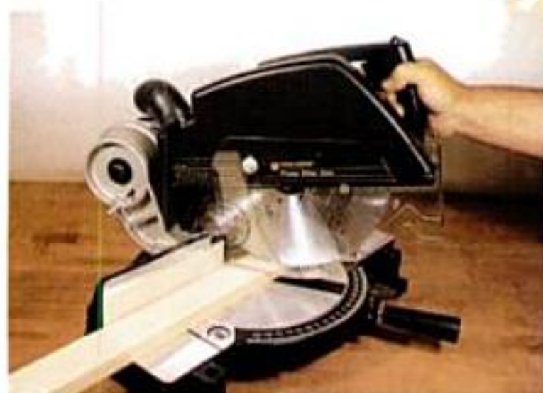
Conventional miter saw. On this type of miter saw, the blade swings left or right to the desired angle and pivots down to make cuts.
