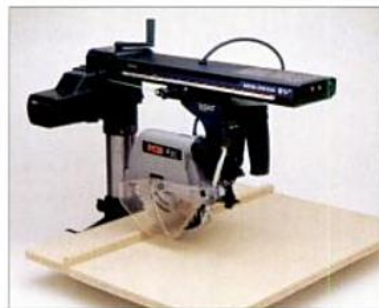
The benchtop option. This single-arm Ryobi has a carriage-advance control that also retracts the motor after a cut.
