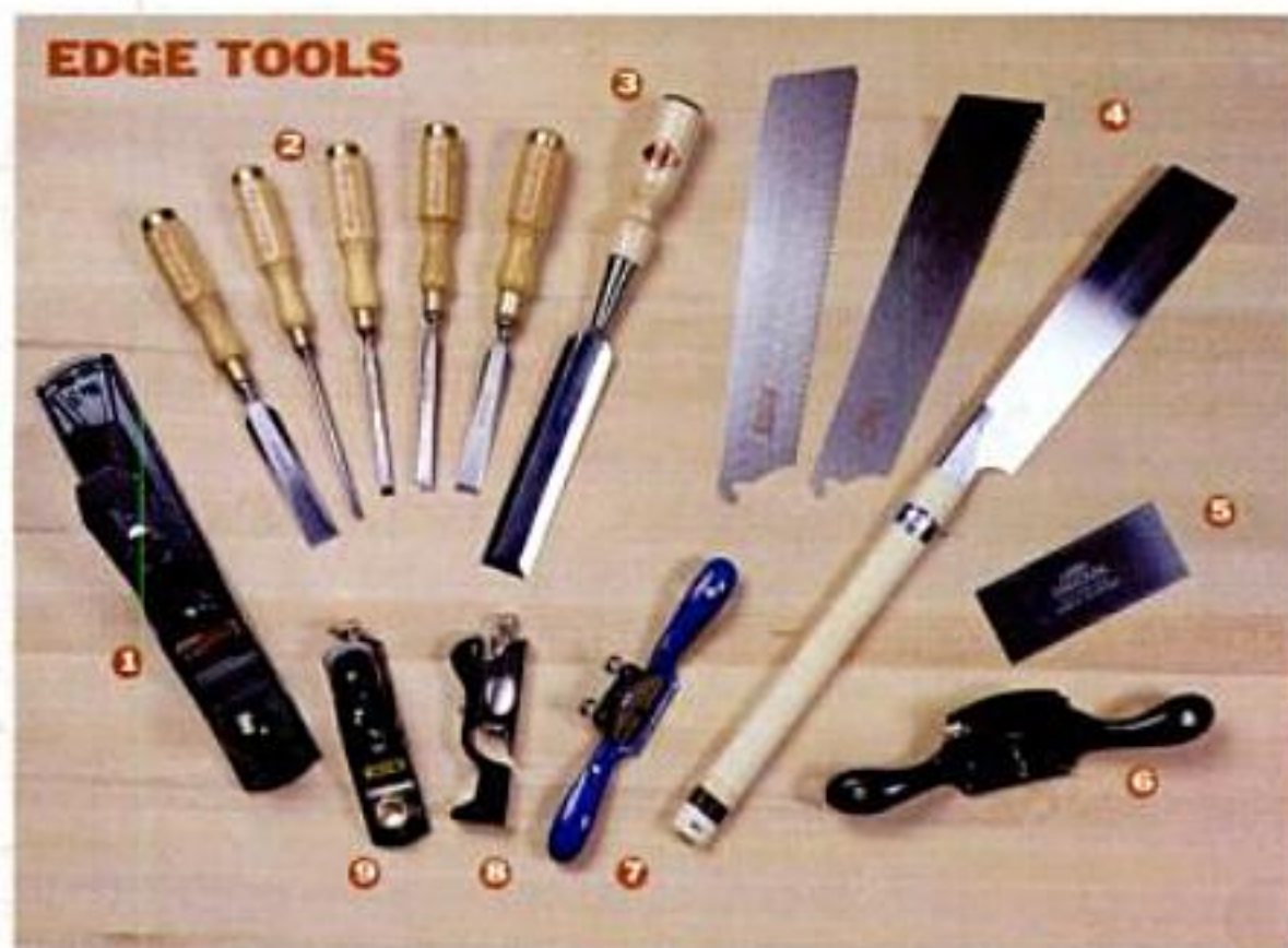
1: Jack plane. 2: Bevel chisels. 3: Firmer chisel. 4: Japanese saw (with interchangeable blades). 5: Hand scraper. 6: Cabinet scraper. 7: Flat-soled spokeshave. 8: Rabbet plane. 9: Low-angle block plane.
