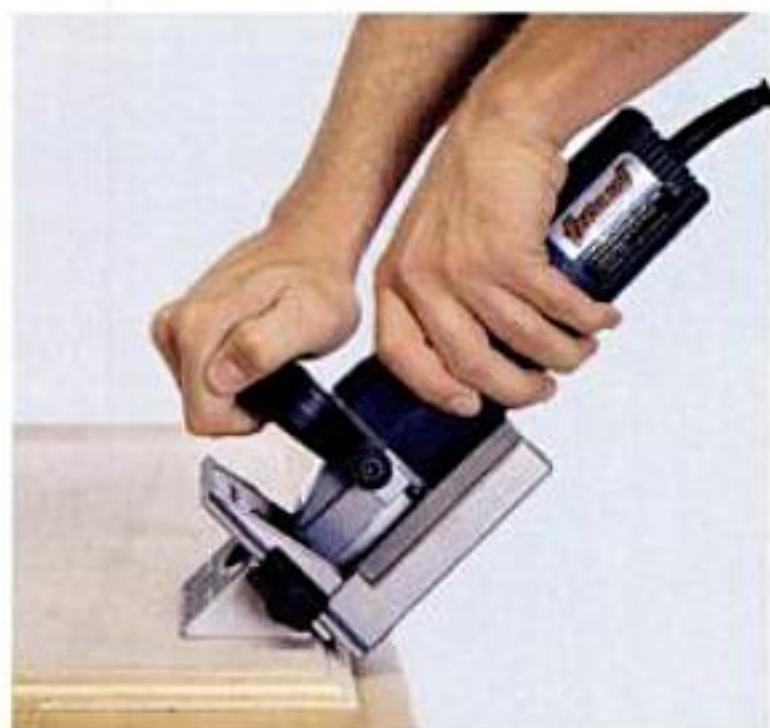
Fence-angle adjustments. Biscuit-joiner fences work in different ways to align cuts in miter joints. At left: A fixed 45° fence registers against the inside face of the work. Center and right: Adjustable fences capture the beveled edge of the miter.
