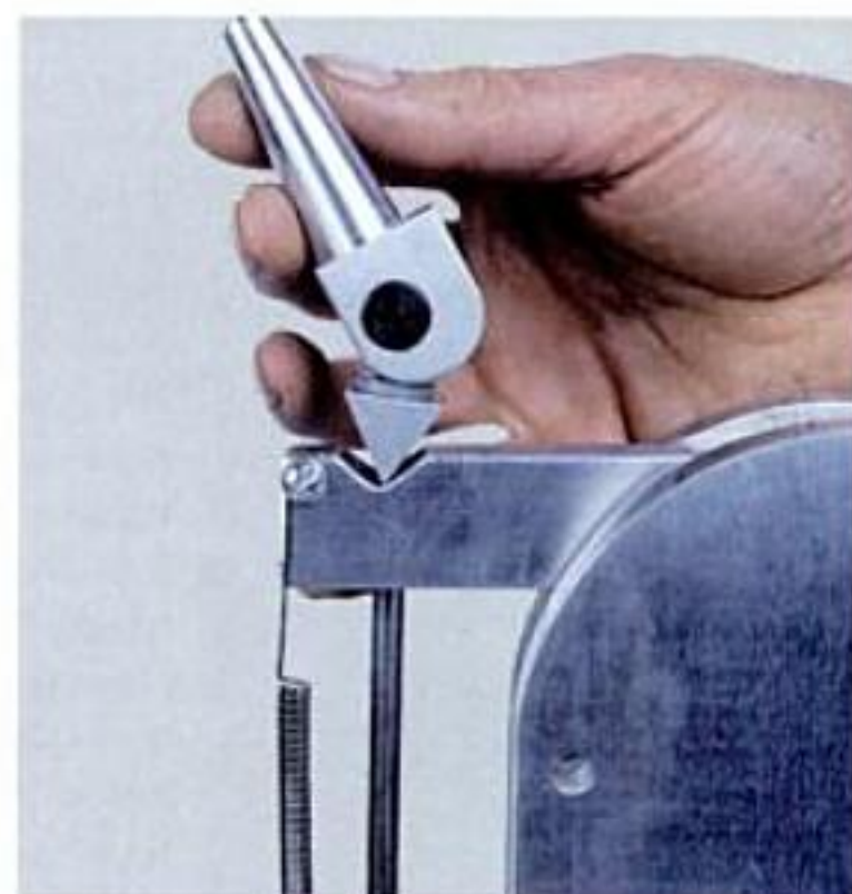
Stress relief. A quick-tension-release lever at the rear of saw arms facilitates blade tensioning.
