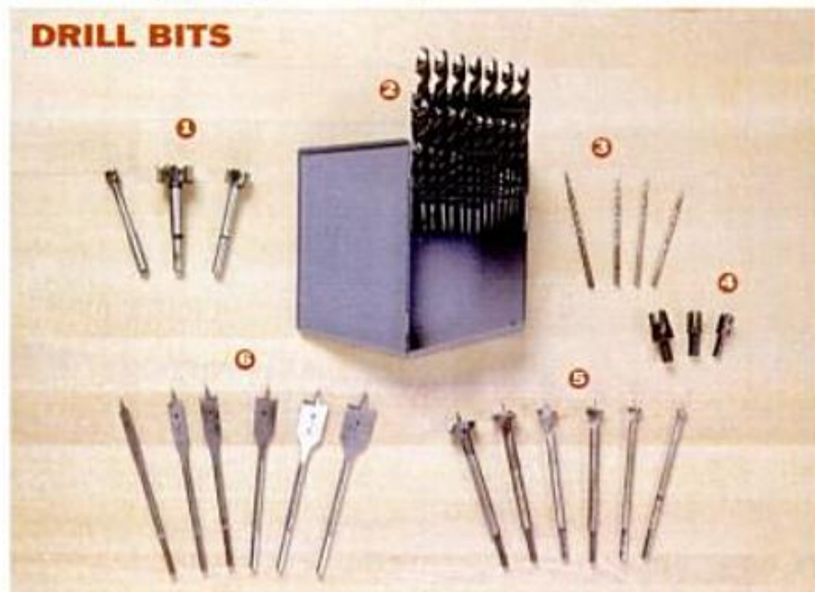
1: Forstner bits. 2: Twist drill set. 3: Taper drills. 4: Plug cutters. 5: "Powerbore" bits. 6: "Speedbor" bits.
