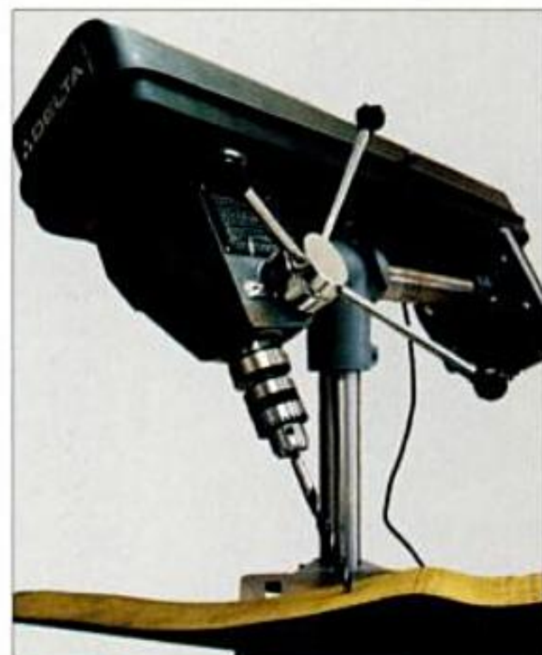
The radial drill press. The tube which holds the head assembly can spin on its column and tilt in either direction, making this type of drill press extremely versatile.
