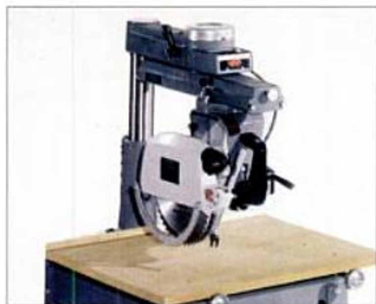
Turret arm. Radial arm saws with a double, or "turret" arm offer full table capacity for mitering.
