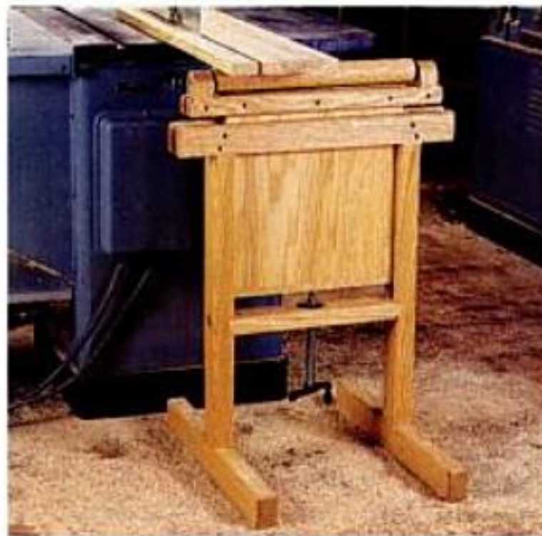
Extending your reach. Extension rollers and tables are a must for handling oversized material, especially if you're working solo. In some cases, it makes sense to build permanent extension tables (left). Adjustable-height extension rollers (center) will adapt to most machines. At right, woodworker Scott McBride shows that it pays to be height-sensitive. A guide board, placed on a lower workbench, provides support for long boards. Ball-bearing rollers in a shop-made stand provide outfeed support.
