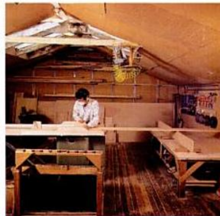
Extending your reach. Extension rollers and tables are a must for handling oversized material, especially if you're working solo. In some cases, it makes sense to build permanent extension tables (left). Adjustable-height extension rollers (center) will adapt to most machines. At right, woodworker Scott McBride shows that it pays to be height-sensitive. A guide board, placed on a lower workbench, provides support for long boards. Ball-bearing rollers in a shop-made stand provide outfeed support.
