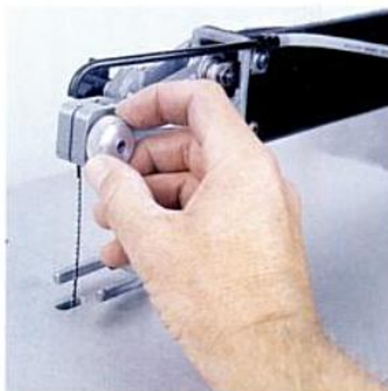
Blade-changing made easy. Finger-operated blade clamps allow tool-free blade-changing.
