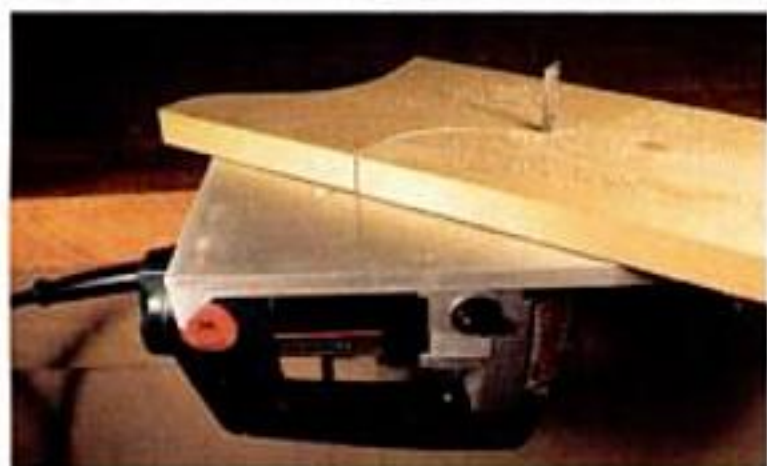
Stationary sawing. This bench-mounted inversion table turns a jigsaw into a sawing station.
