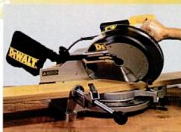
Compound miter saw. A compound miter saw's blade pivots and swings like a conventional saw's and can also tilt to cut compound angles.
