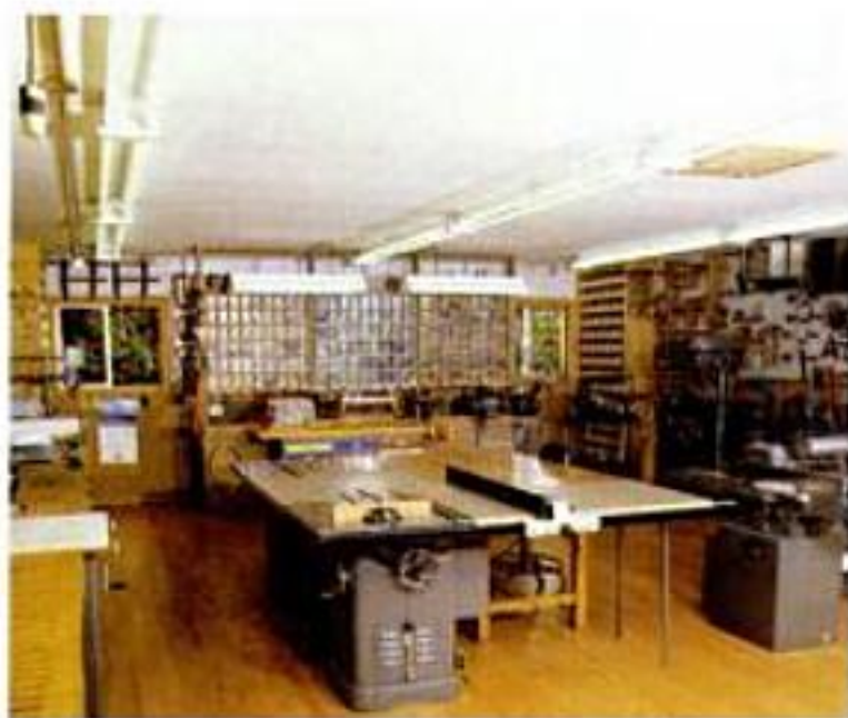
The right light. Ideal for overall illumination, fluorescent tubes (left) provide even light without consuming much electricity. Incandescent lights (right) remain the first choice for task lighting.
