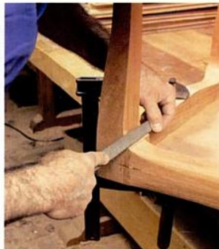
Blending the curves. After gluing up the table, fair the inside curves of the legs and rails with a patternmaker's rasp.
