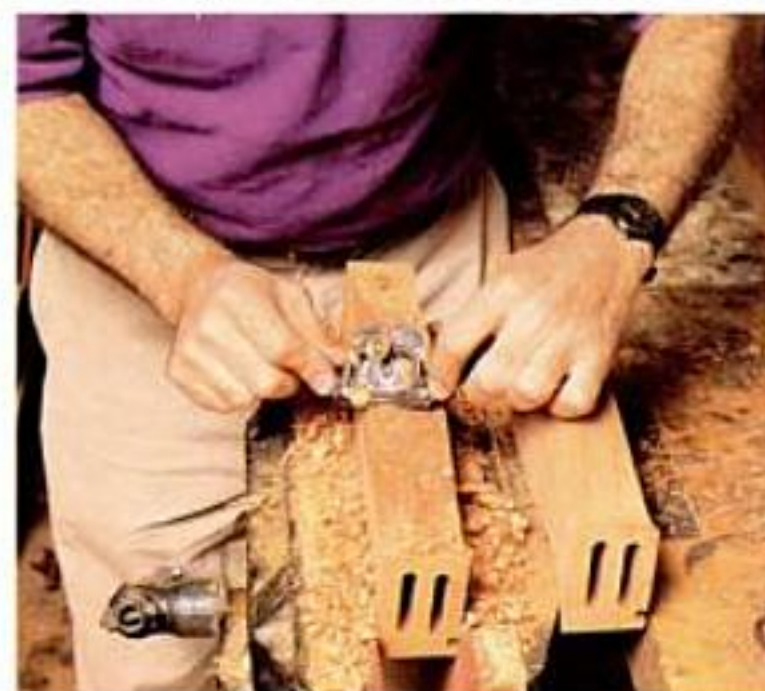
Carving the rails. Shape the face of each bandsawn rail (left) and round its lower edge (center) with a spokeshave. Complete the process with a random-orbit sander (right).
