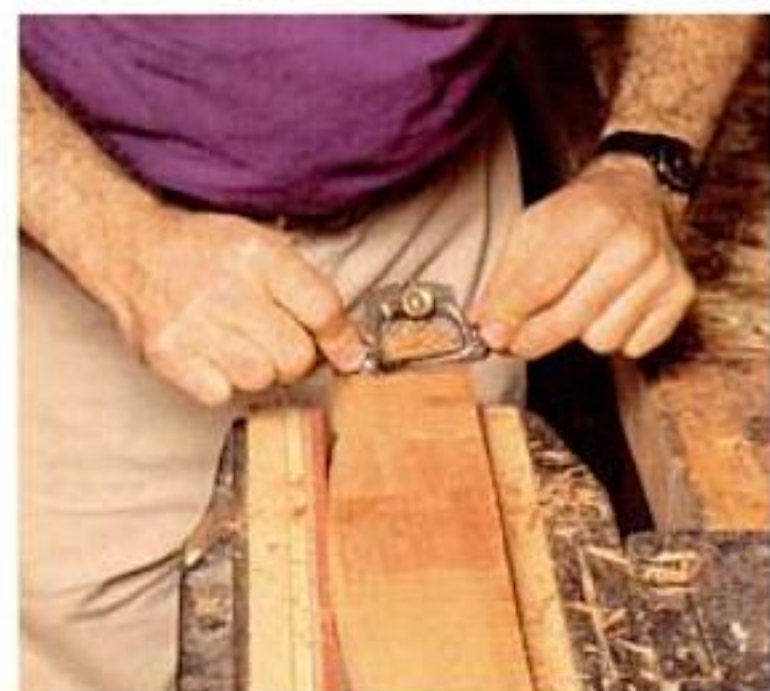
Carving the rails. Shape the face of each bandsawn rail (left) and round its lower edge (center) with a spokeshave. Complete the process with a random-orbit sander (right).
