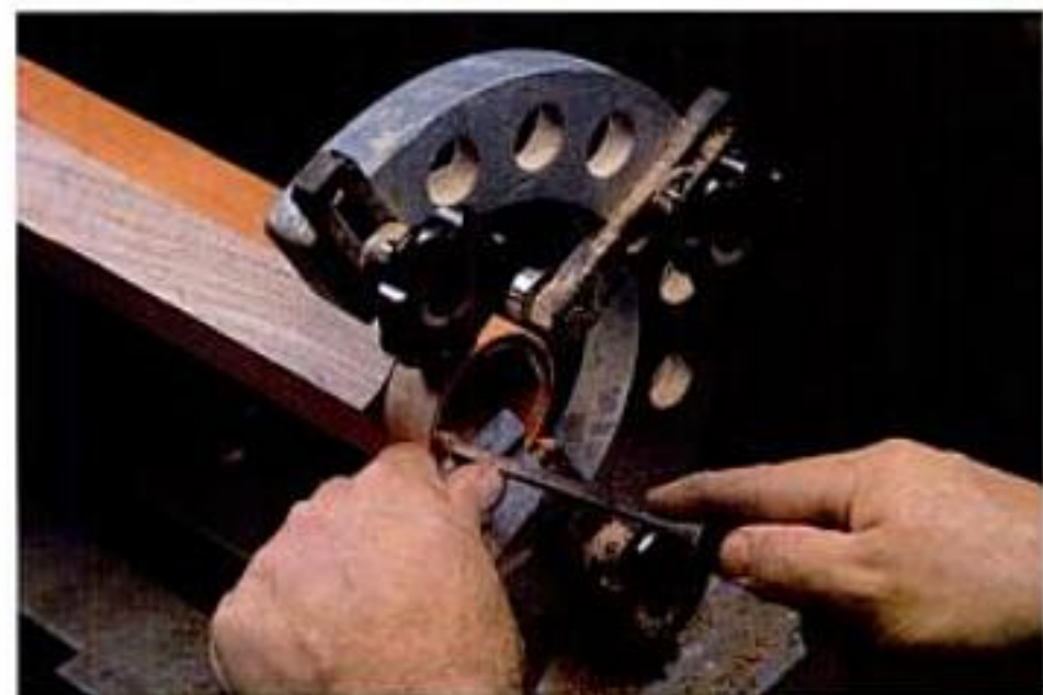
Rabbeting for the blocker. Using a commercial steadyrest, author rabbets the barrel for the glass "blocker" that keeps dust from contaminating the mirrored interior of the finished scope.
