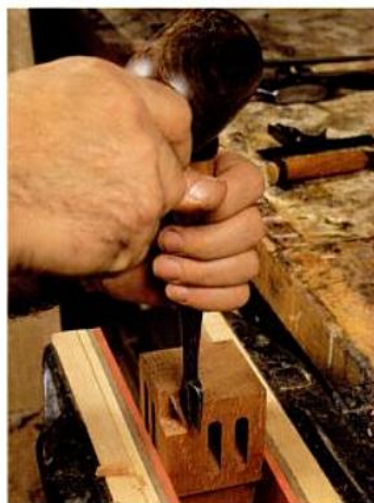
Notching the leg. Saw inside your layout marks first (above), then chisel away the waste (below).
