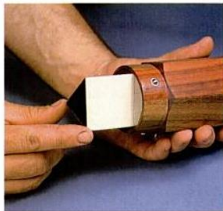
Installing the prism. Carefully insert the prism into the barrel, adding wraps of tape if necessary to achieve a snug fit.
