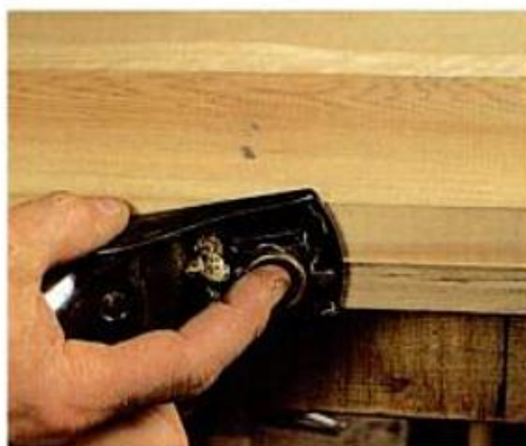
Jointing the veneers. Plane the edges of the face veneers with a block plane. Veneers are clamped between two straight-edged boards.
