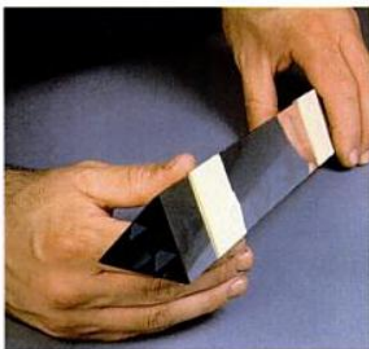
Completing the prism. When correctly assembled, mirror edges overlap, assuring tight seams.
