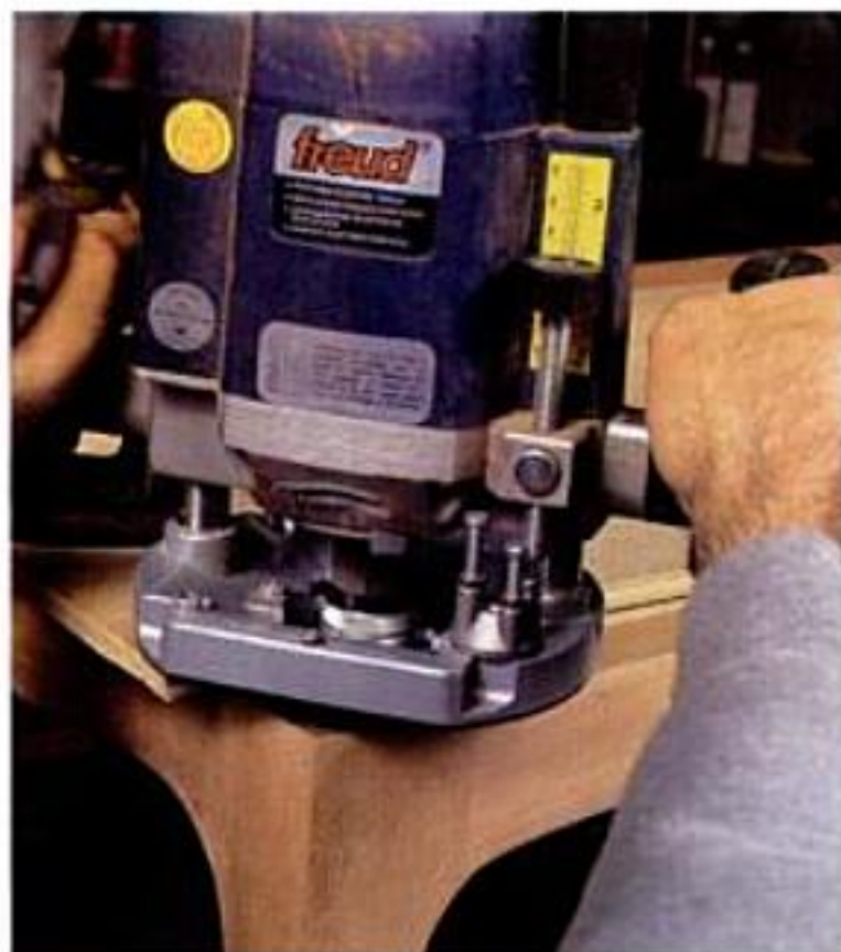
Grooving for inlay. Rout the inlay grooves with a plunge router and a straight bit, using a piece of 1/2-in. plywood as a template guide (left). Then chisel the corners to complete the groove (center).
