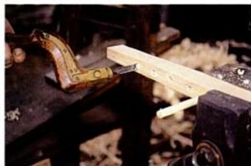
Aligning the tines. Drill one hole near the middle of the rake head and insert a tine to serve as a guide for boring all tine holes.
