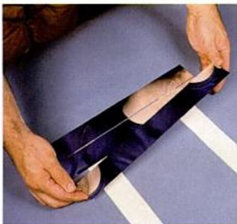
Making the mirror prism. For easy assembly, lay the mirror strips "coated side up" on two pieces of masking or duct tape.
