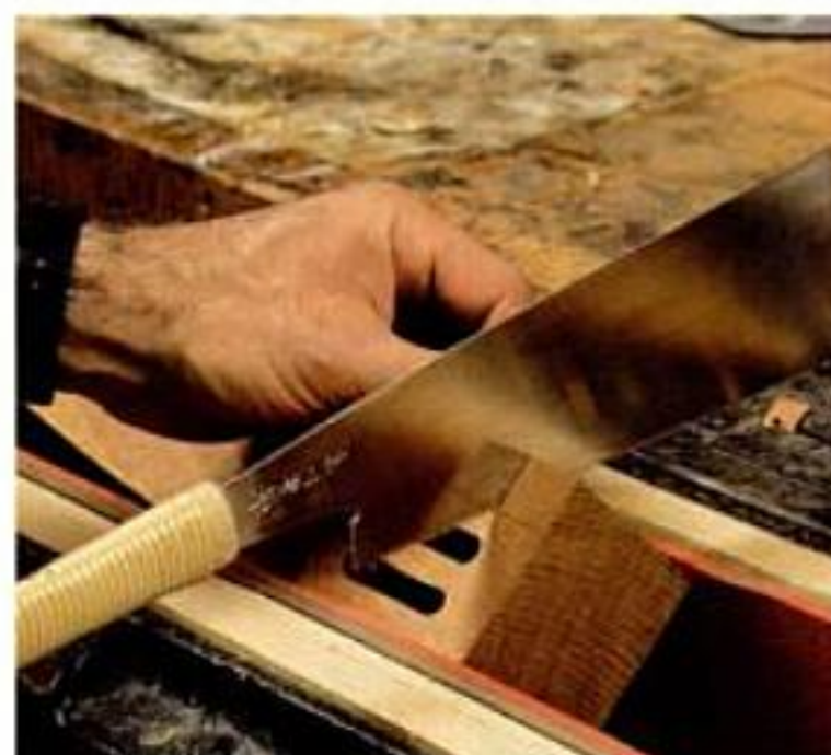
Notching the leg. Saw inside your layout marks first (above), then chisel away the waste (below).
