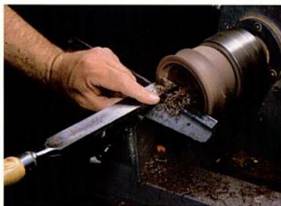
Turning the steps. A square-nosed tool is used to rabbet steps for the objective glass.
