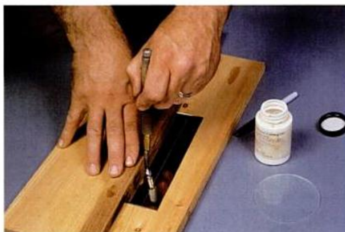
Straight cutting. Score the unsurfaced side of the mirror with a straight cutter dipped in light oil. A wooden straight-edge guides the cut.
