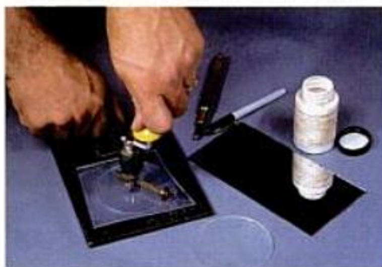
Circle cutting. This "lens cutter" lets you cut a disc without a center pivot point touching the glass.
