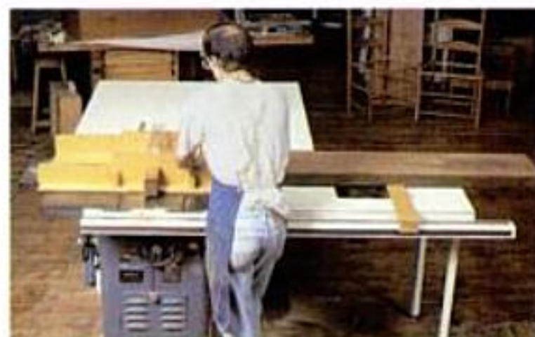
Big capacity. You can crosscut heavy boards with a side extension table, using a bench hook under the stock. The hook's thickness should match that of the cut-off box's base.
