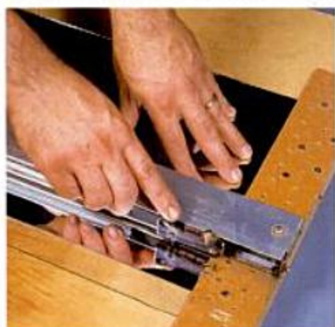
Rail-mounted cutting. This commercial rail-mounted cutter provides the utmost in accuracy and speed for production cutting.
