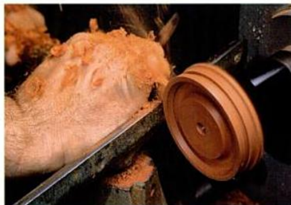
Parting off the retaining ring. Part off the retaining ring after turning the outside and inside surfaces. A screw chuck holds the blank for turning.
