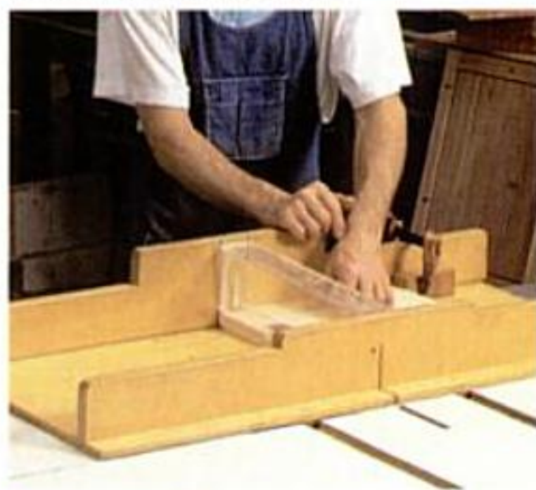
Speedy repetition. First make a square cut from one side of the blade, then butt the cut end against a stop block and crosscut to length.
