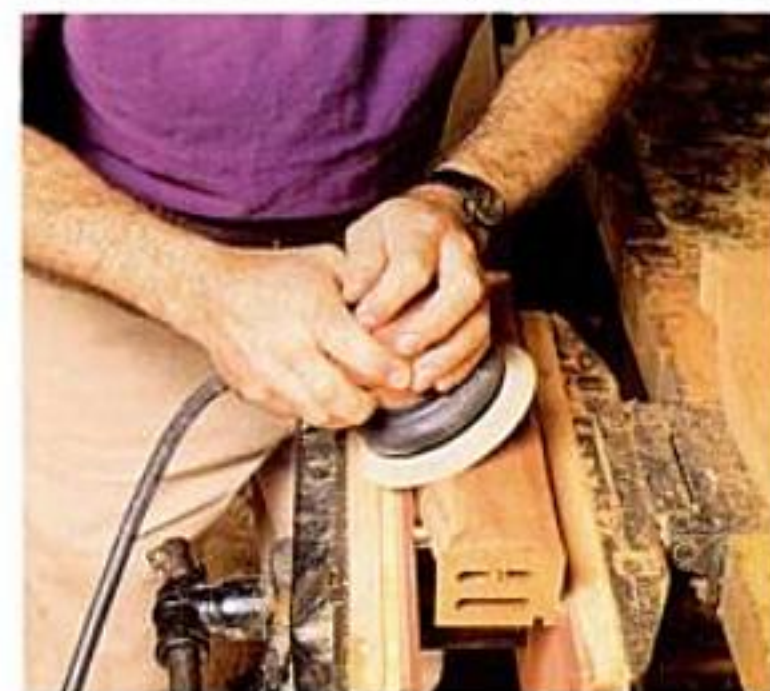
Carving the rails. Shape the face of each bandsawn rail (left) and round its lower edge (center) with a spokeshave. Complete the process with a random-orbit sander (right).
