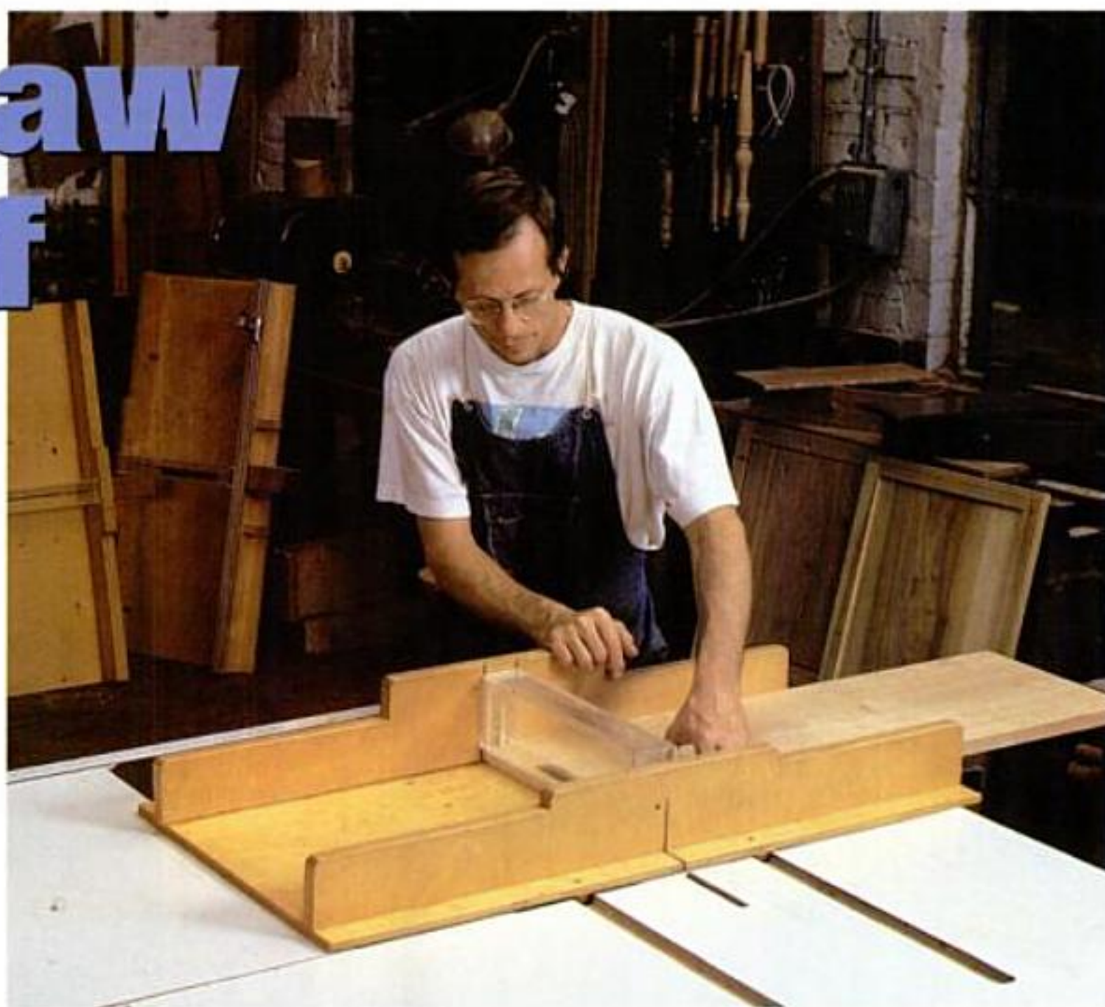
Crosscutting control. Mehler's cut-off box produces a dead-accurate 90° cut in small or large workpieces.
