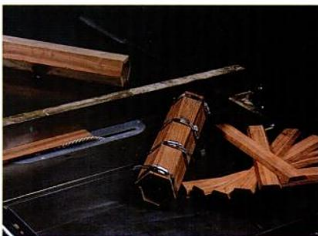
Making the coopered barrel. The author likes to use contrasting staves for his kaleidoscope barrels. After ripping the contrasting strips, glue them up and clamp with hose clamps.
