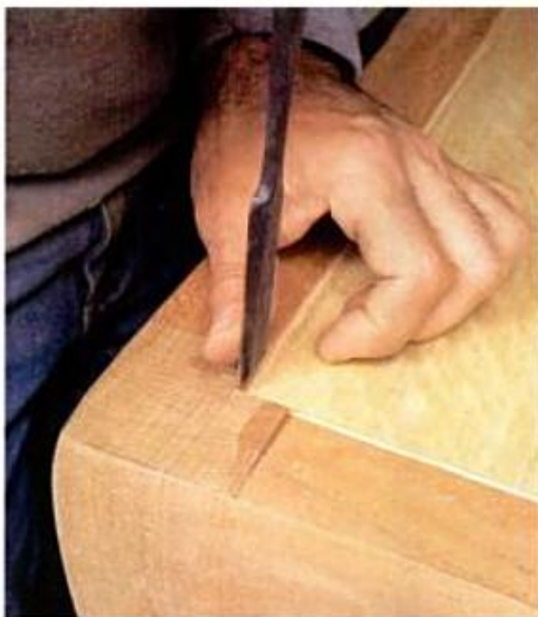
Grooving for inlay. Rout the inlay grooves with a plunge router and a straight bit, using a piece of 1/2-in. plywood as a template guide (left). Then chisel the corners to complete the groove (center).
