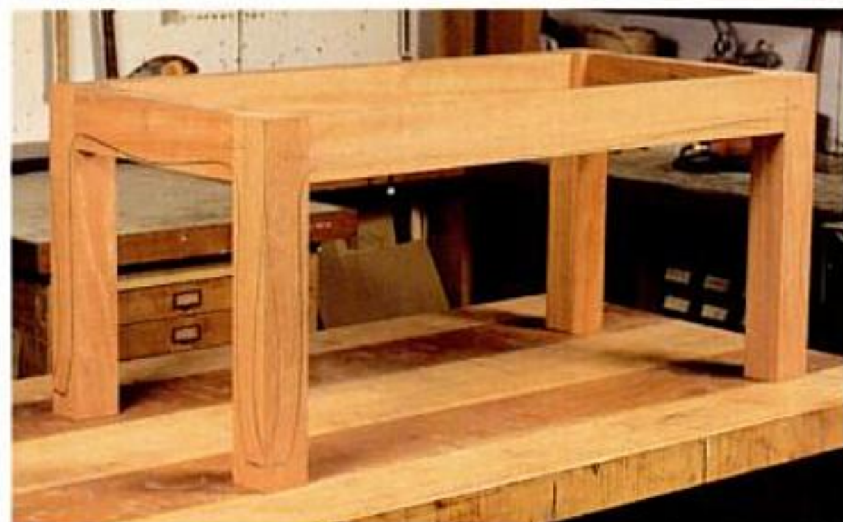
Checking the curves. After you've completed the joinery, preview the curves by tracing the curved templates on the dry-assembled table.
