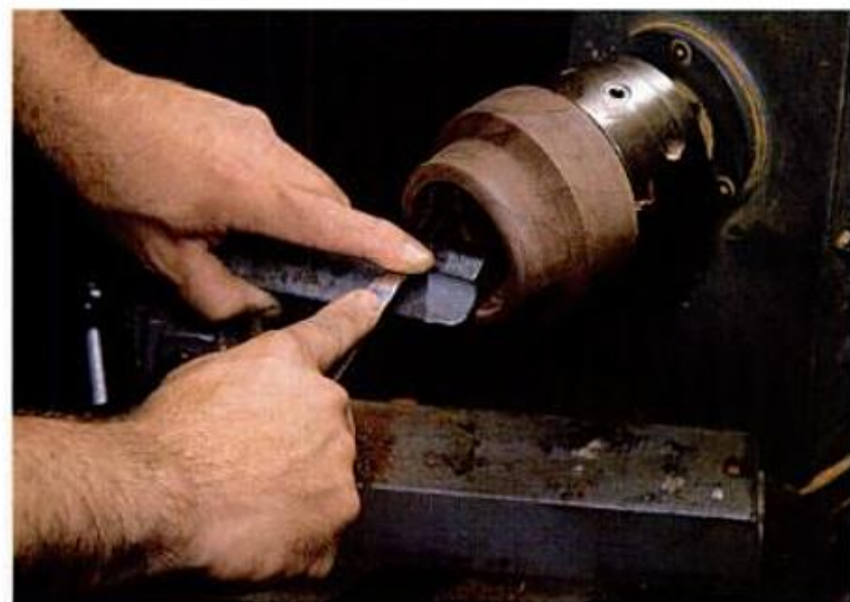
Turning the bullet groove. With the objective held in a three-jaw chuck, the author turns a round-bottomed groove to mate with bullet catches in the barrel.
