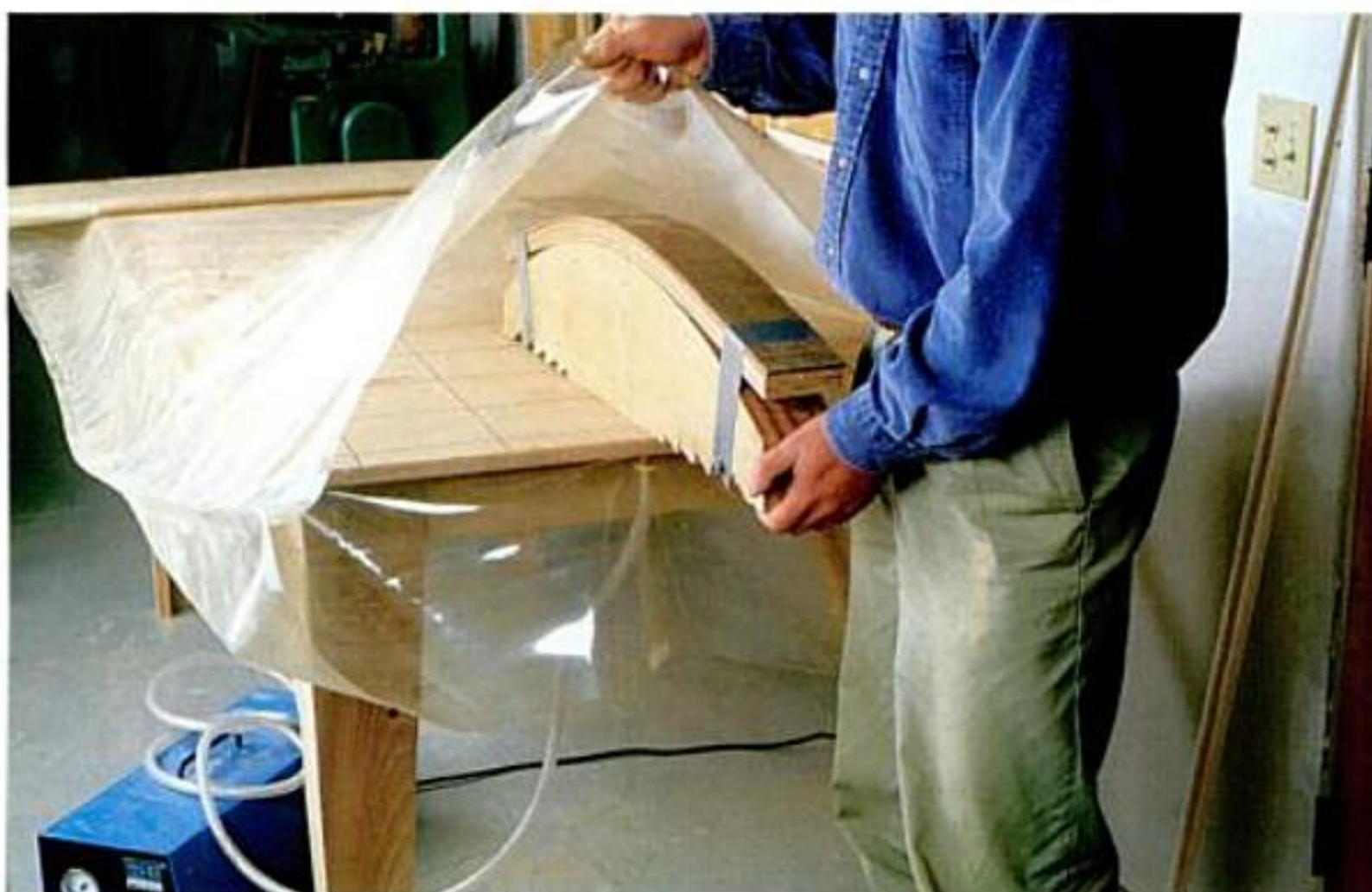
Author uses a vacuum press to clamp laminates onto a one-part form. The work is placed inside the bag (left) and the vacuum pump on the floor sucks the air from the bag. Atmospheric pressure holds the laminates (above) tightly to the form.
