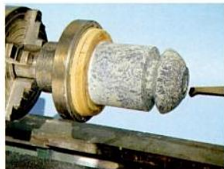
Author screws faceplate to a 2-in. piece of steel and then mounts this in a four-jaw chuck whose jaws move independently. This allows him to precisely center a blank after it is mounted.
