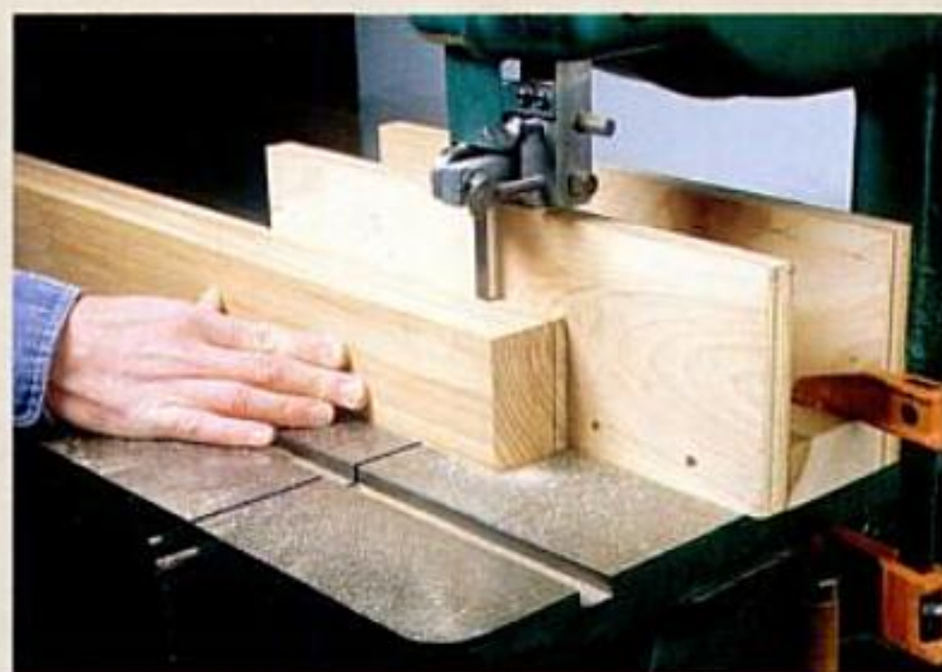
Resawing is more accurate when you use a sharp blade and a simple shop-made fence.
