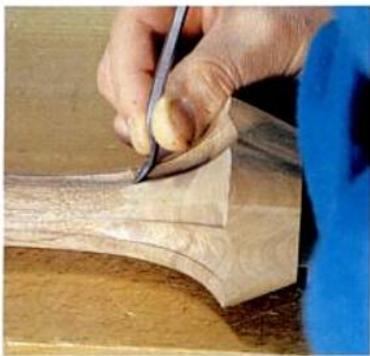
STEP 4: Carve the hollows and rounds with a 1/2-in.-wide, #7 spoon-bent gouge, and switch to a 1/4-in.-wide, #7 spoon-bent gouge as the hollows narrow at the ankle.
