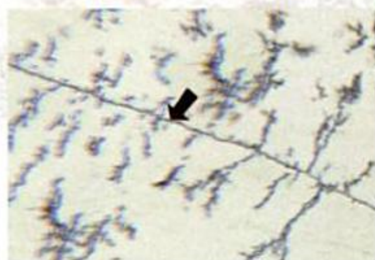
When a turning blank has a black line fracture like this one, it is sure to break. Author splits blanks like these into smaller chunks to turn miniature pots.
