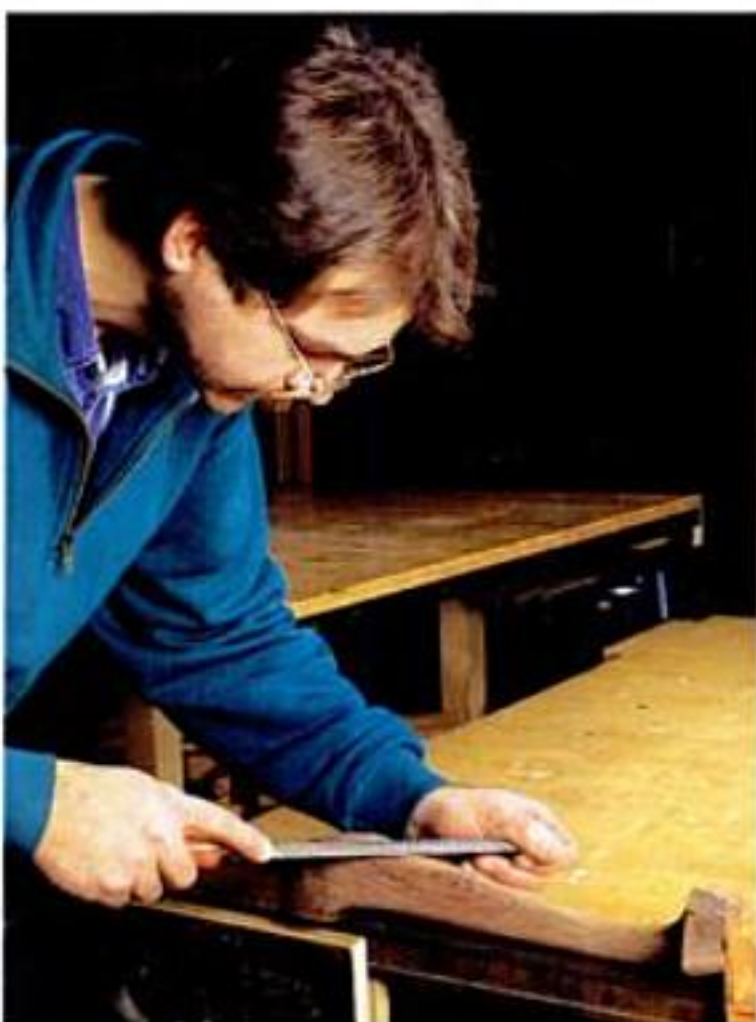
Author holds leg in a pipe clamp held in a vise so he can shape it with a rasp prior to filing and sanding.
