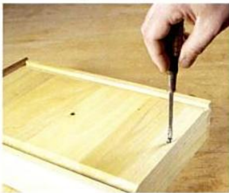
Author attaches drawer bottom to back with a screw. Slotted hole permits bottom to move.
