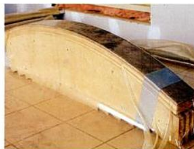
Author uses a vacuum press to clamp laminates onto a one-part form. The work is placed inside the bag (left) and the vacuum pump on the floor sucks the air from the bag. Atmospheric pressure holds the laminates (above) tightly to the form.
