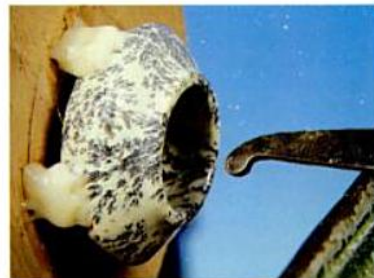
After the outside is turned, the bowl is reversed and then glued to a recess cut in a wooden faceplate. To get a good bond, author builds up layers of hot-melt glue.
