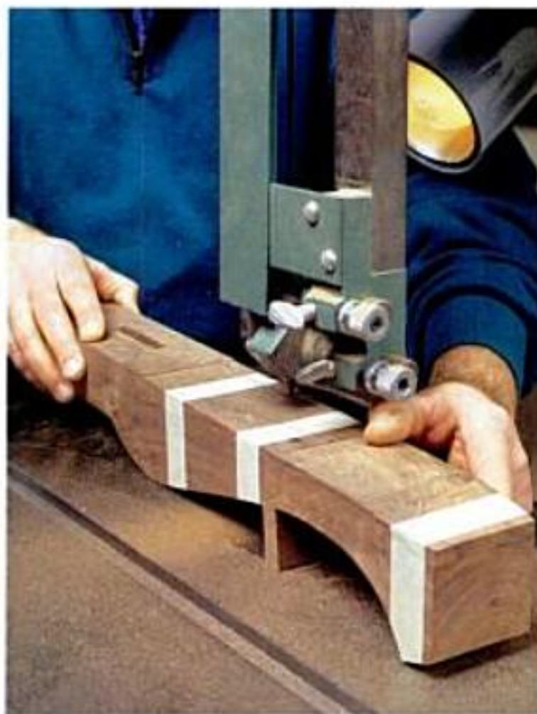
To cut compound curve on a cabriole leg, author saws one face, then tapes on the offcuts and cuts adjacent face.
