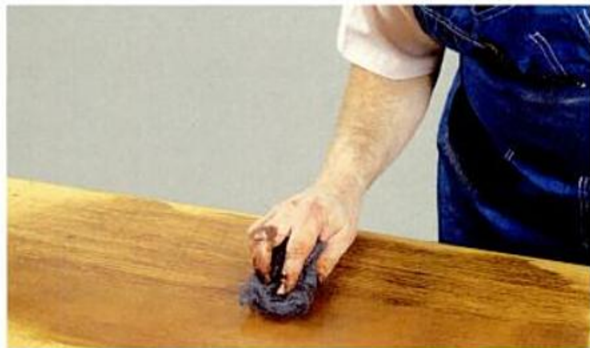
Author adds a wood-grain effect by lightly wiping fine steel wool through a thin coat of wet glaze.
