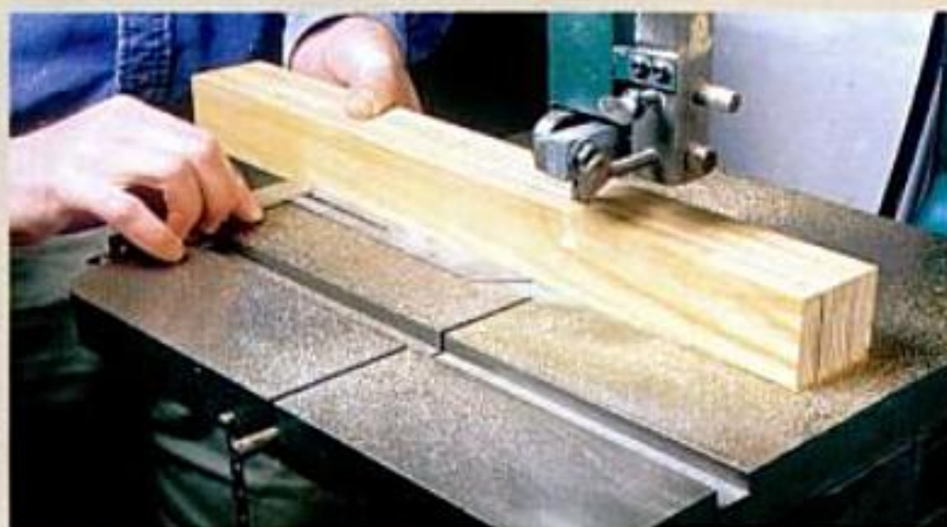
Author saws along a straight line to determine the "drift" of the blade, and then records the angle with a bevel gauge.
