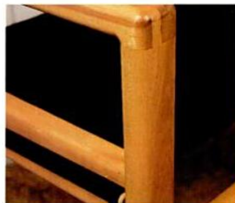
The ends of the seat fit through slots in the side rails. A dowel slips into a pocket at each end to hold the seat in place.
