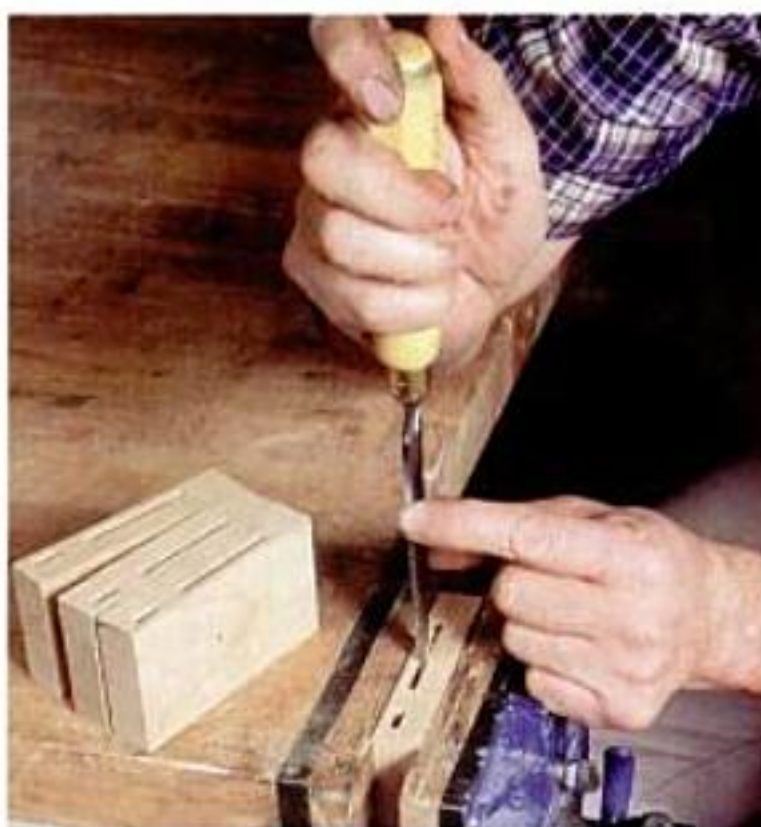
To support thin mortise walls when paring with a chisel, clamp the corner blocks in a vise.
