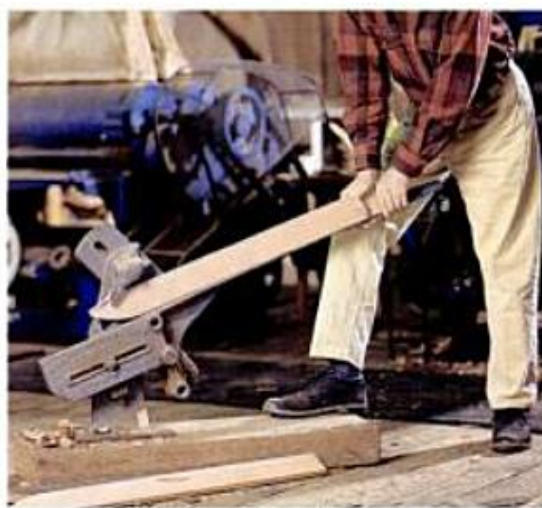
Simple but effective, this hand-operated machine uses leverage and a sharp blade to slice points on the ends of slats for picket fences.
