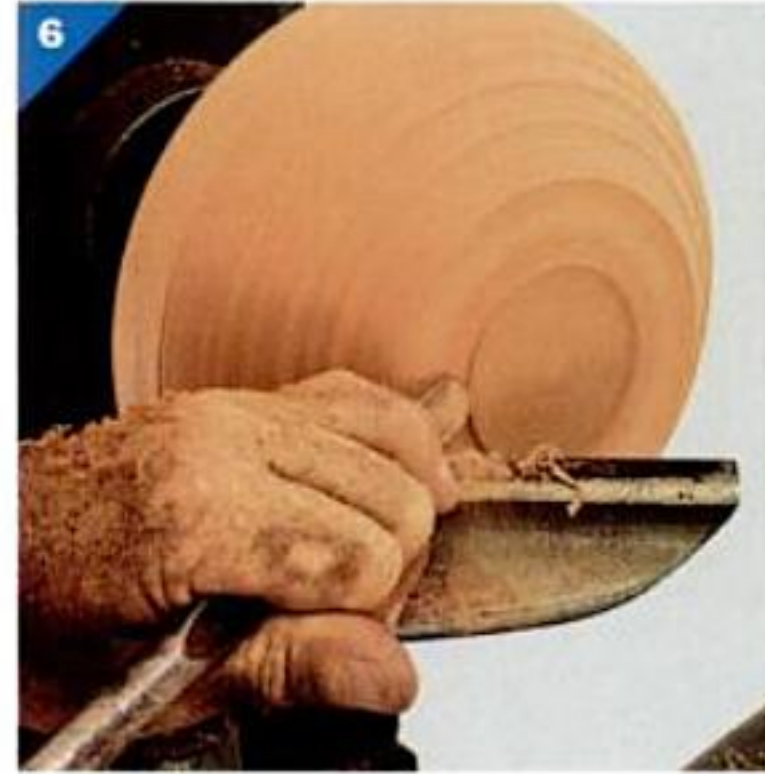
To true the base, squeeze your hand (left), pulling the tool into the uneven surface to flatten it, then turn the tool around and shear cut toward center (right).
