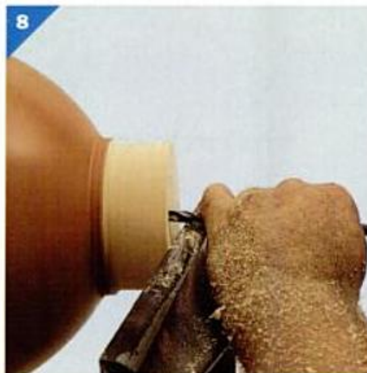
To establish hole depth, author bores with a hand-held twist drill. Scribed marks on the drill help him determine the exact depth of the hole.
