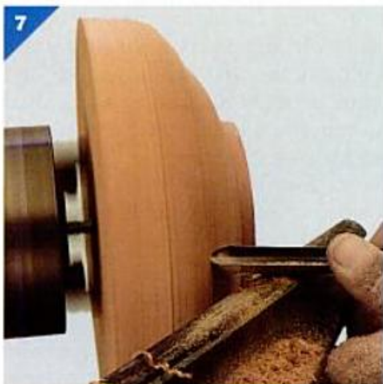
To finish the profile of the bowl, use the shallow gouge, held nearly horizontal, and lightly shear cut from the bottom to the top of the bowl.
