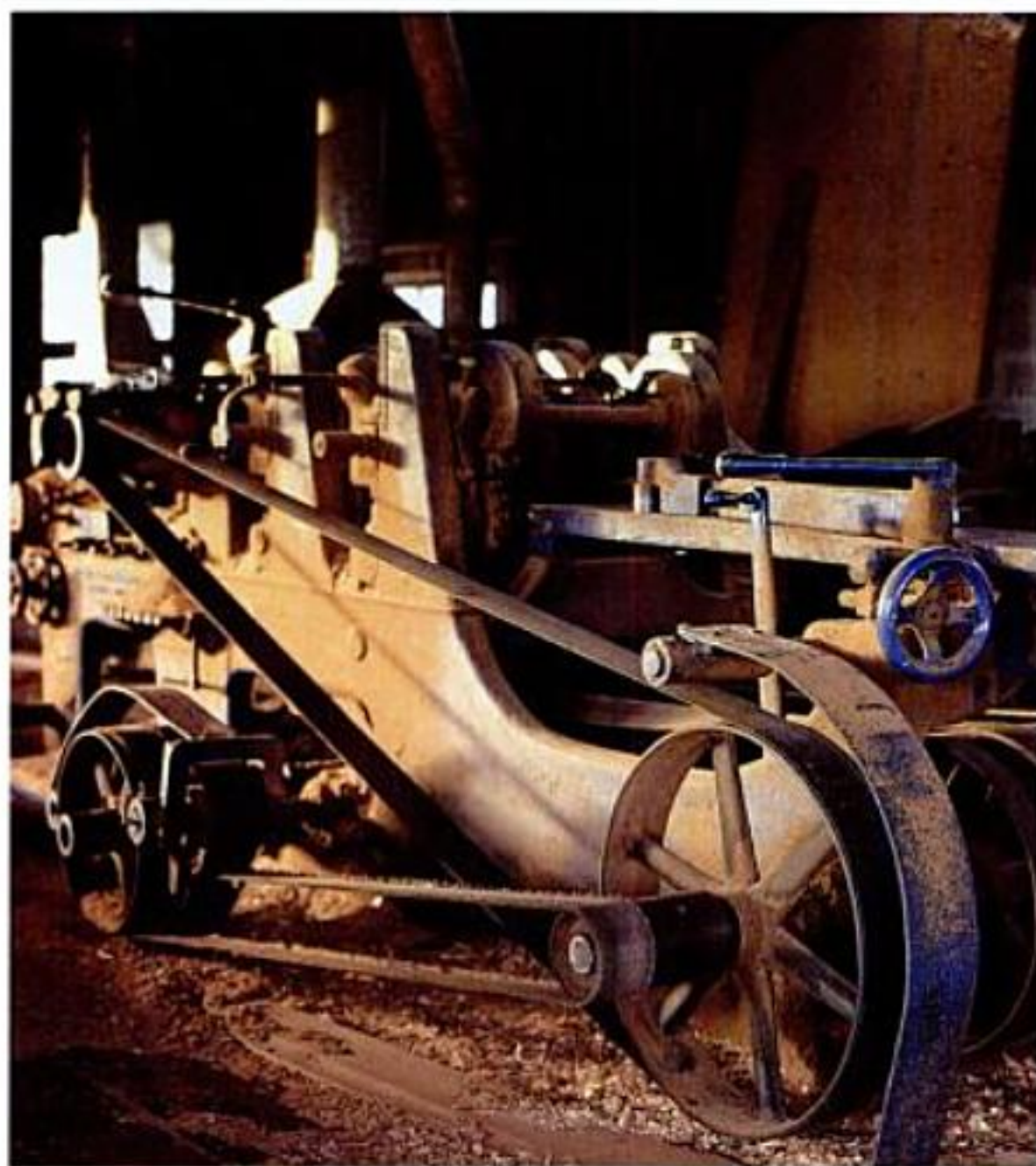
This massive Hermance molder, vintage 1912, will shape profiles on four sides of a piece of wood at once.
