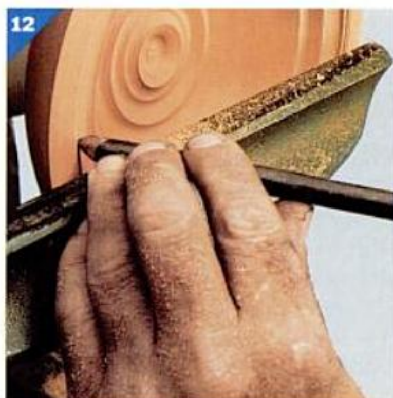
To prevent kickback when starting a cut from space, bring the tool down through an arc into the wood by lifting the handle and pivoting the tool on the rest.
