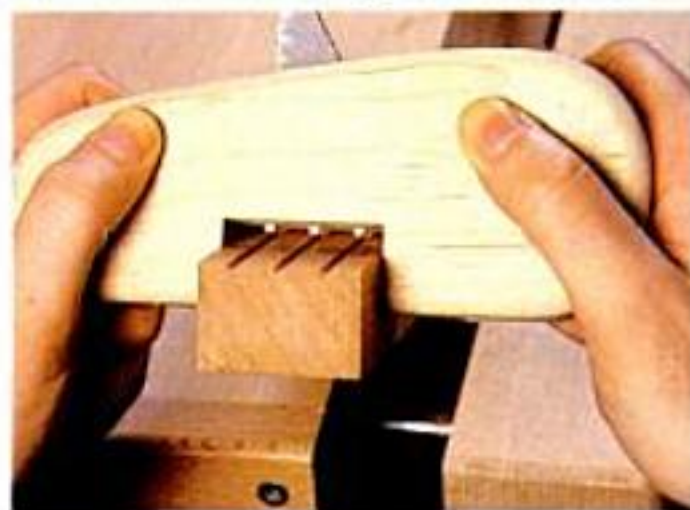
This scratch stock (left) registers on both sides of the work to cut three inlay grooves very accurately (right).
