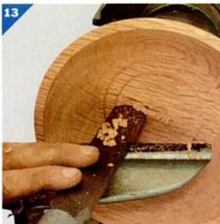
13 Finish the interior with a large scraper, swinging the tool in broad movements.
