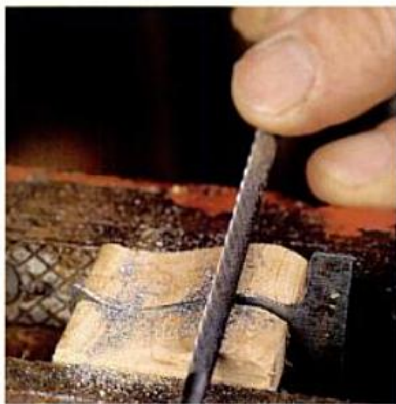
Bandsawn blocks help keep the file square to the blade when shaping the final profile.
