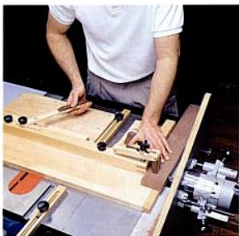
The jig's hold-down clamp pivots so you can clamp stock against either face of the sliding fence.
