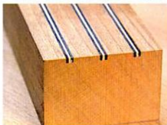
This scratch stock (left) registers on both sides of the work to cut three inlay grooves very accurately (right).
