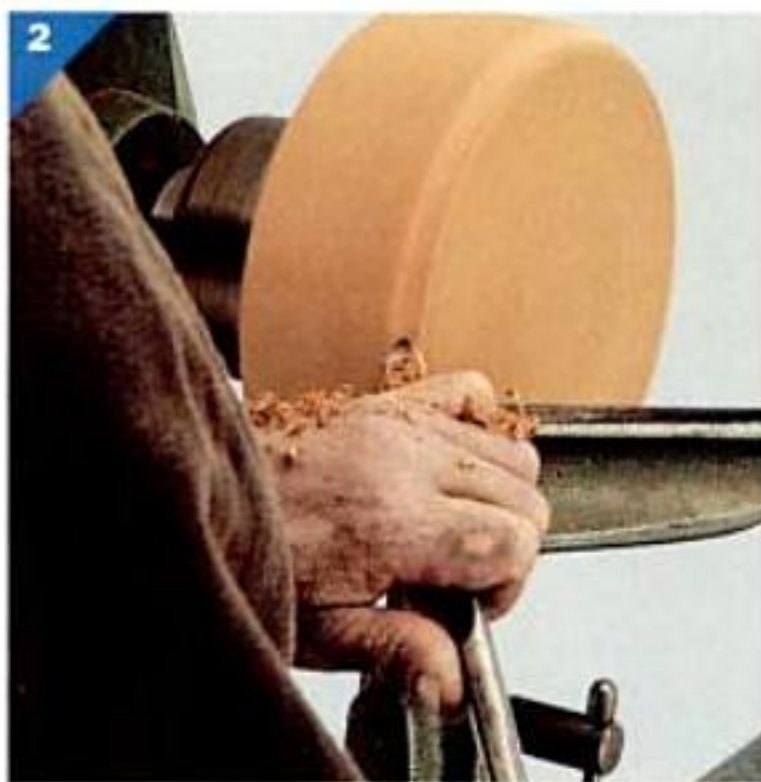
To rough out the profile, hold the shallow-fluted gouge about 30° up from horizontal. Then raise the handle to pivot the cutting edge into the work and sweep the tool through an arc (left and center). The bevel doesn't contact the wood, as shown at far right.
