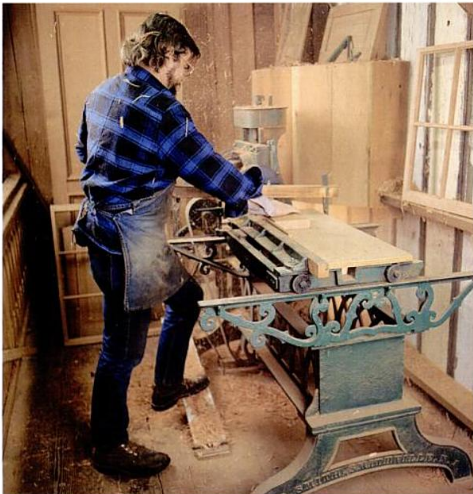
Hollenbeck cuts tenons on an antique tenoner that's covered with cast-iron filigree.
