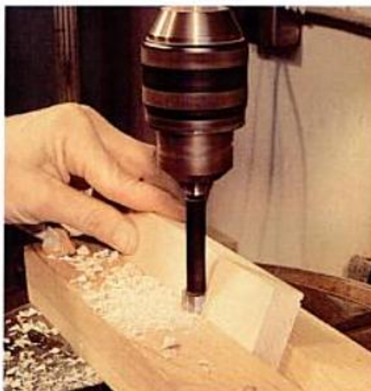
Drill pocket holes in the top rails with a \frac{1}{2} -in. Forstner bit, using a simple jig to hold the stock at 15° from vertical.
