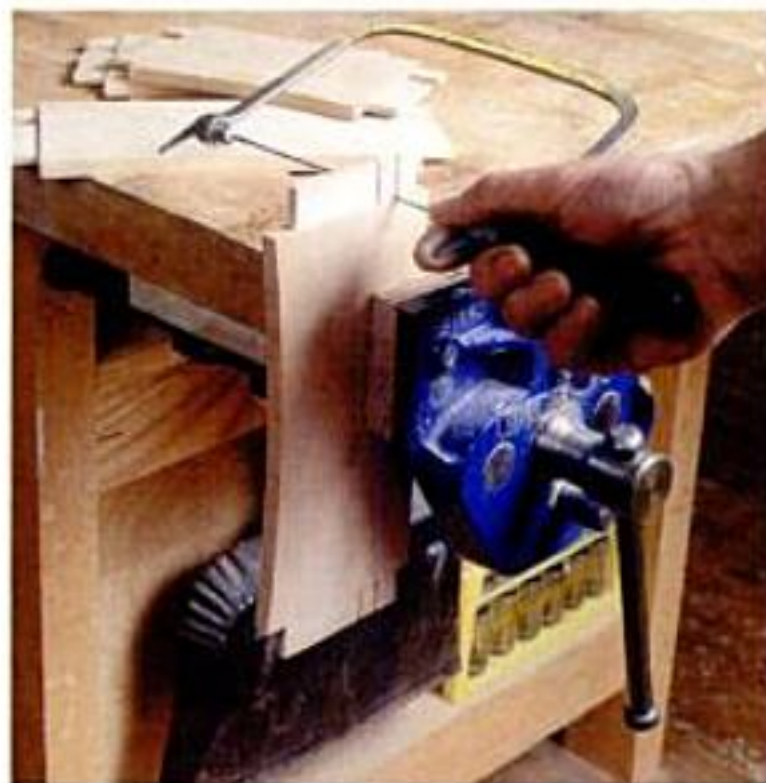
Make two tenons from one by removing material from the middle with a back-saw, coping saw and chisel.
