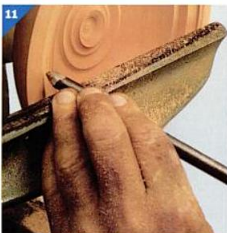
To prevent kickback when starting a cut from space, bring the tool down through an arc into the wood by lifting the handle and pivoting the tool on the rest.
