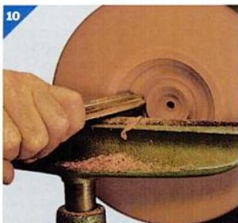
To hollow the interior, cut from the larger to smaller diameter, using a shear cut with the flutes facing toward center.
