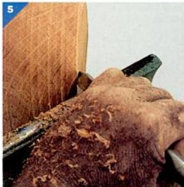
To true the base, squeeze your hand (left), pulling the tool into the uneven surface to flatten it, then turn the tool around and shear cut toward center (right).
