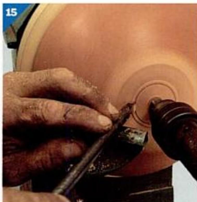
15 For added support while finishing the base, you can use the tailstock to press the bowl into the chuck (left), or apply pressure to the bowl with your upper hand (right). In either case, make light cuts; they'll be less likely to catch.
