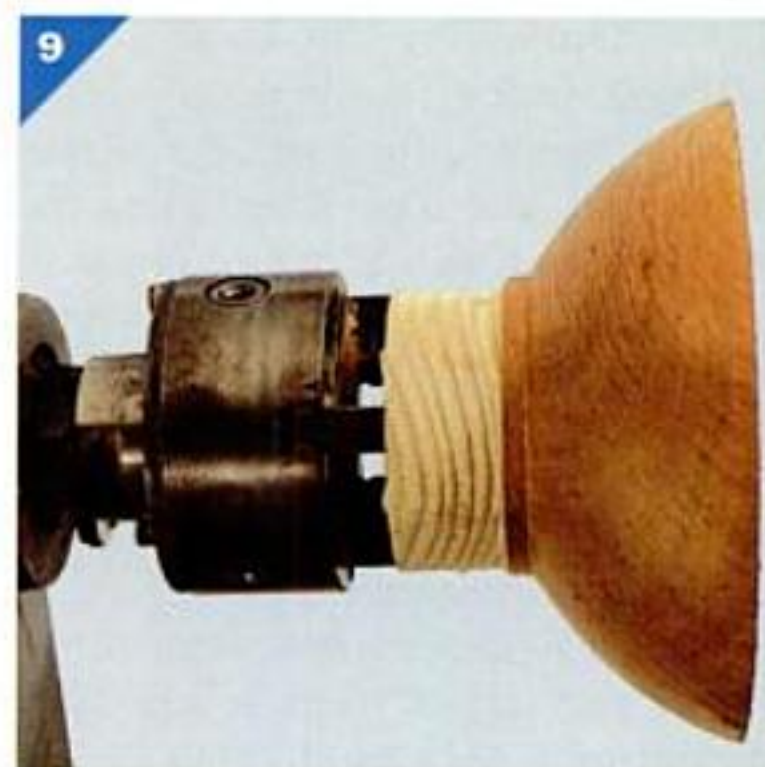
When reversing the bowl for hollowing on a screw chuck, glue the base of the bowl to a waste block, then screw the block to the chuck.
