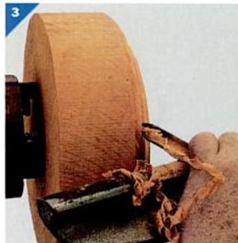
To rough out the profile, hold the shallow-fluted gouge about 30° up from horizontal. Then raise the handle to pivot the cutting edge into the work and sweep the tool through an arc (left and center). The bevel doesn't contact the wood, as shown at far right.
