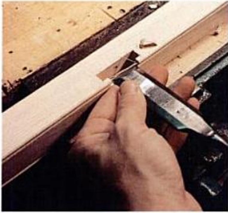
STEP 3: Remove waste between the saw cuts with a sharp chisel, being careful not to pare past the bottom of the bead.
