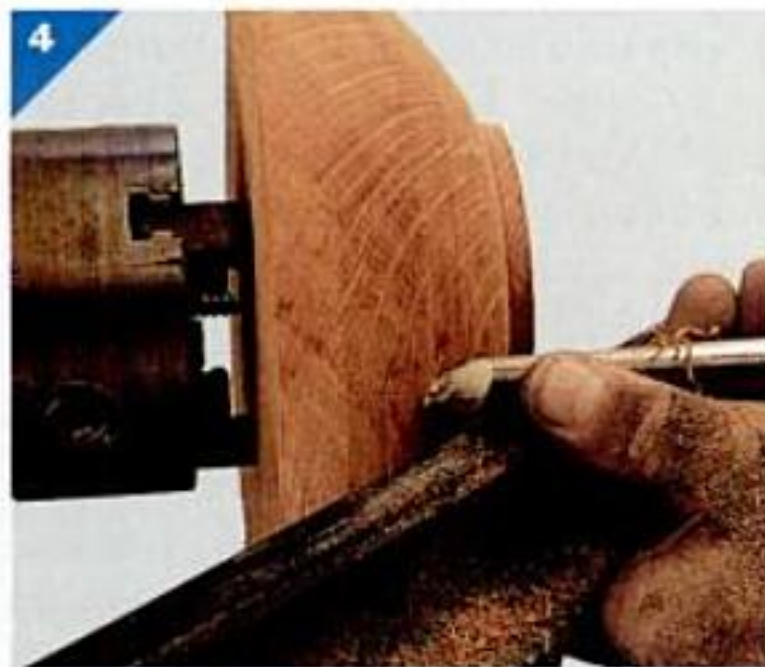
The cleanest roughing cut comes from a back cut, where you shear with the full round shoulder on the inside edge of the gouge.
