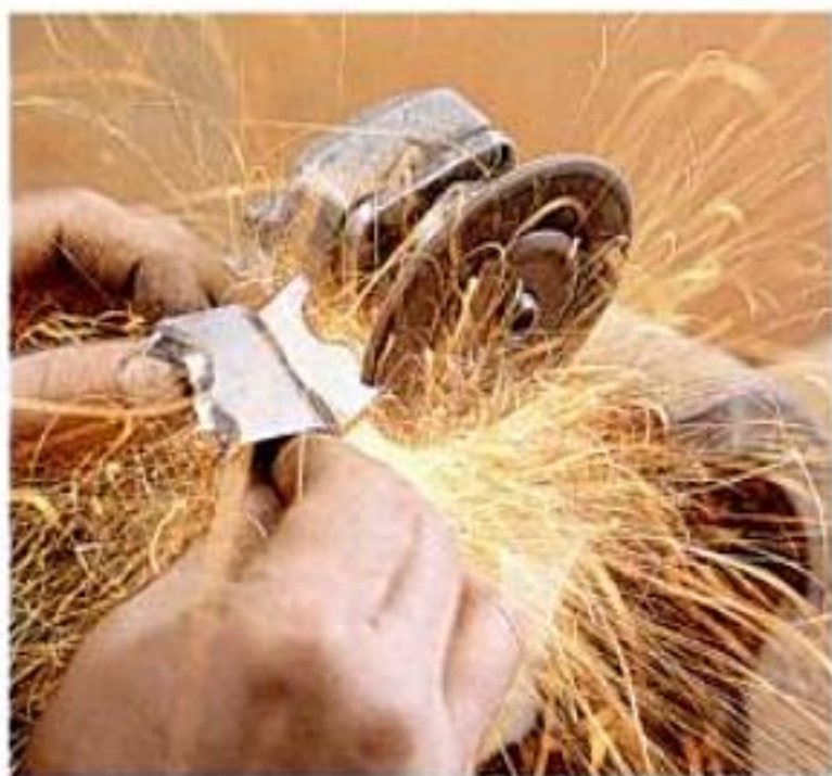
To match 19th-century moldings, Hollenbeck grinds his own cutters using a portable electric grinder clamped in a machinist's vise.
