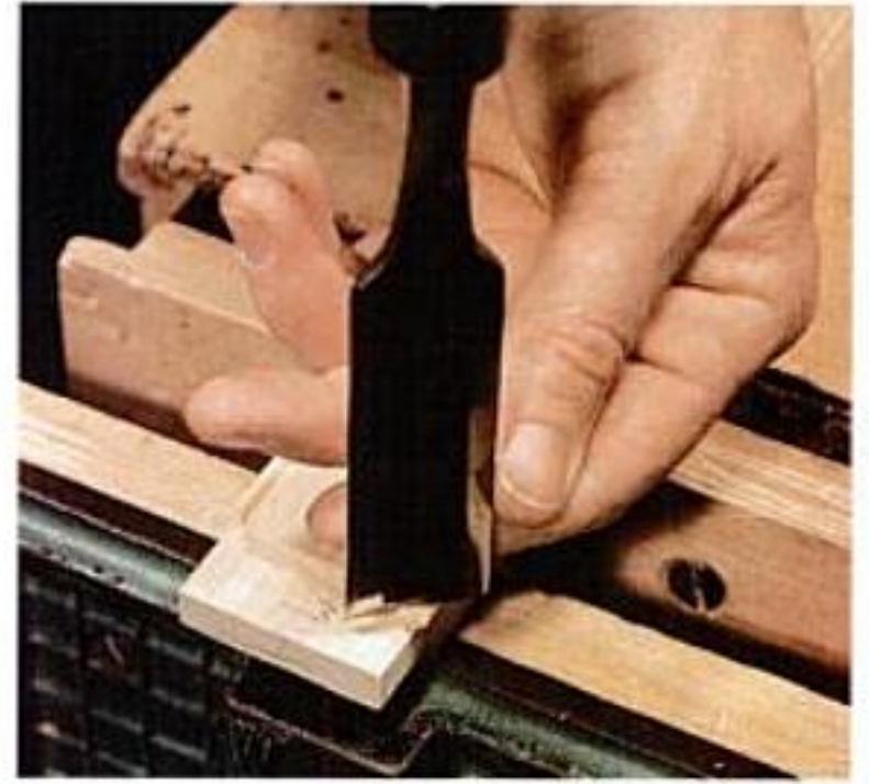
STEP 5: Cut the miters on the rails free-hand, fit the rails and make any necessary corrections.
