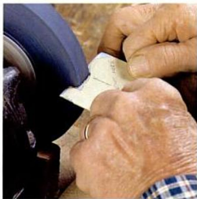
Author uses paper template as a guide while grinding the blade blank to create a rough profile.
