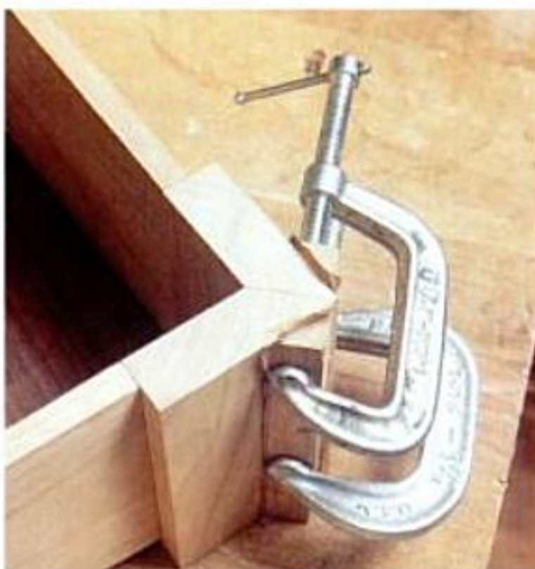
Clamp the miters using angled blocks to direct clamping pressure.
