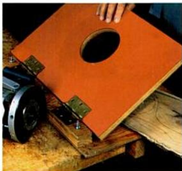
For production runs, author lays mirror blanks under the opening in a hinged circle template, then clamps the template to hold the board and routs the mirror recess.
