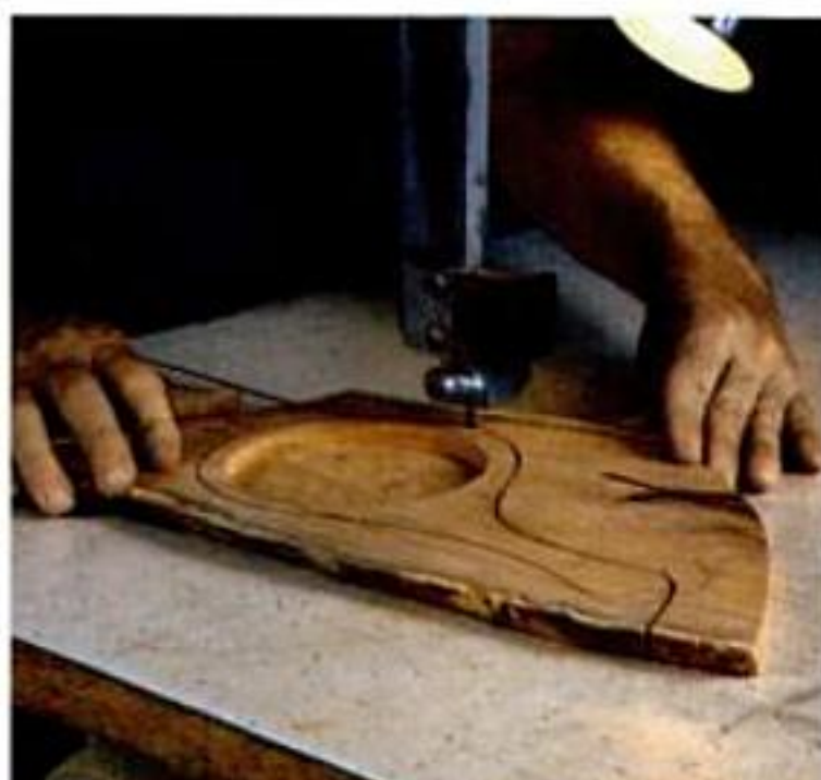
Cut out the mirror body on the bandsaw, then round over and smooth the edges.
