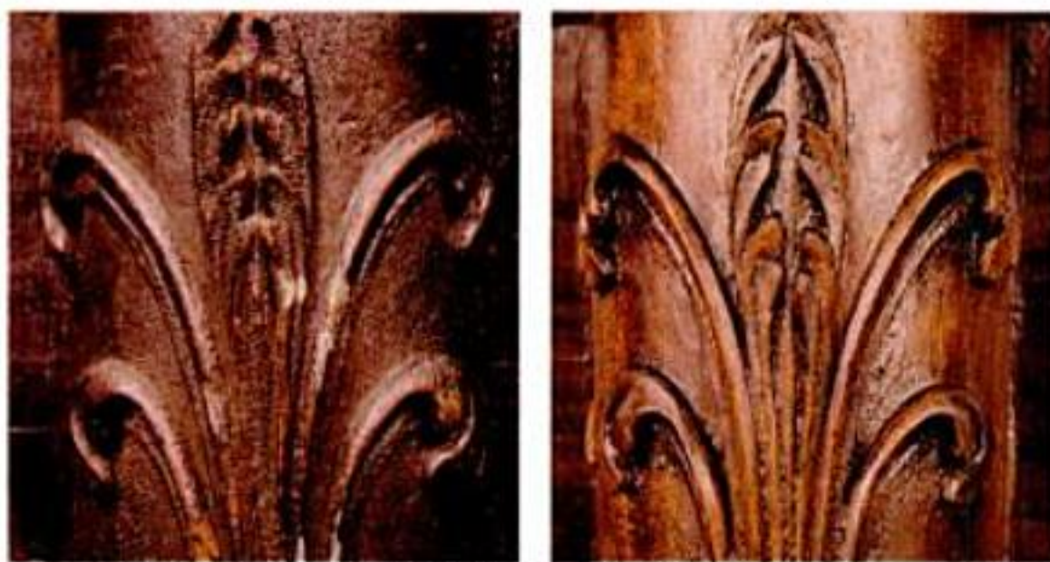
The old shellac on this table leg (left) was rejuvenated by wiping and brushing the surface with alcohol.
