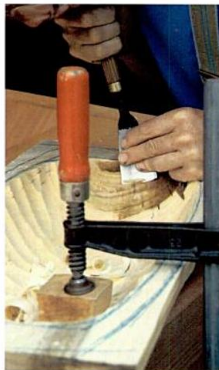
With the blank clamped to the workbench, author uses a bent gouge to refine the shape of the interior.
