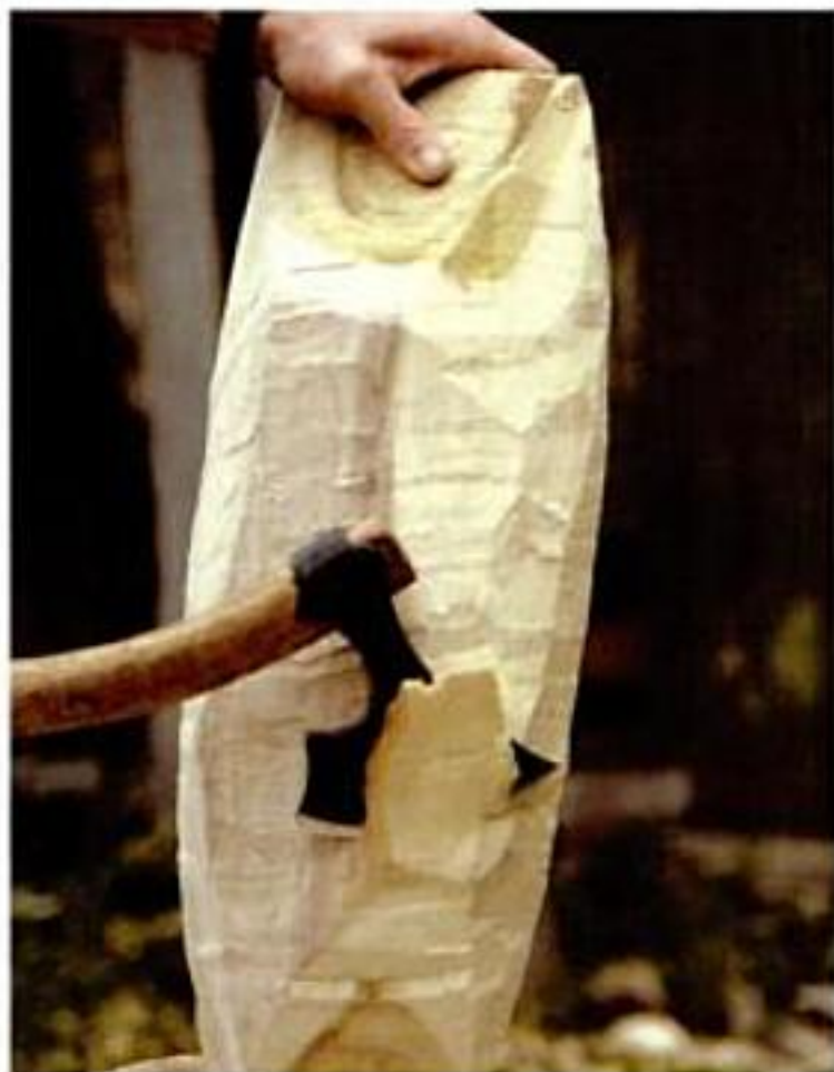
To rough-shape the exterior of the bowl, first use a hatchet to hew the ends (above), then round the sides (below).
