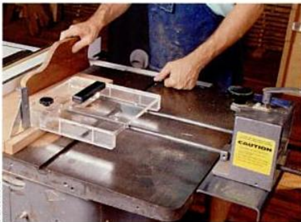
The Brett-Guard 10A-L's blade cover rides lightly on the workpiece to hold it down.
