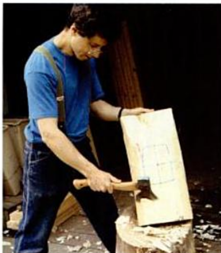
To rough-shape the exterior of the bowl, first use a hatchet to hew the ends (above), then round the sides (below).
