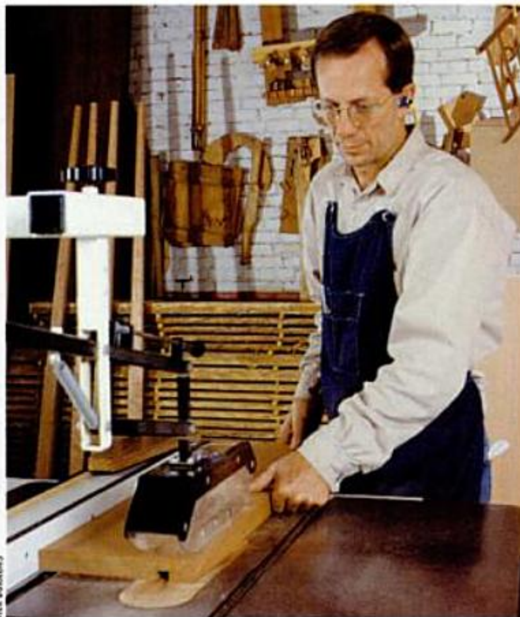
Aftermarket tablesaw guards protect your hands during many types of cuts where a standard guard gets in the way.
