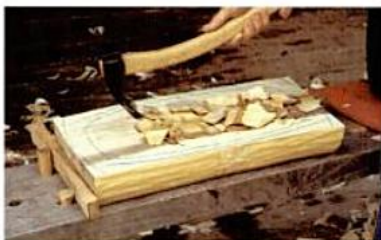
Working on a low bench, author uses a Swedish hollowing adze to begin hollowing the bowl.
