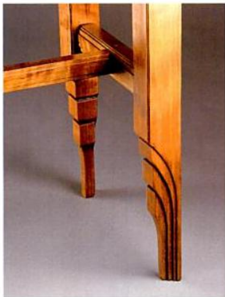
Author created foot details and fillets on legs, stretchers and breadboard ends with a 10-in. saw blade.
