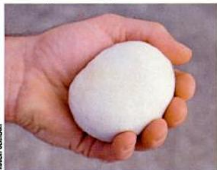
Author makes a finishing pad by wrapping layers of lint-free cloth around a handful of cotton.
