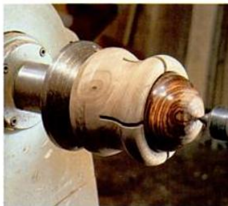
Use the tailstock to seat the shaker in the compression chuck, taking care not to push too hard on the shaker's delicate walls.
