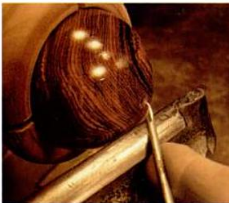
A curved-tip scraper made from a cement nail flares the edges of the shaker's holes.
