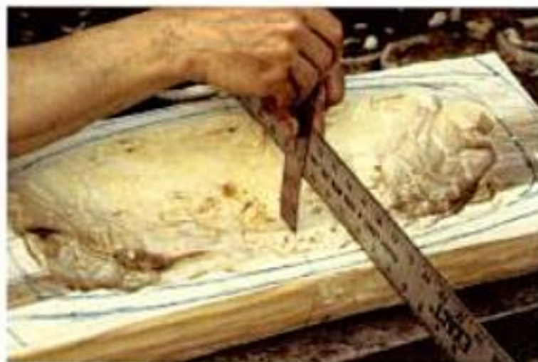
To determine the thickness of the bowl bottom, measure against a ruler set across the rim. The difference between the inside and outside measurements represents the thickness.
