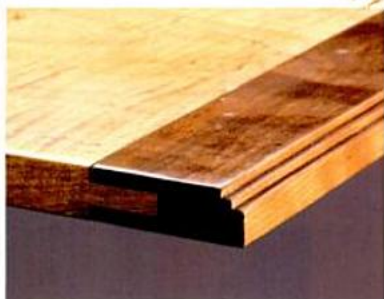
Author created foot details and fillets on legs, stretchers and breadboard ends with a 10-in. saw blade.
