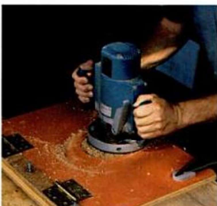
For production runs, author lays mirror blanks under the opening in a hinged circle template, then clamps the template to hold the board and routs the mirror recess.
