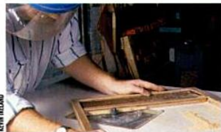
Author routs the rabbet for the mirror by running the glued-up frame over a piloted bit in his router table.
