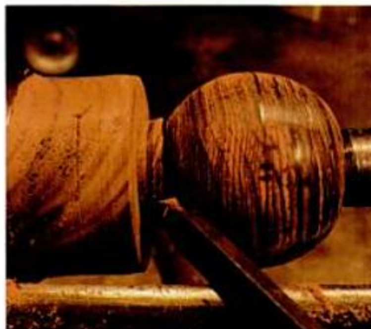
To work the tight space at the base of the sphere, author makes shear scraping cuts with the side of a specially ground parting tool.
