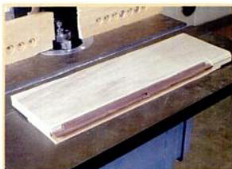
This simple plywood jig holds muntins safely for sticking and rabbeting.
