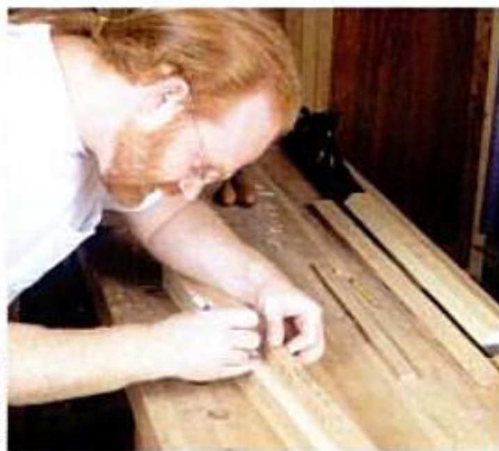
Using a story pole to lay out dimensions on posts such as legs and rails keeps measurements uniform from piece to piece.
