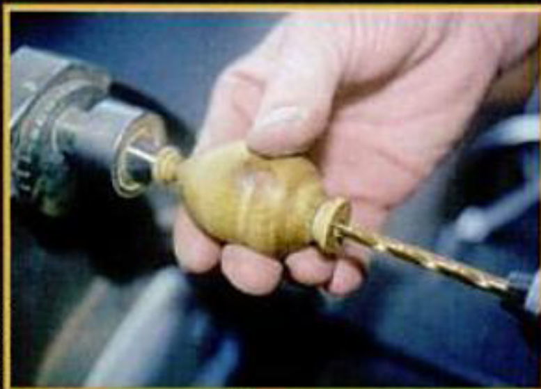
With one end of the top pressed against the tailstock for support, drill the stem hole. Use the center marks left by the drive center to align the bit.
