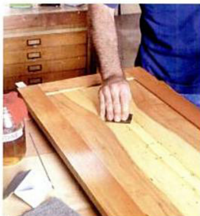
Author wet-sands the second coat to help fill the pores while removing any surface roughness.
