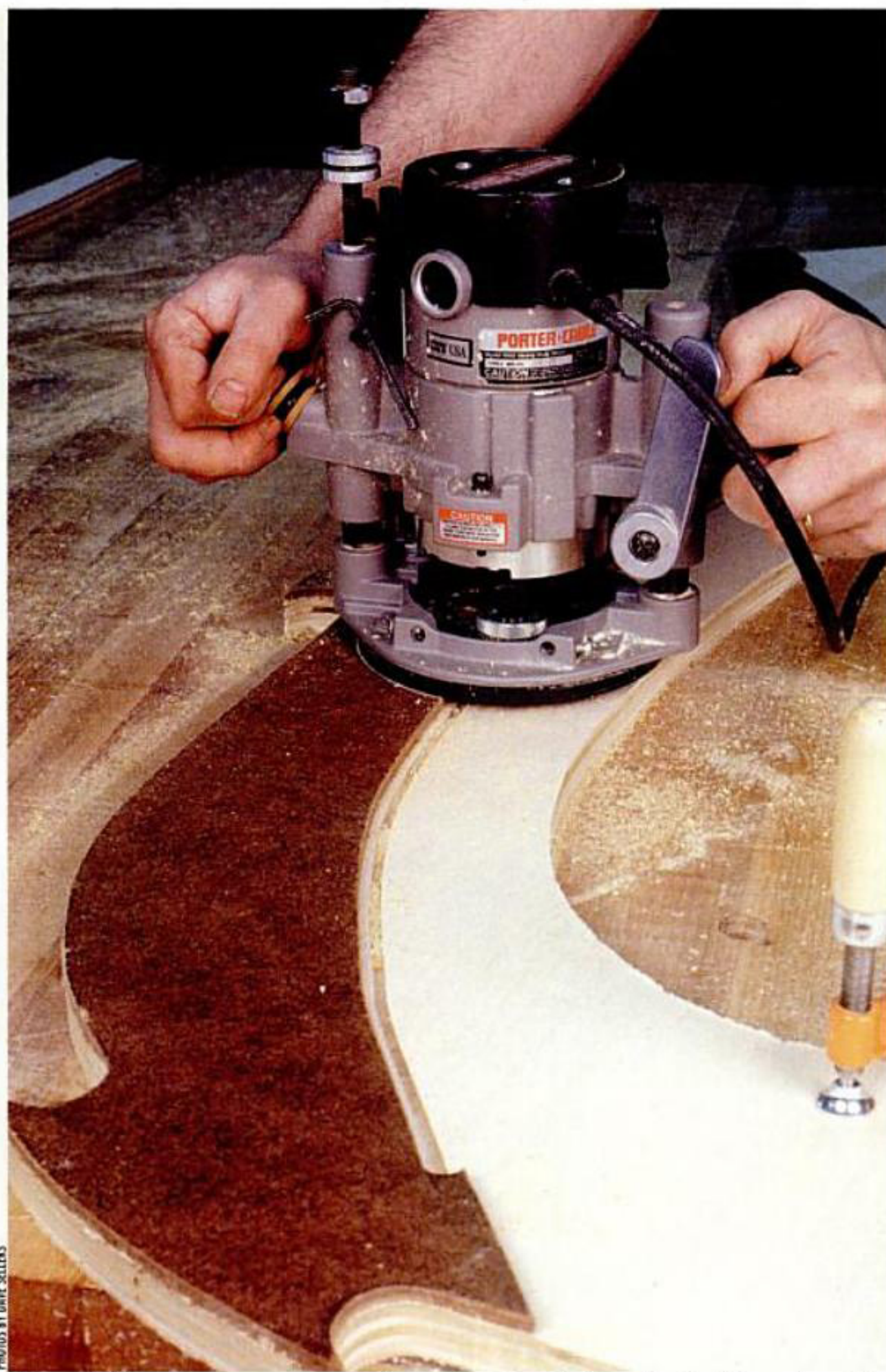
To rout the ramp groove, run the router template guide bushing along the edge of the template. The hole at the end of the template's curve provides a stop for the router.
