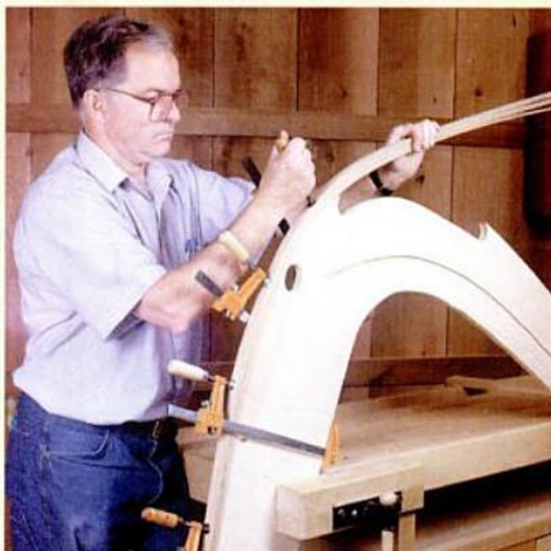
Form the curved handrails by gluing, bending and clamping a laminated stack of thin oak strips around the edges of the slide's sides.
