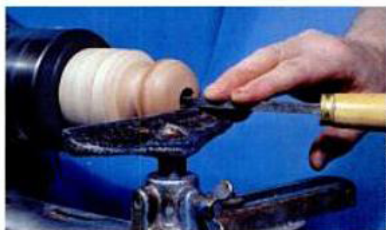
To refine the shape inside the globe, the author uses a shop-made bent-angle tool (top).
