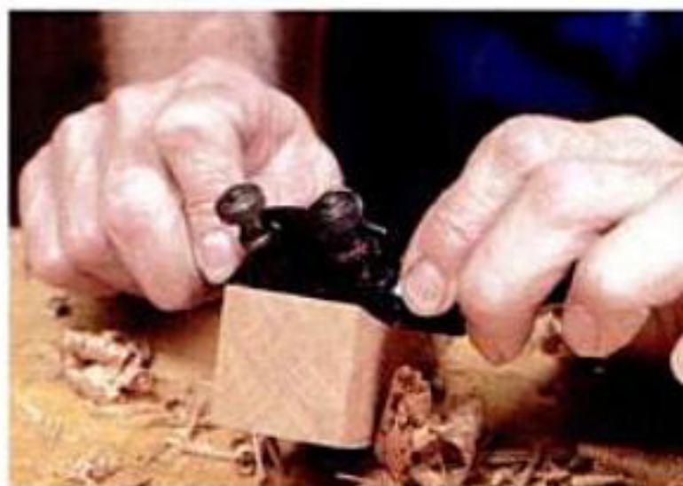
Frank Klausz uses his thumbs and forefingers to direct pressure to the front sole of the spokeshave on both push stroke (right) and pull stroke (left).
