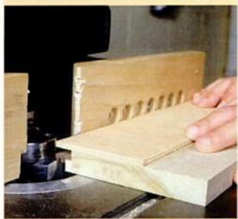
This simple plywood jig holds muntins safely for sticking and rabbeting.
