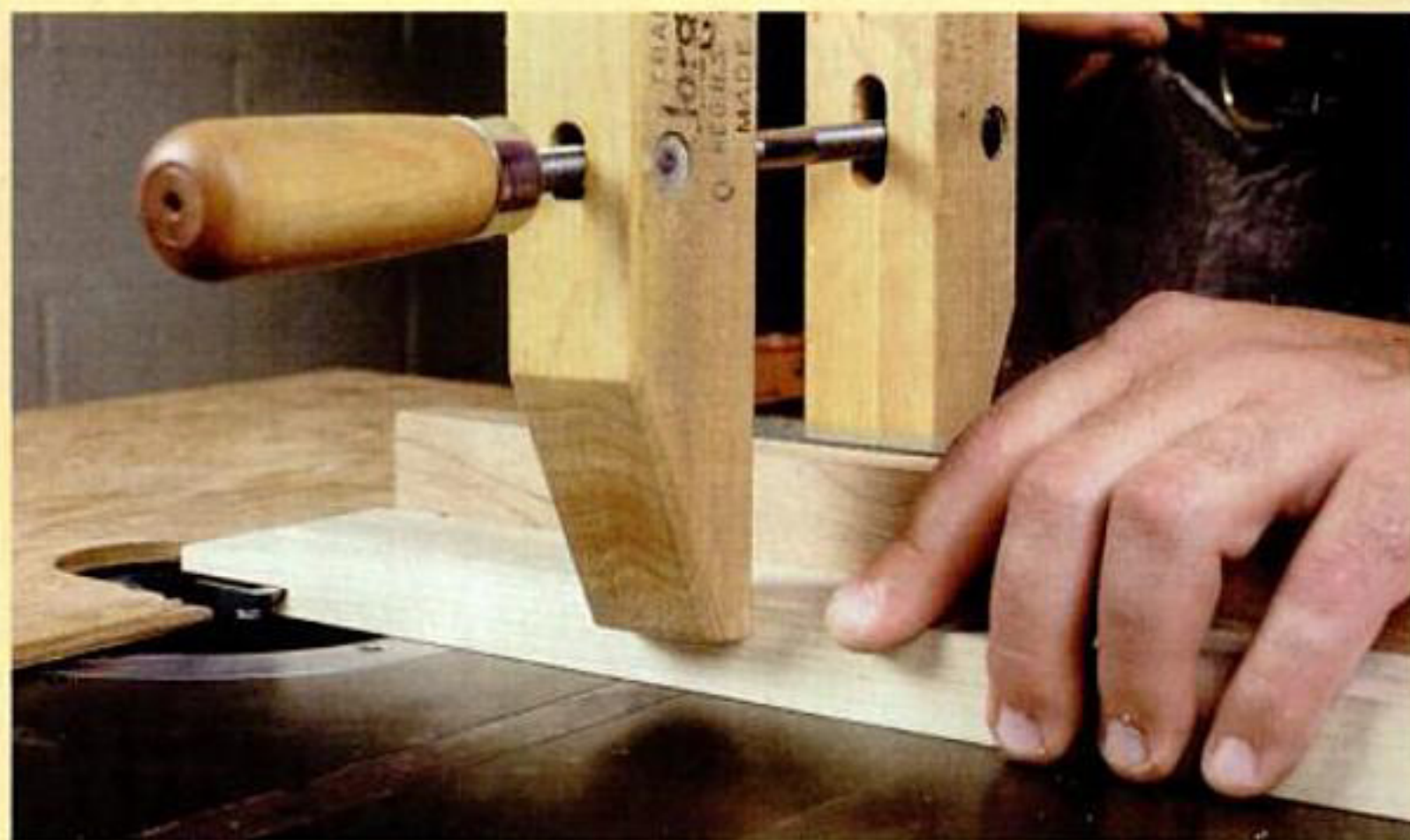
A cradle fence allows you to shape the face of a circular section. Stub spindle copes end of rail while allowing tenon to pass unobstructed.
