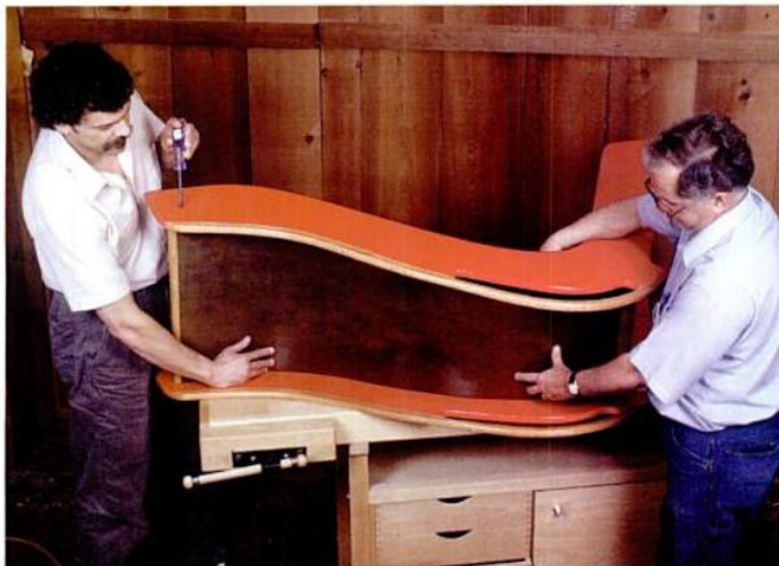
To assemble the slide, bend the hardboard ramp into the grooves in the side pieces as your helper starts the screws into the nosings and treads.
