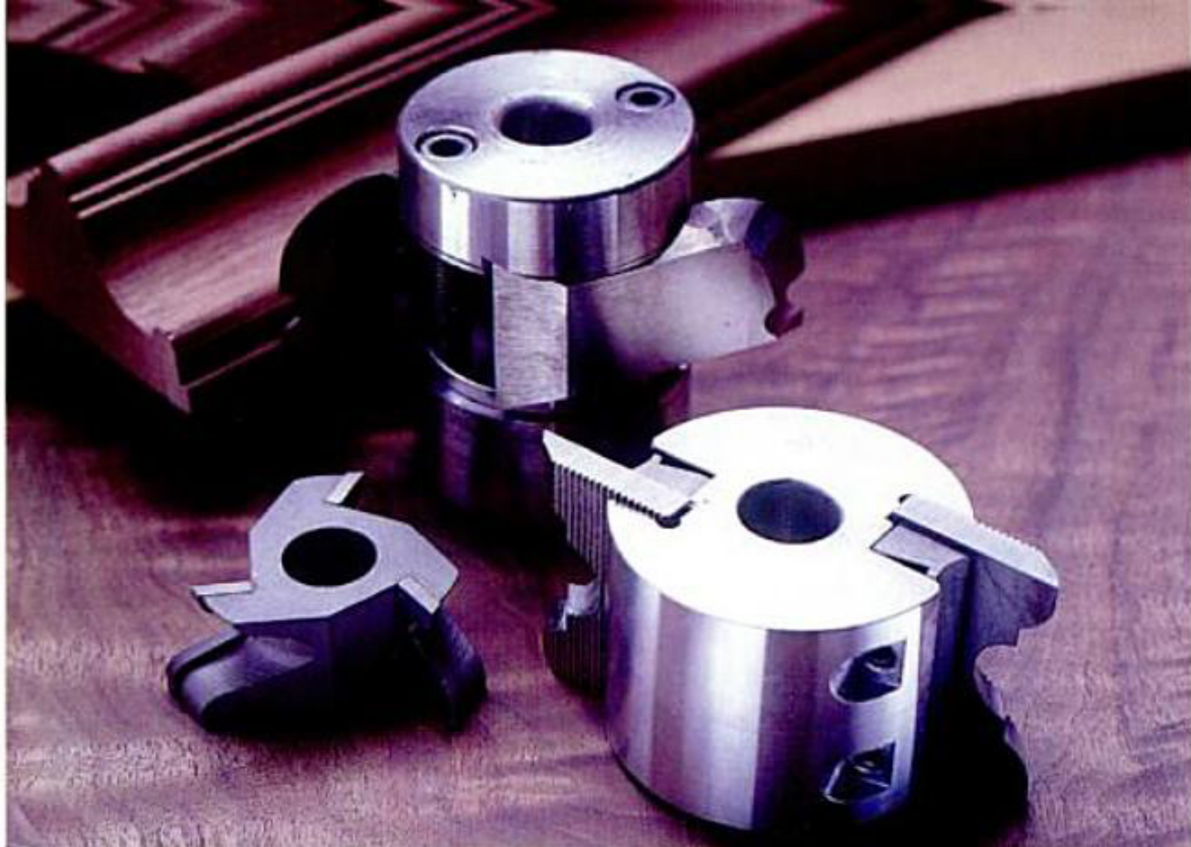
The three main cutterhead types are (counterclockwise from left) three-wing, gib-screw and bevel-edge cutters. Each has advantages for certain types of cuts.
