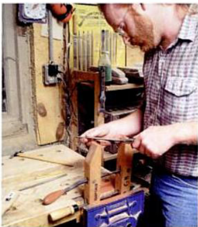
To bring the drawer handle up to a comfortable working height, the author holds it in a clamp in his vise.
