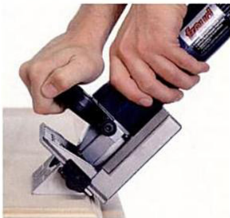
Biscuit-joiner fences work in different ways for cutting miter joints. Left: fixed 45° fences register against inside surface of work. Middle and right: Notched fences capture beveled edge.
