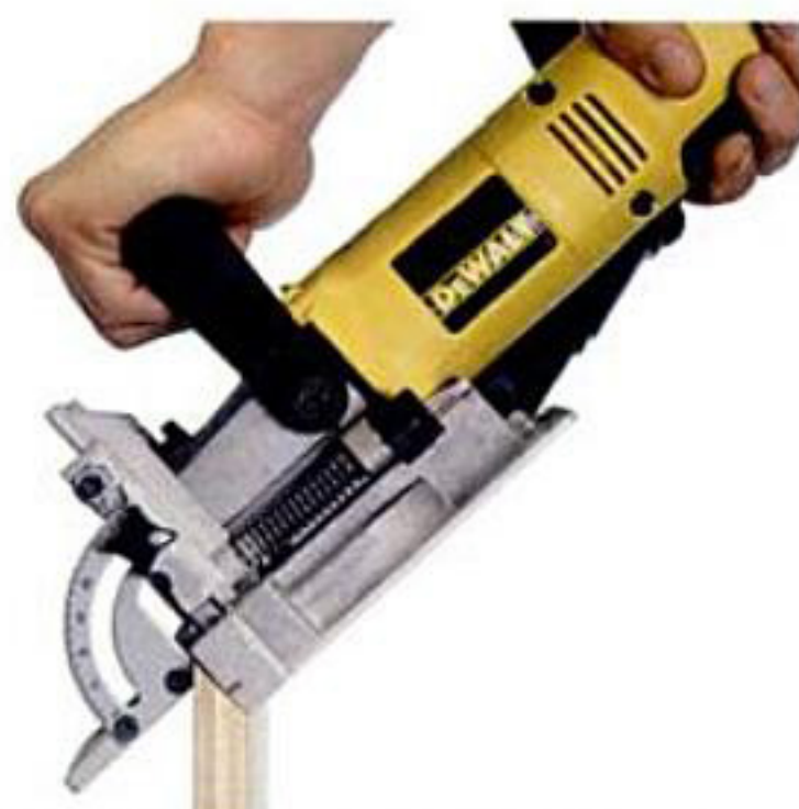
Biscuit-joiner fences work in different ways for cutting miter joints. Left: fixed 45° fences register against inside surface of work. Middle and right: Notched fences capture beveled edge.
