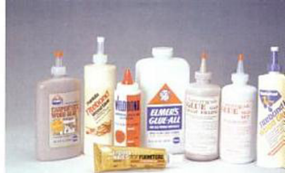
Polyvinyl acetate (PVA) glues are good for indoor woodworking, but only one type, Titebond II, withstands wet conditions.
