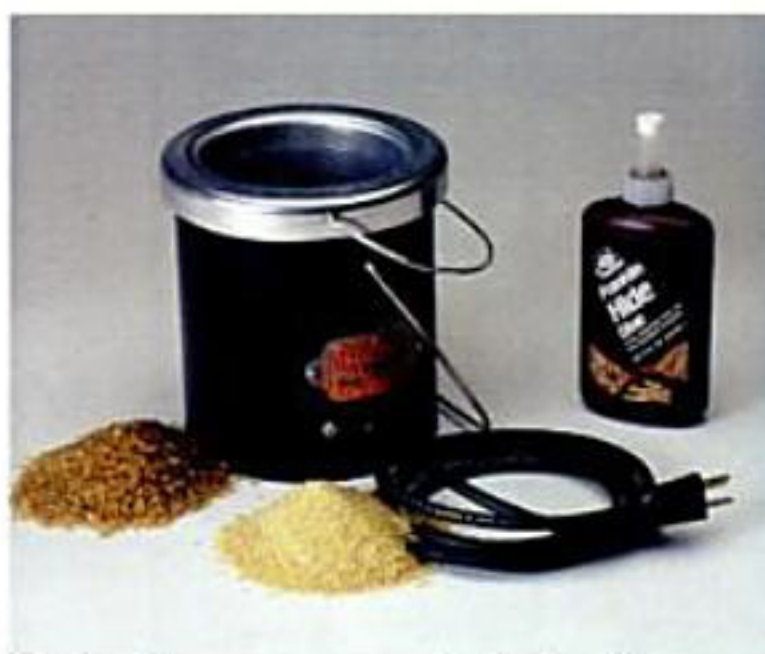
Hide glues are a good choice for joints that you may want to disassemble later.
