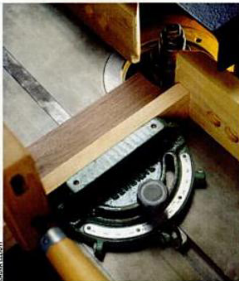
A miter gauge is a must for shaping the ends of narrow pieces. Hold or clamp stock firmly to avoid having it pulled into the rotating cutter.
