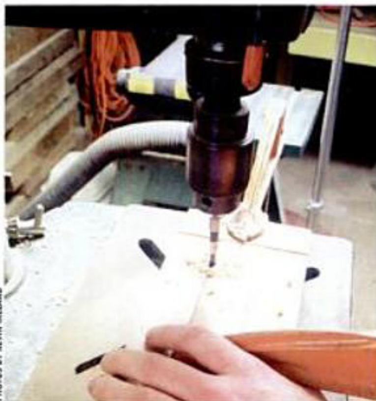
A U-shaped jig supports and locates the leg when drilling the foot.
