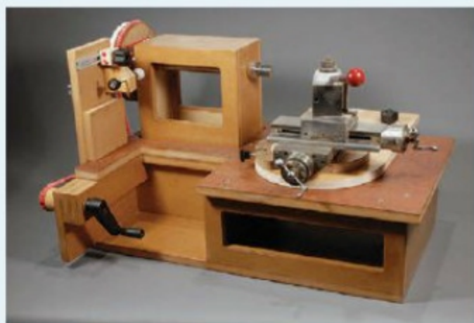
MDF Rose Engine with sliderest, 2007. Learn more about the MDF rose engine at rogueturner.com .
