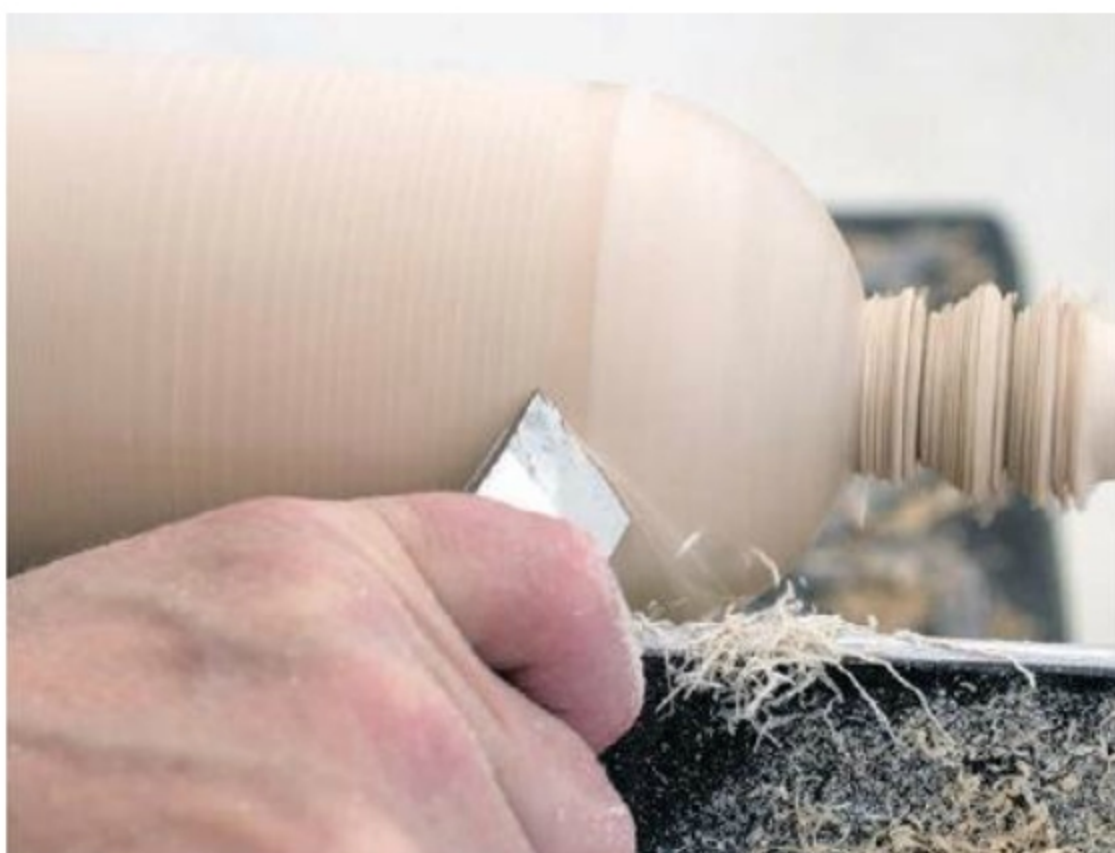
The fine "angel hair" shavings from a skew's shearing cut indicate a clean cut along the wood's sidegrain.
