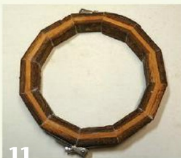
(10) Clamp the bark accent strips to the cherry support strip. Keep everything in line by clamping one strip at a time.
