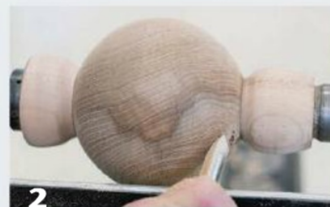
Direction of cut depends on grain orientation. At left, shear-cutting "downhill," from large diameter to small, on a sphere with the grain parallel to lathe bed. At right, shear-scraping "uphill," from small diameter to large, with sphere repositioned and its grain perpendicular to the lathe bed.
