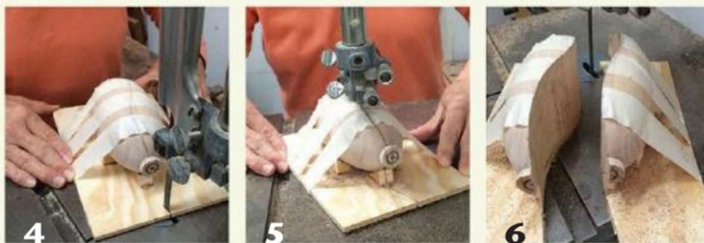
4 The author's pod cut in half on a curved line. The tenons at each end can be cut off after the pod is split.
