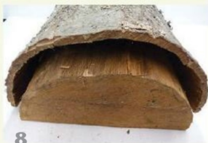
8 To harvest bark from an oak slab, drive narrow maple wedges between the bark and the wood.
