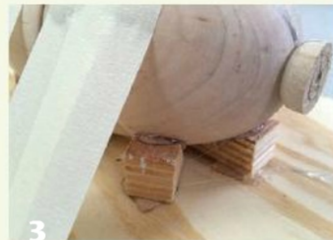
2 Workpiece is glued and taped to the wedges and carrier, ready to be cut apart on the bandsaw. Note the intended cut line for this pod form (along the sidegrain). The jig can also be used to cut across the grain to remove a tenon.
