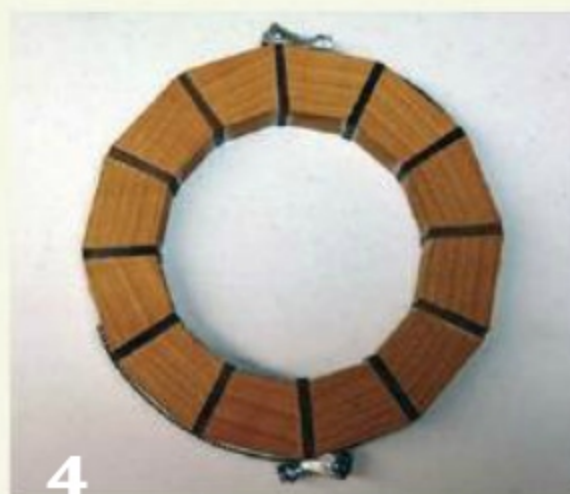
4 Use two hose clamps in tandem to glue up the first segmented ring, with walnut splines between the cherry segments.
