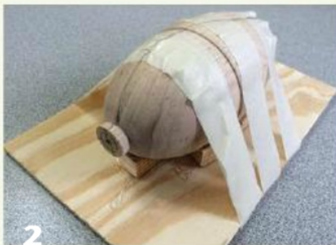
2 Workpiece is glued and taped to the wedges and carrier, ready to be cut apart on the bandsaw. Note the intended cut line for this pod form (along the sidegrain). The jig can also be used to cut across the grain to remove a tenon.
