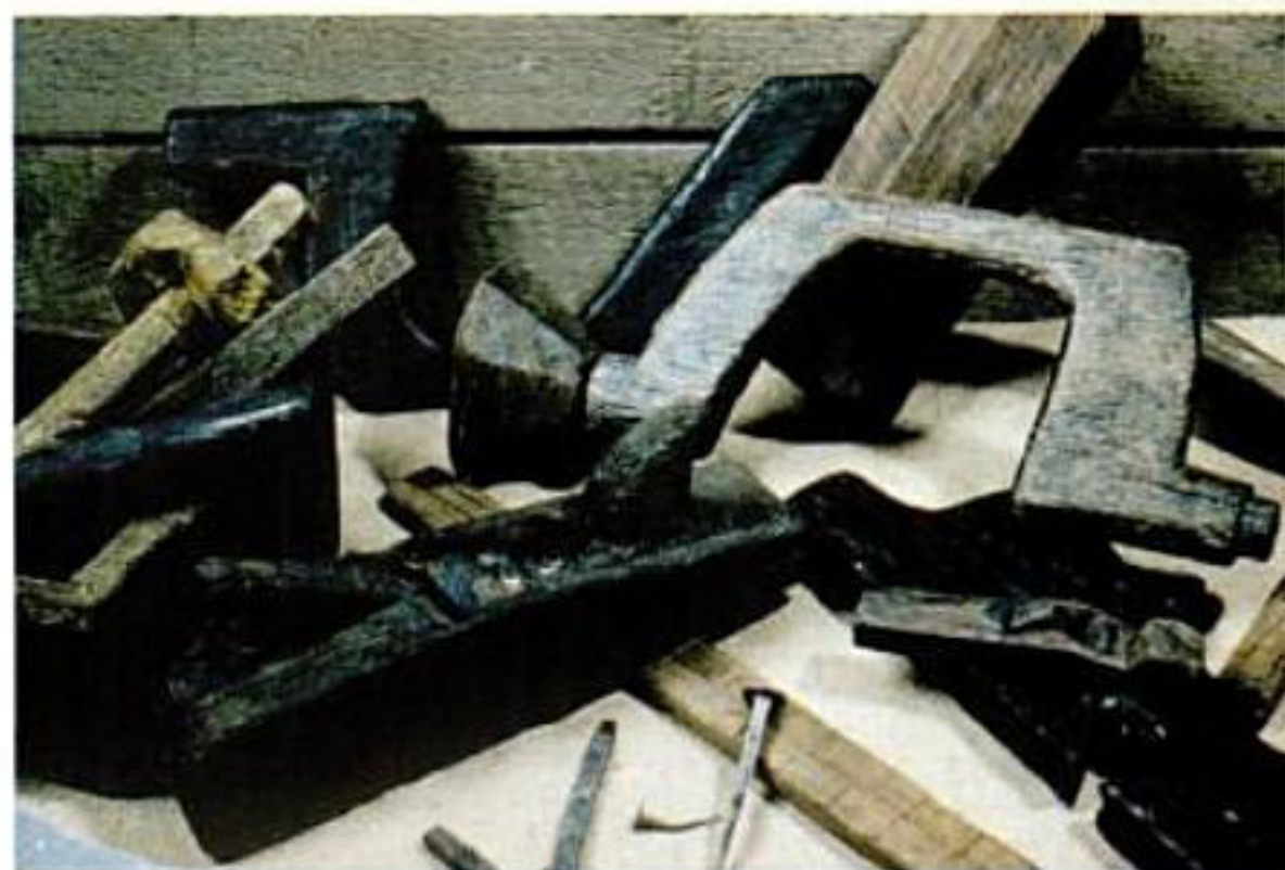
Most of these tools that divers recovered from the ship's carpenter's cabin will look familiar to present day woodworkers. The author held a modern rule alongside one recovered and found a discrepancy of only \frac{1}{4} in.
