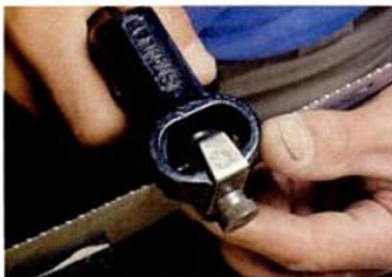
Before filing the teeth, use a mill file to joint the saw teeth level (left). Above, author uses a saw set to bend the teeth so they're set uniformly.
