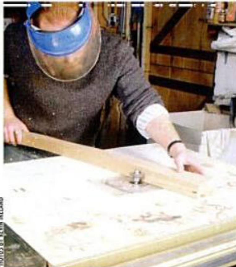
For safety and stability, rout the panel slot in the curved rail before sawing the upper arc of the curve.
