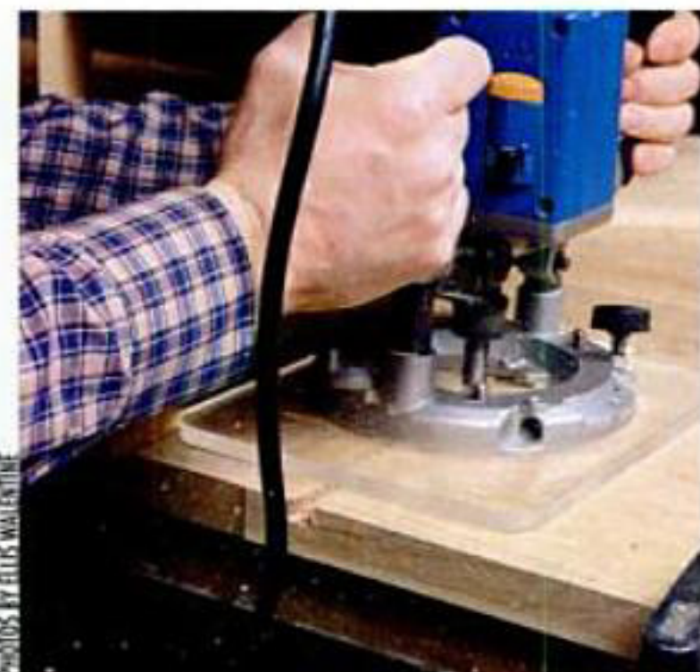
To rout dovetail grooves, guide hand-held router against a fence clamped across the workpiece. Cut the mating tongues on a router table.
