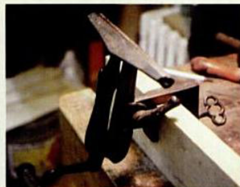
A magnifying visor, saw set and files (left) are some of the tools that make sharpening easier. To bring his antique saw vise to the proper height, author clamps it to a block of wood, then clamps wood in his bench vise (above).
