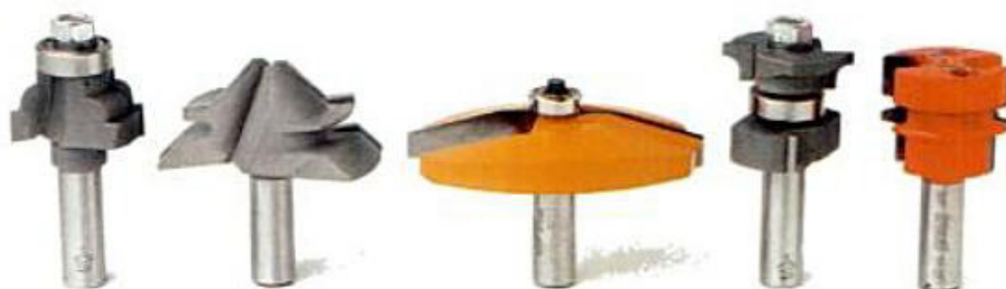
Left to right: rail cutter, lock-miter, anti-kickback panel raising, stile cutter, anti-kickback glue-joint.
