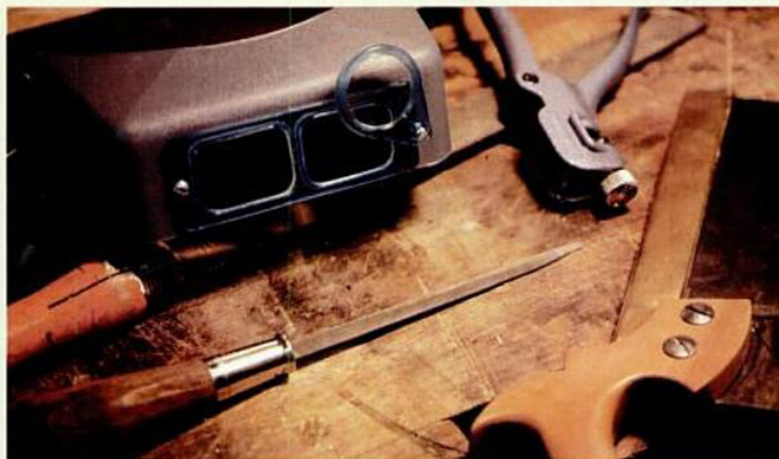
A magnifying visor, saw set and files (left) are some of the tools that make sharpening easier. To bring his antique saw vise to the proper height, author clamps it to a block of wood, then clamps wood in his bench vise (above).
