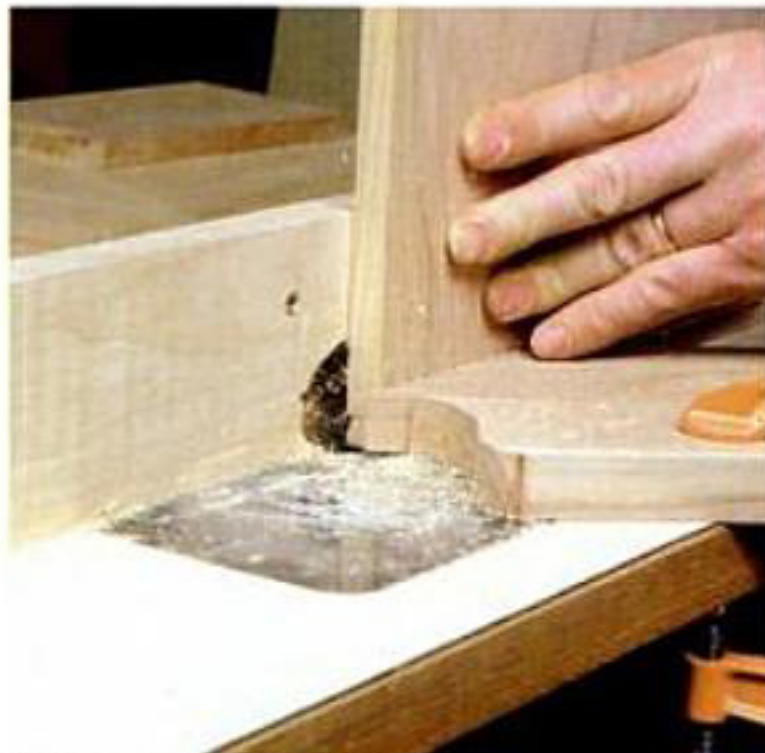
To rout dovetail grooves, guide hand-held router against a fence clamped across the workpiece. Cut the mating tongues on a router table.
