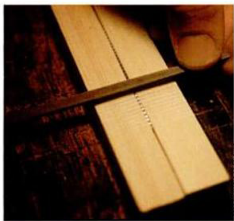
When filing saws with small teeth, author clamps saw between blocks of wood, letting the teeth protrude above blocks. When the file cuts into the wood, he moves on to next tooth.
