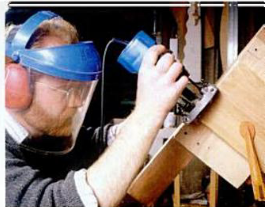
For strength, bed hardware should be mortised tightly into the legs and rails. A simple jig gives the router stability.
