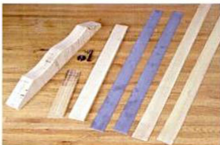
The basic ingredients of a laminated bow are hard wood and thin, uni-directional fiberglass strips.
