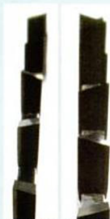
A thin-kerf blade, left, requires less horsepower and wastes less wood than a regular blade, right.
