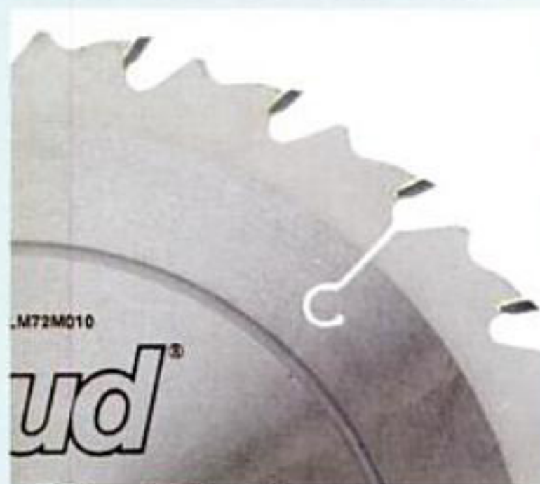
High shoulder extensions limit the depth of cut to minimize kickback on this rip blade.
