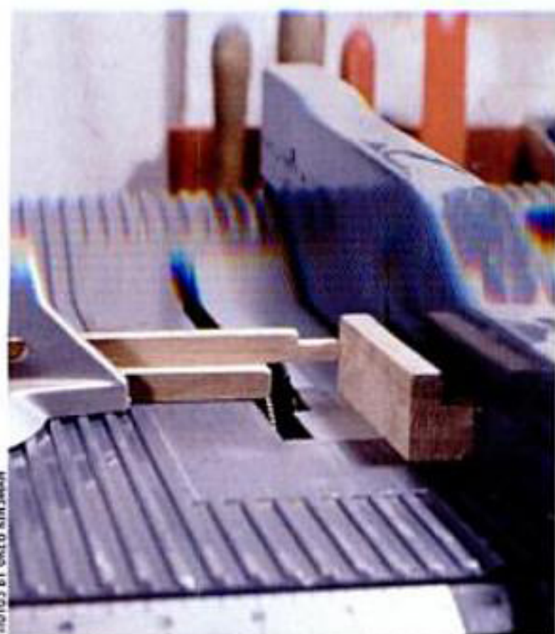
Cut the tenons on the muntins with a dado head, using a gauge block against the rip fence to determine the shoulder locations.
