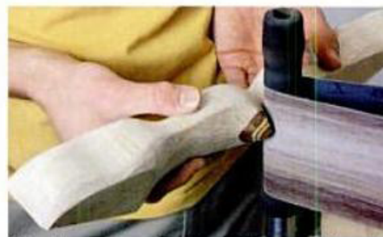
To shape the riser handle, use a hand-saw and belt sander.
