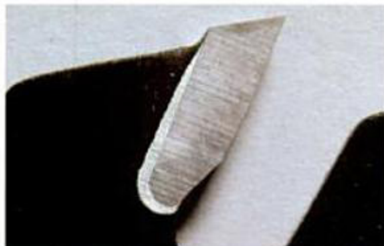
Good and bad blades: Poor brazing and rough grind marks on tooth at left are a tip-off to a cheap blade that will never cut smoothly. At right is the smooth brazing and fine grinding common on a high-quality blade.
