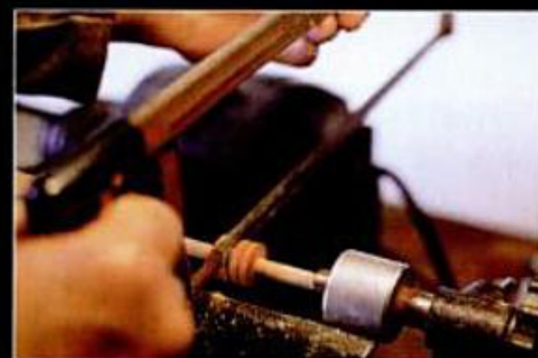
With the lathe spinning, author uses a hacksaw to part the pivot pins.
