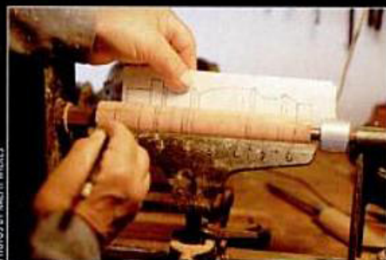
Author holds template against spinning workpiece and marks key diameters with a pencil.
