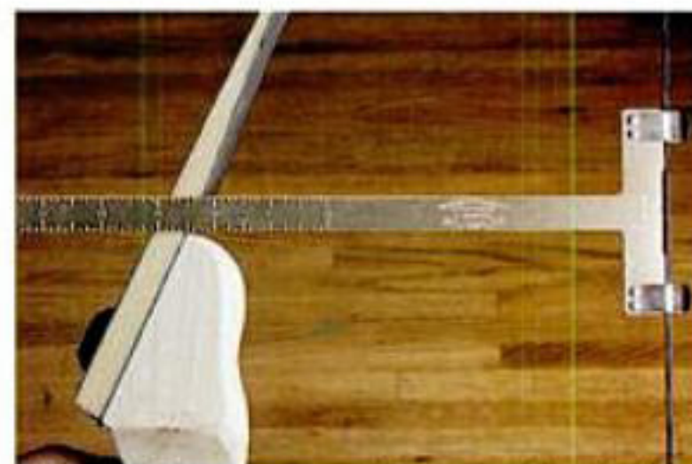
To check symmetry between the limbs, measure from the string to the ends of the riser. The upper limb should have \frac{1}{4} in. more bend than the lower one.
