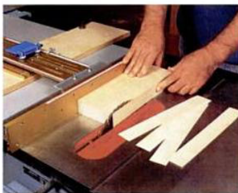
Sawing uniform veneer or laminates as thin as 1/32 in. is a snap with a positioning jig.
