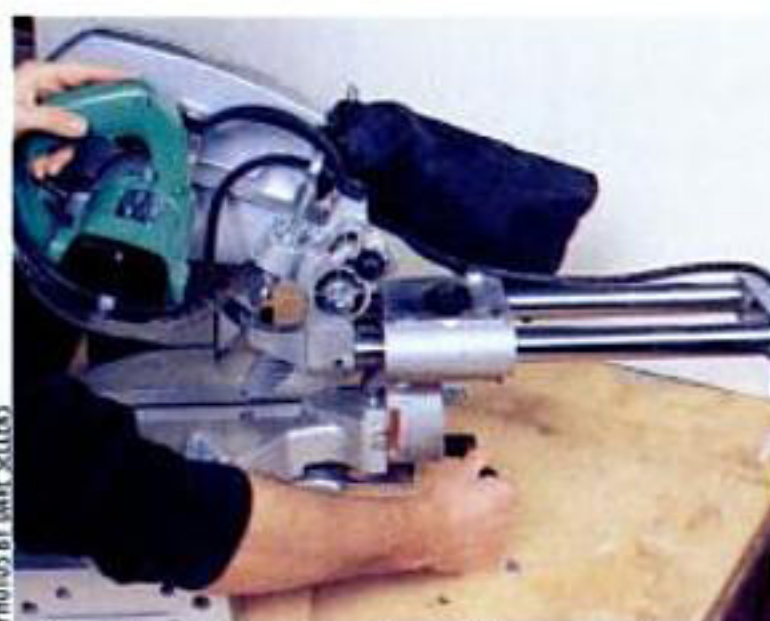
PHOTOS BY DAVID SELLERS To adjust the bevel cutting angle on the Hitachi (shown), Sears and Makita saws, you have to reach to grip the rear-mounted bevel lock lever. The bevel scale is just left of the lever.
