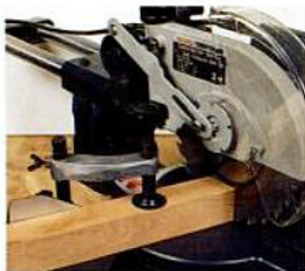
Auxiliary work vise (standard on Sears and Makita, optional on others) keeps the stock from shifting during the cut (above.)
