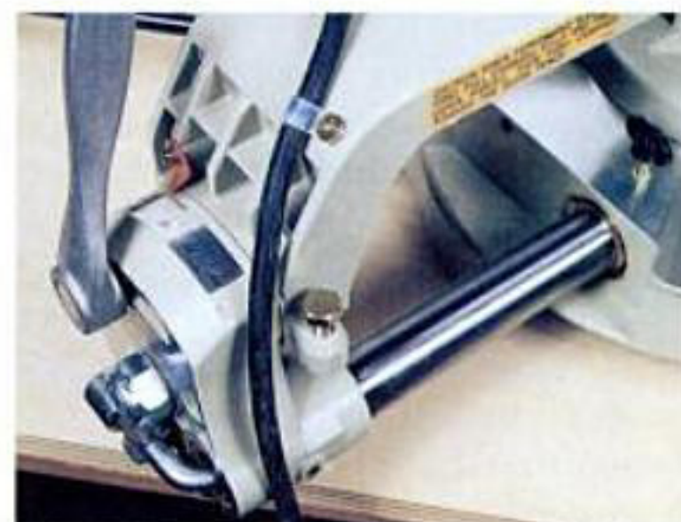
The Makita's single sliding rod is just as rigid as the twin rods on other saws, and moves very smoothly. Note bevel lock lever and scale at left.
