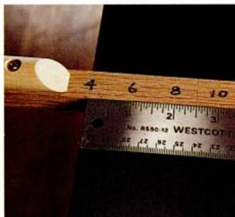
To calibrate jig, make knife marks at 1/2-in. intervals on the adjustable slide bar.
