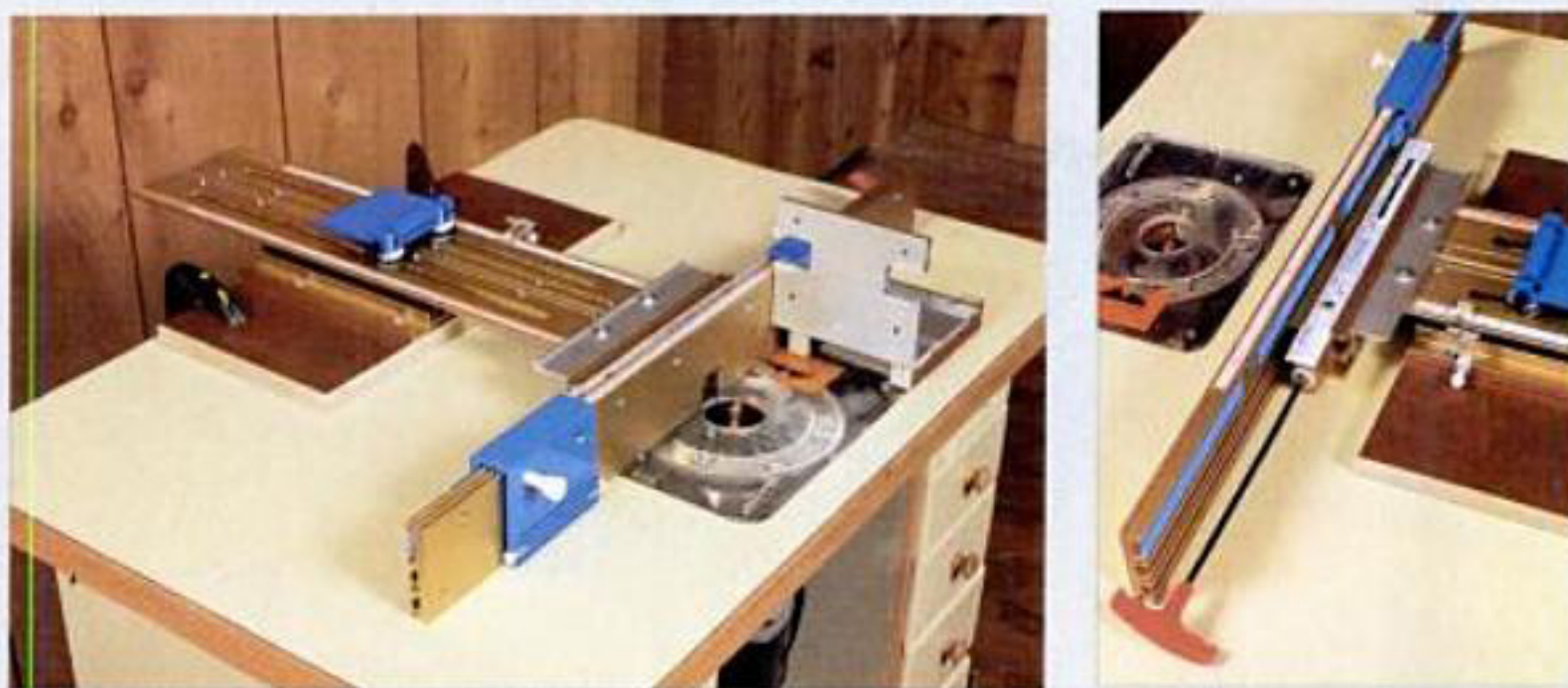
The INCRA Jig Pro model, above left with optional 28-in. fence, right angle fixture and stop block. (Price as tested: $239.80.) The optional micro-positioning feature, above right, permits fence adjustment within 0.001 in.
