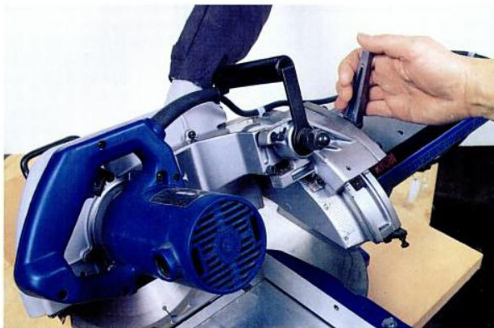
Ryobi's bevel scale and lock lever are more accessible than rear-mounted ones. The cutterhead tilts by moving on curved trunnions.
