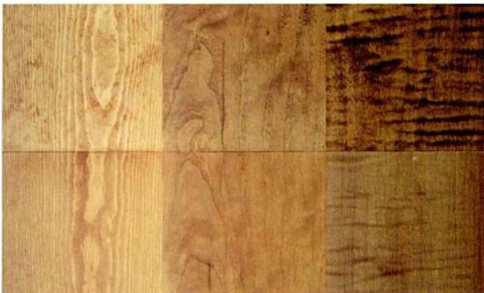
Liquid stains (top row) cause splotching on pine (left) and cherry (center), but highlight the figure of curly maple (right). Gel stains (bottom) stain all three evenly because they penetrate less.
