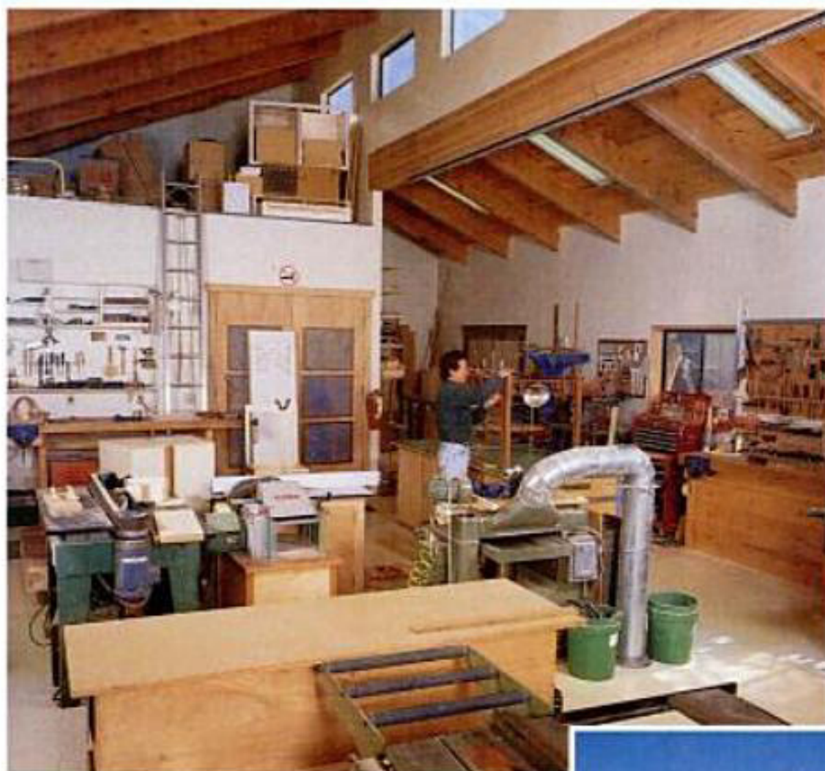
South-facing clerestory windows, left and below, provide excellent natural light all the way to the back wall of Peter Axtell's California workshop.
