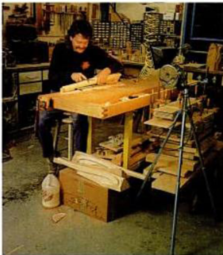
The strong shadows raised by an oblique side or back light are ideal for defining carved highlights or spotting sanding scratches and finish flaws. Roger Heitzman made this detailing lamp by mounting a cheap quartz-halogen floodlight on a camera tripod and wiring it with a retractable cord reel from a used vacuum cleaner.
