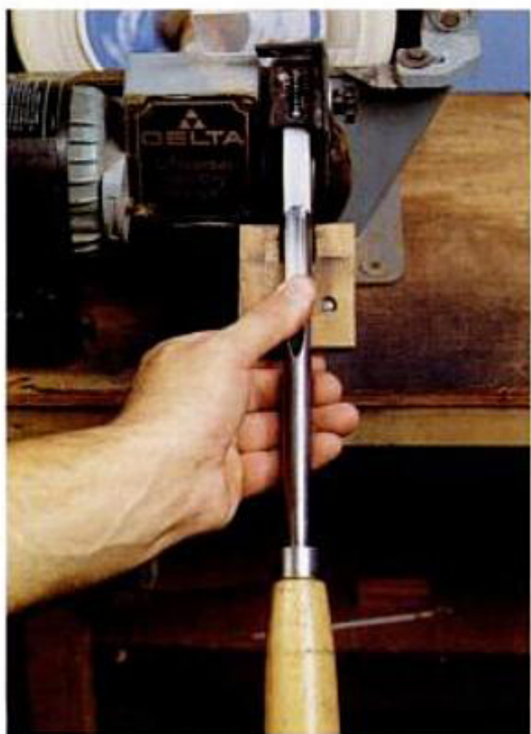
To grind the other side, switch hands and start at the midpoint again (left). Roll the gouge to the left, swinging the handle to the left, as you roll.
