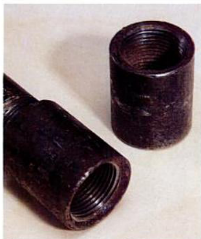
The author used threaded connectors to extend his pipe clamps for long work.
