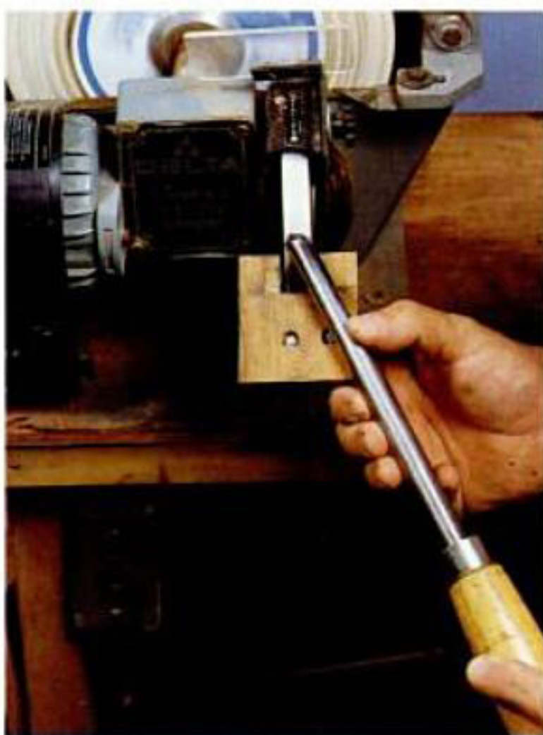
It's easiest for beginners to grind each half of a fingernail profile separately. Starting in the midpoint (top left), roll the gouge to the right, swinging the handle to the right as you roll the tool (top right).
