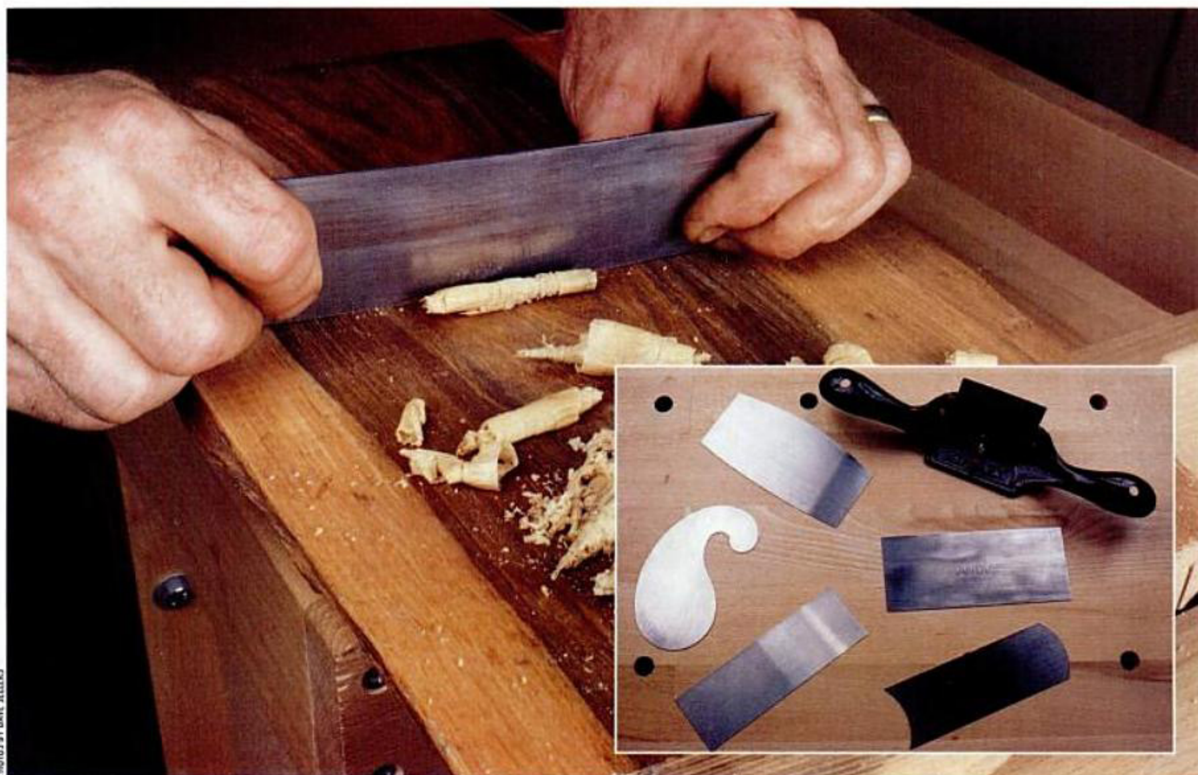
Planes and sandpaper aren't the only way to prepare wood for finishing. Author shows how easy it is to use a scraper. Scrapers come in different sizes and shapes to fit the contours of your work (inset).
