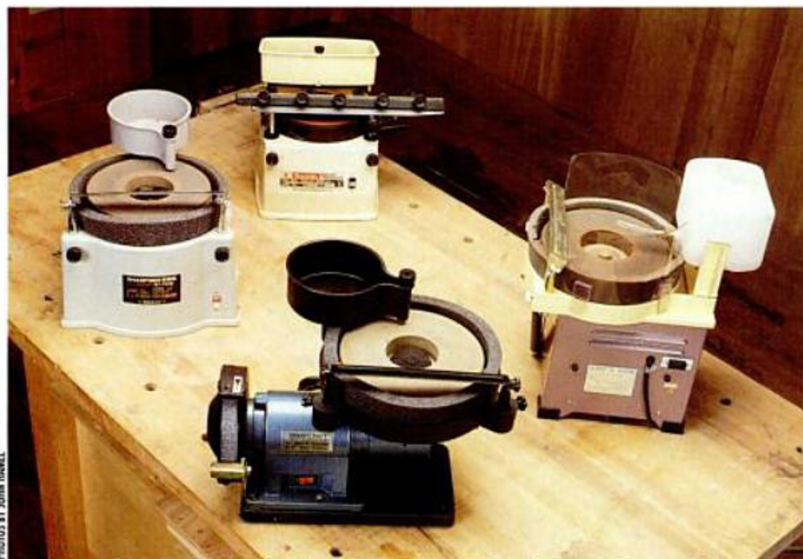
Horizontal, water-cooled grinders produce a flat bevel and a superior edge. Counterclockwise from rear: the Makita comes with a jig for grinding planer and jointer knives, an option on the Matsunaga grinder, Woodcraft's combo has a high-speed wheel for rough grinding, the Rakuda sports a sheet-steel housing instead of plastic.
