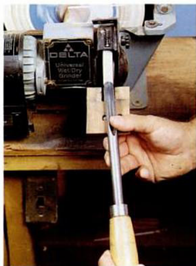
It's easiest for beginners to grind each half of a fingernail profile separately. Starting in the midpoint (top left), roll the gouge to the right, swinging the handle to the right as you roll the tool (top right).
