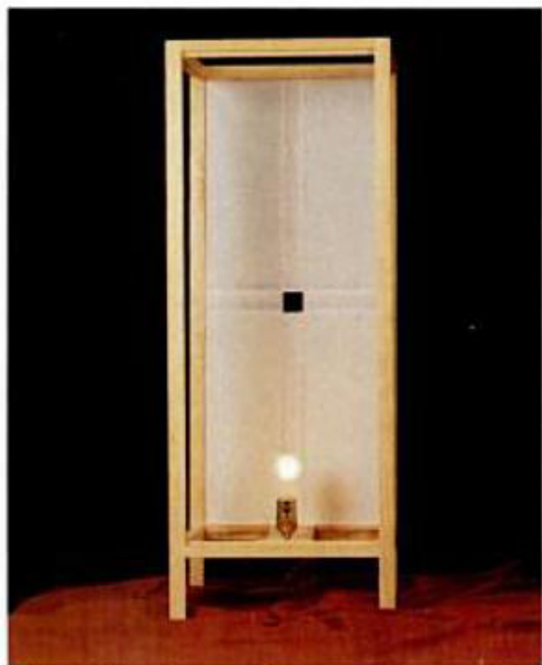
The light fixture attaches to a maple strip that is screwed to two rabbeted blocks. The blocks are screwed and glued to the rails.
