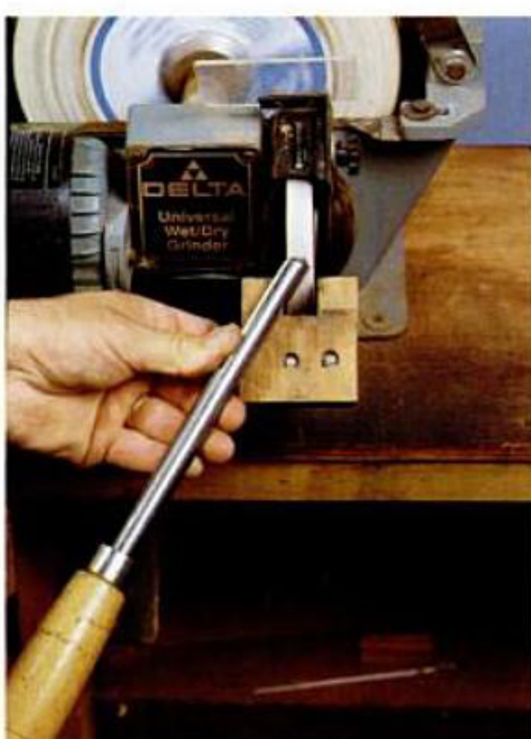
To grind the other side, switch hands and start at the midpoint again (left). Roll the gouge to the left, swinging the handle to the left, as you roll.
