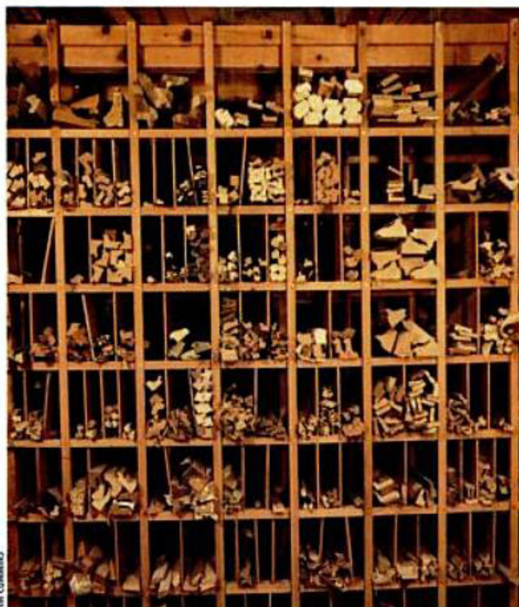
This molding rack made from 1x1s is a series of hanging grids extending back 12 ft. You can use similar small-scale racks to store dowels, scrap or other long and thin stock.
