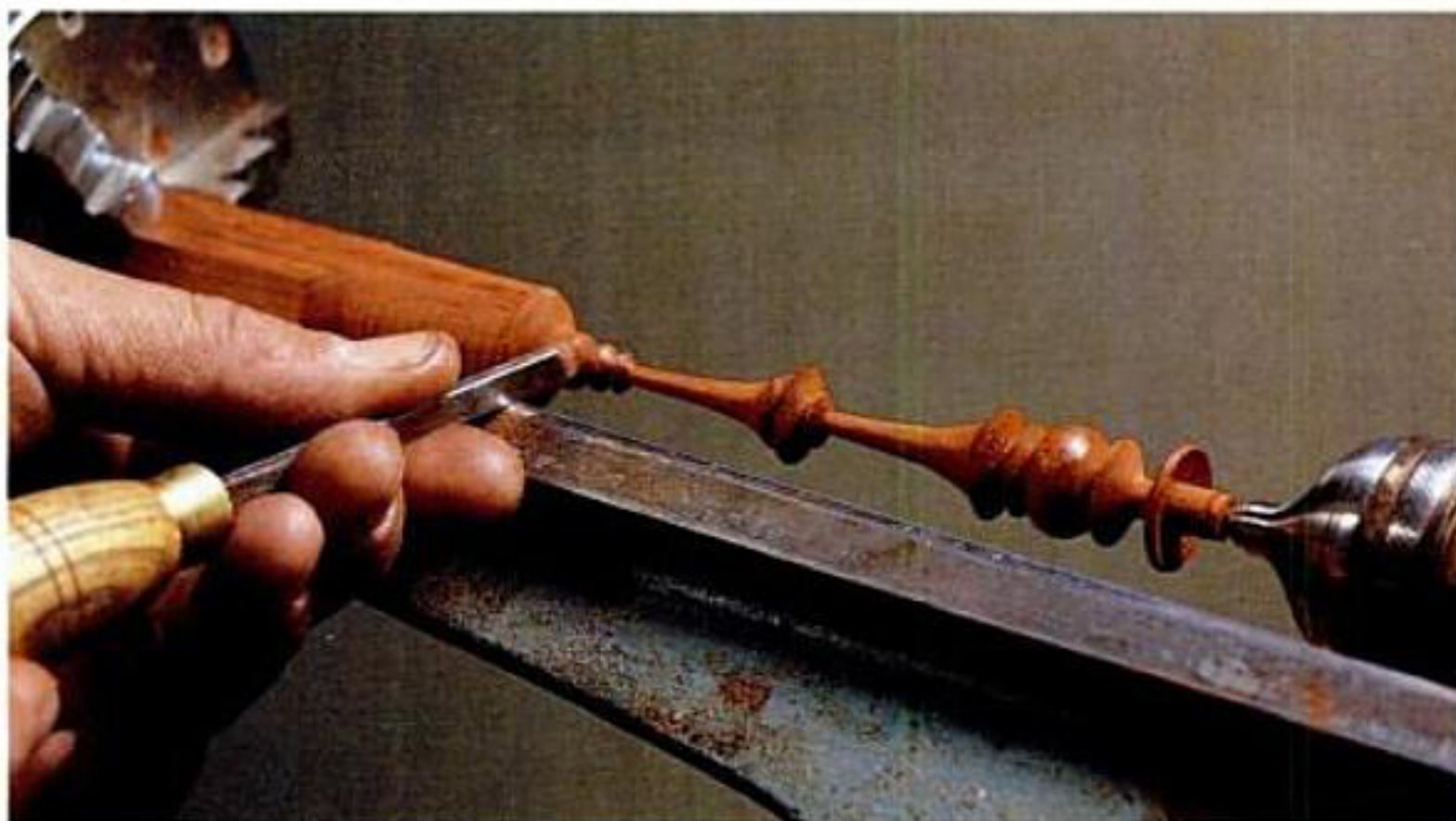
Turn the decorative spindles for the main ornament between centers. A \frac{1}{4} -in. dia. tenon turned on one end fits the center hole of the ornament.
