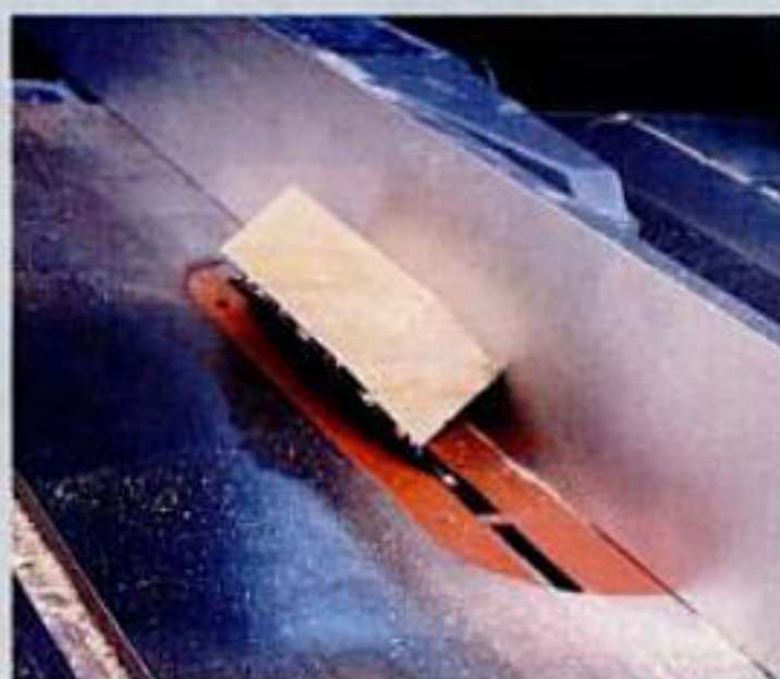
Woodturners can reduce scrap and check stock for defects at the same time by sawing square blanks into octagons. The no-math, no-measurement trick shown in these two photos sets the saw fence at the perfect distance to produce an octagonal turning blank. Tilt the blade to 45°. Rest the squared stock against the blade (left), and bring the fence up until it touches the corner of the stock. Then lay the wood flat and run it by the blade to remove the corners. The same idea works on the band-saw with the table tilted to 45°.
