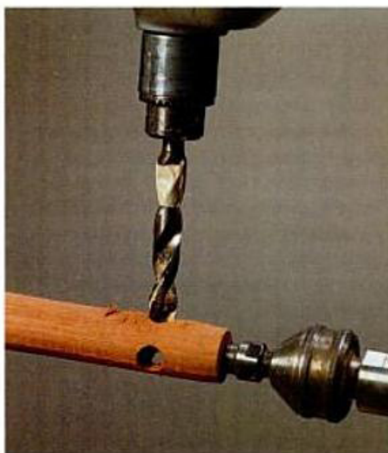
Bore out the small, interior ornament with a \frac{1}{2} -in. dia. brad-point bit in a hand-held drill, as shown at left. The three holes make it appear that the tiny piece is also hollowed. After boring the small ornament, round off the outside of the drilled area and turn two decorative ends, as shown above.
