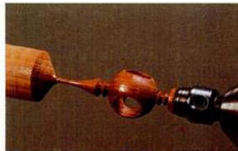
Bore out the small, interior ornament with a \frac{1}{2} -in. dia. brad-point bit in a hand-held drill, as shown at left. The three holes make it appear that the tiny piece is also hollowed. After boring the small ornament, round off the outside of the drilled area and turn two decorative ends, as shown above.
