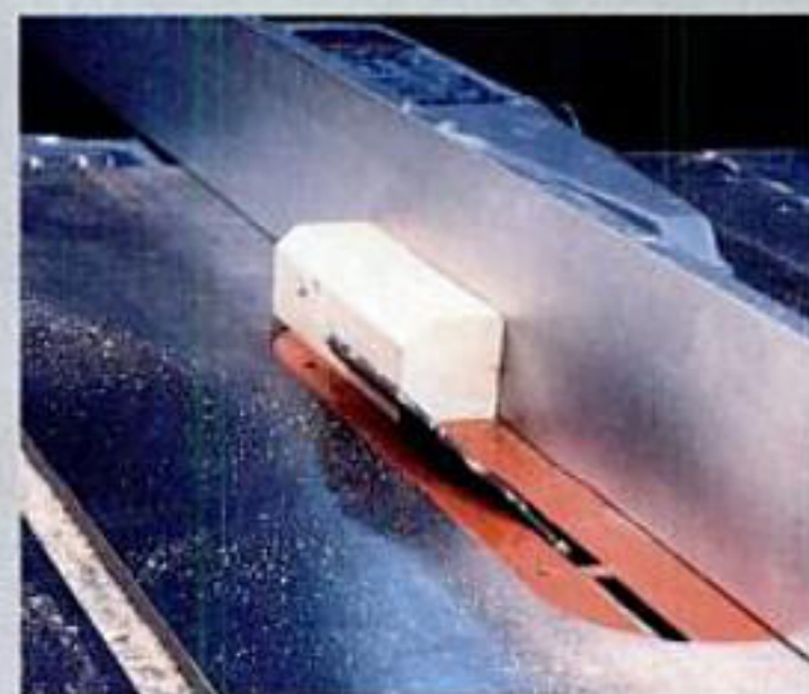
Woodturners can reduce scrap and check stock for defects at the same time by sawing square blanks into octagons. The no-math, no-measurement trick shown in these two photos sets the saw fence at the perfect distance to produce an octagonal turning blank. Tilt the blade to 45°. Rest the squared stock against the blade (left), and bring the fence up until it touches the corner of the stock. Then lay the wood flat and run it by the blade to remove the corners. The same idea works on the band-saw with the table tilted to 45°.
