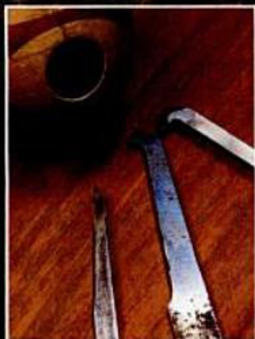
Author uses several offset round-nose scrapers, made from planer blades or high-speed steel, to hollow the interior.
