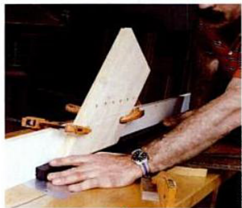
Round the cabinet posts on the router table, using feather boards to keep the flat faces firmly against the table and fence.
