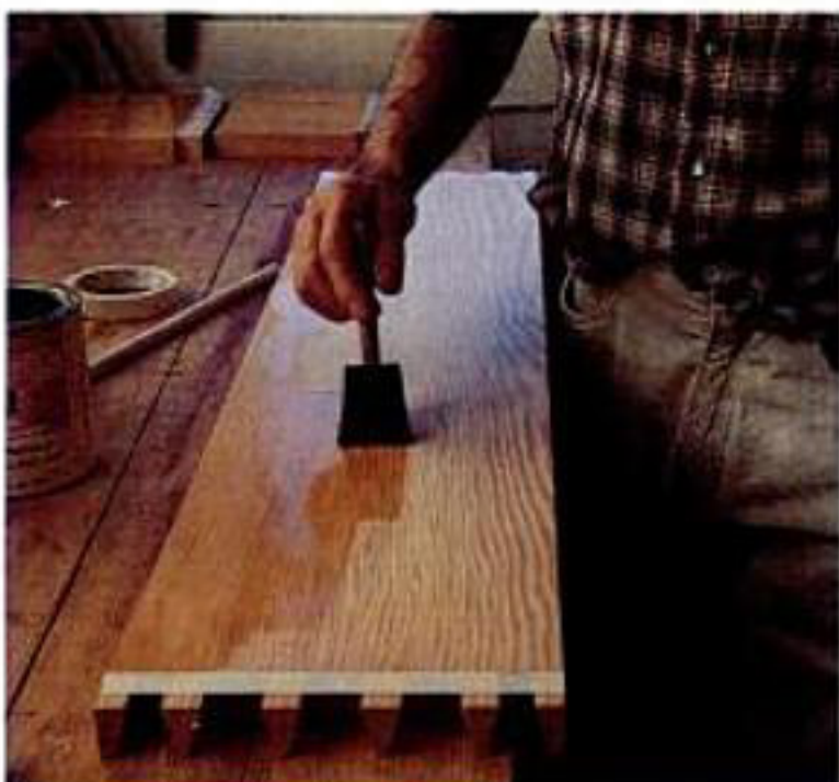
When applying a finish before glue-up, be sure to mask off all glue surfaces.
