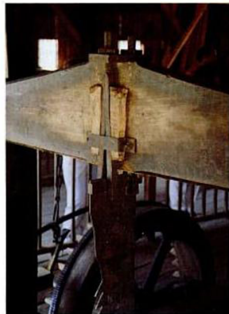
Though it's slow, the sawmill's 6½-ft. long, 7-in. wide blade has massive 1-in. long teeth that cut deeply on each pass.
