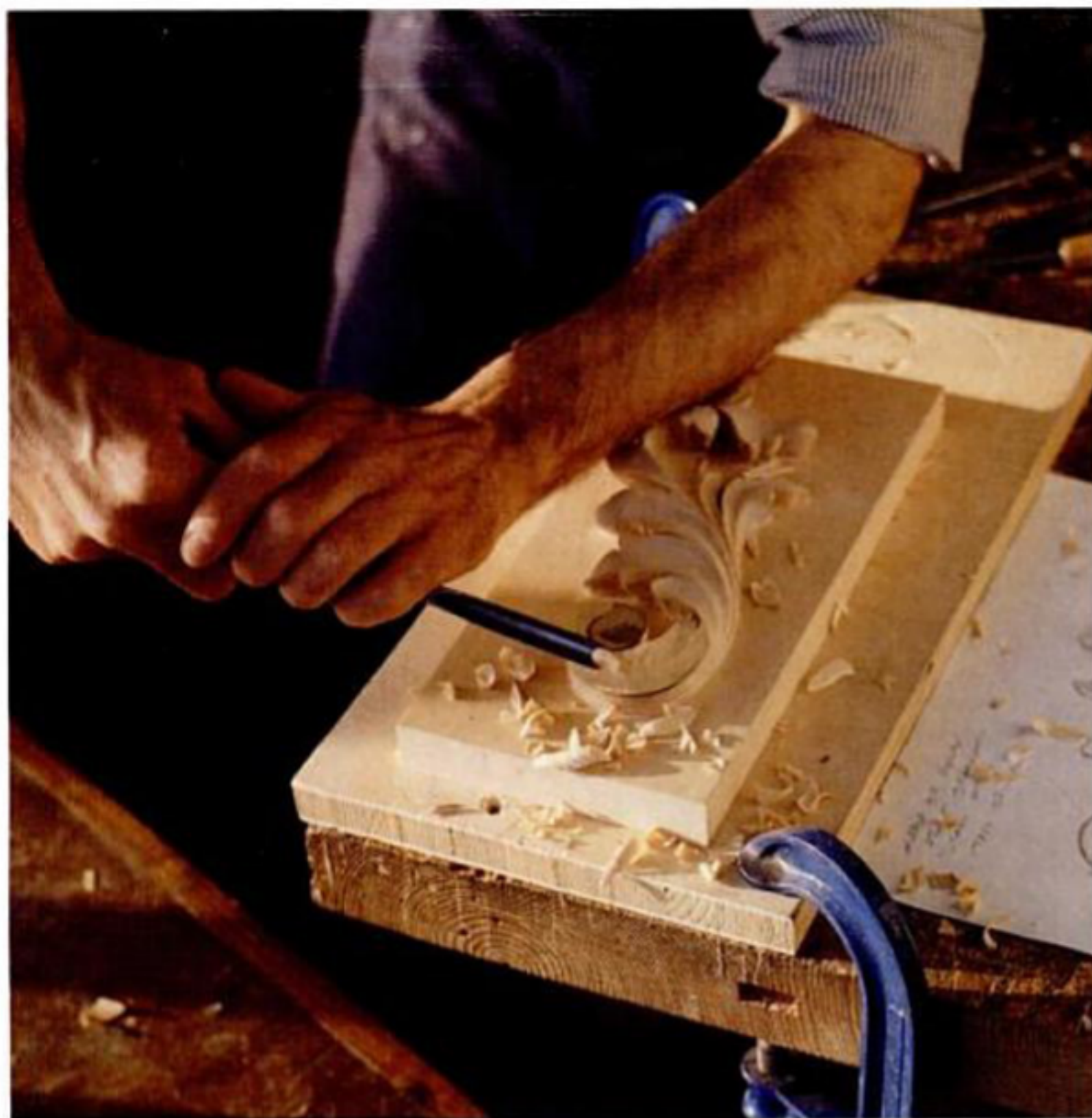
11. To form the scroll, start by carving the general slope of the scroll ridge, ending the slope at the channel carved earlier.
