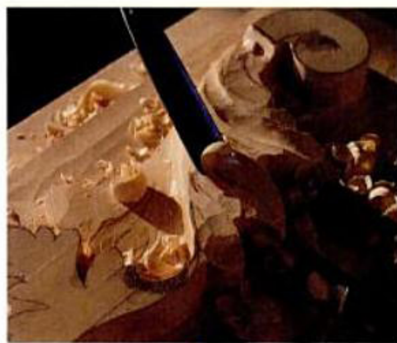
8. To model the lobes, use gouges and fluters to hollow out the areas between the pipes. This will create ridges that form the pipes and valleys that make up the lobes.
