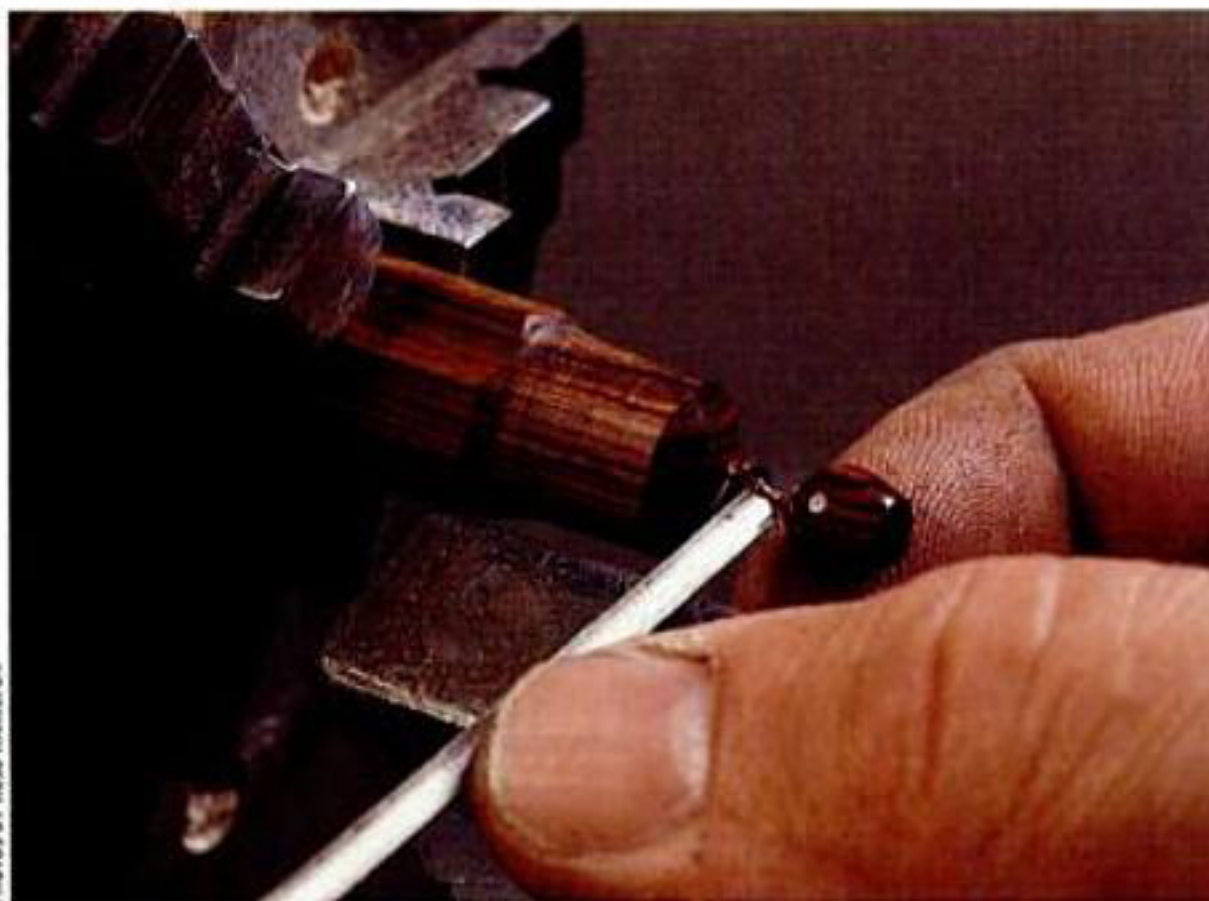
Author's index finger supports the work from behind to dampen vibrations that can cause the tool to catch.
