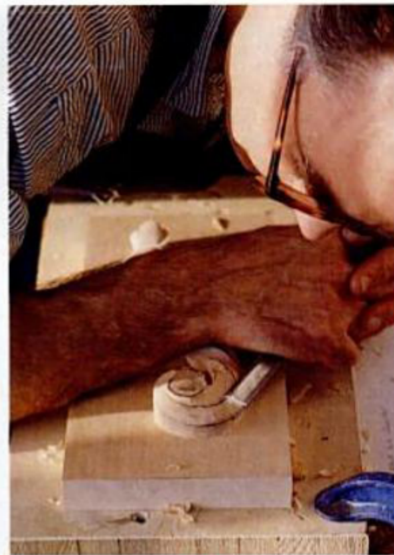
12. To model the convex portion of the scroll, carve down around the slope with a gouge held upside down.
