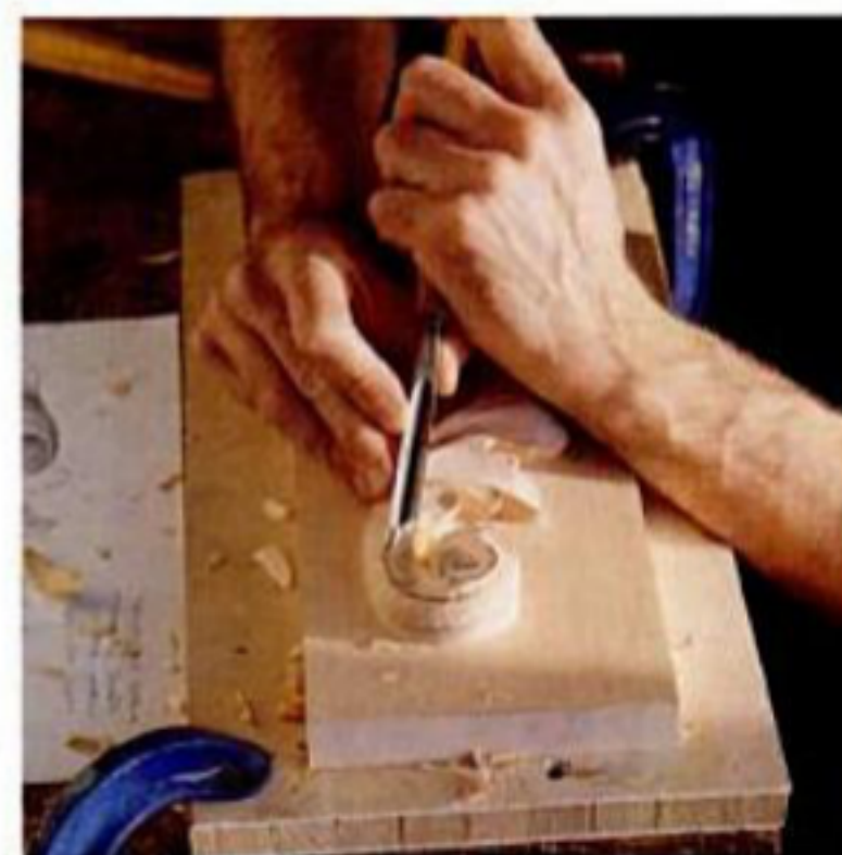
13. Hollow out the concave portion with a gouge held right-side up.
