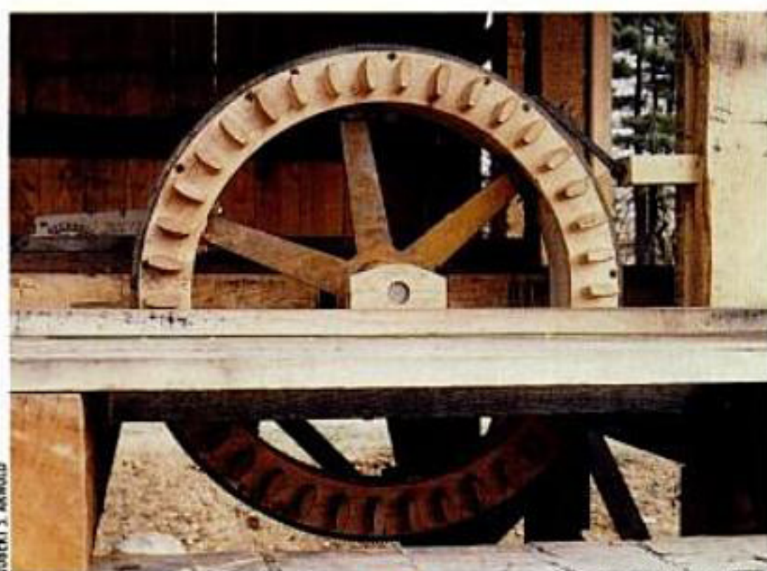
The cogged rag wheel advances the log through the saw blade by means of a rack-and-pinion mechanism.
