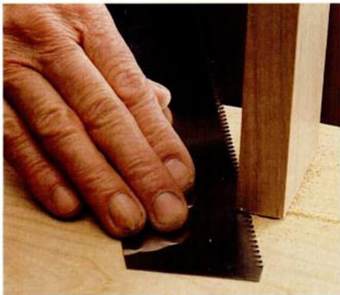
Author saws around rails' tenon shoulders so they'll seat firmly against the headboard and footboard.
