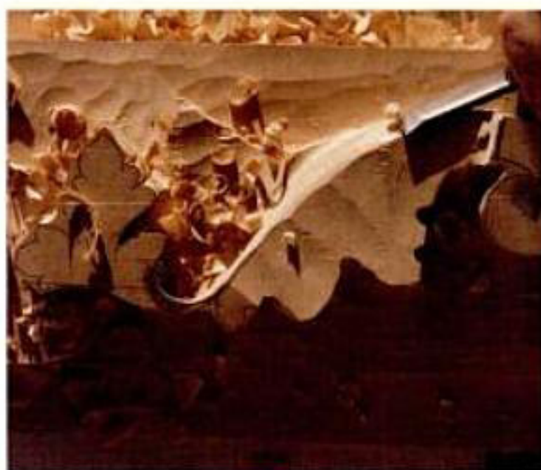
7. Round over the main stem of the leaf with a wide gouge held upside down, following the ridge of the main pipe. Work from the scroll toward the middle of the leaf.
