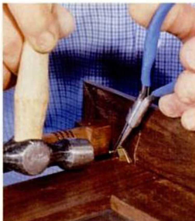
The door hinges pivot on brass escutcheon pins. It's easier to drive the pins if you hold them with a pair of pliers.
