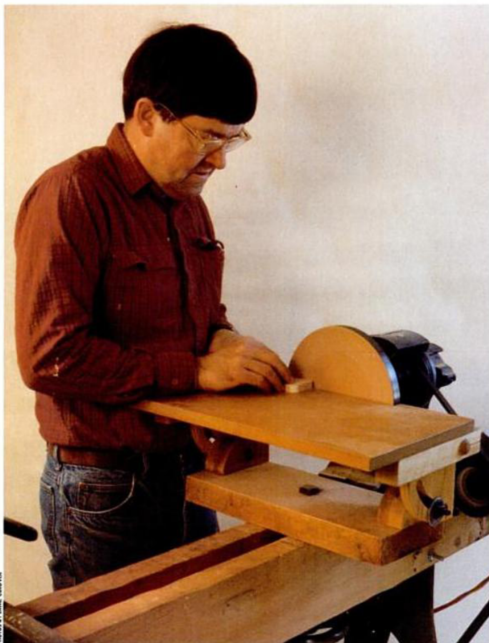
Convert your lathe to a disc sander with this simple tilting table.
