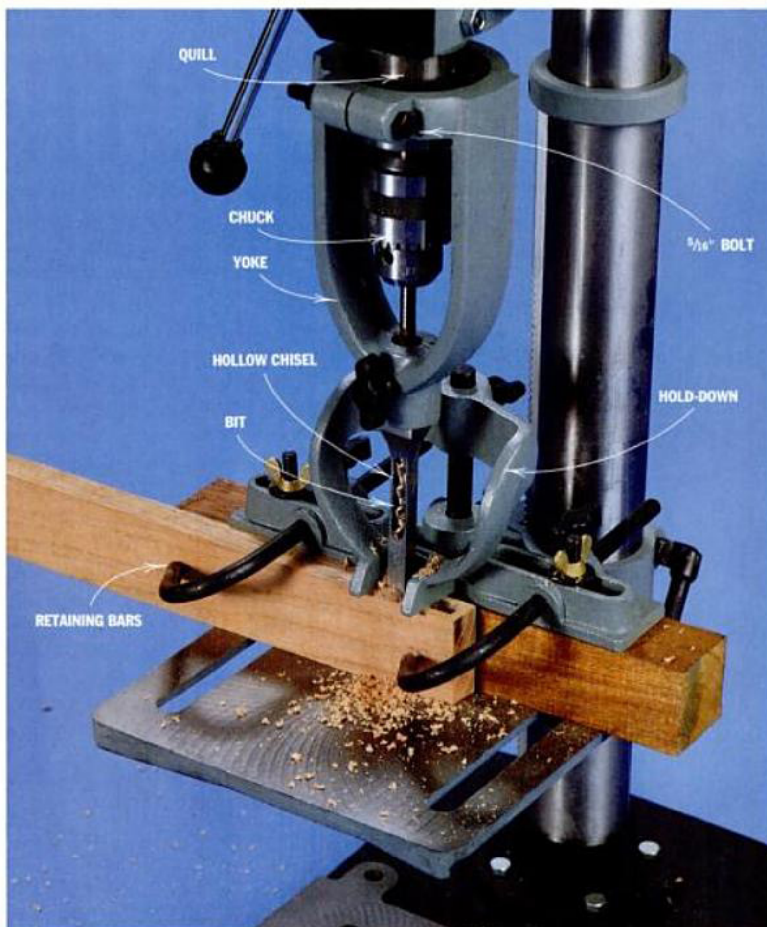
This 14-in. drill press is fitted with a conventional hollow-chisel mortising attachment.
