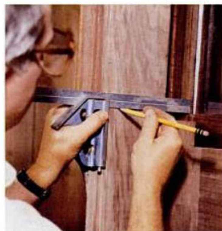
To locate the bottom edge of the dial, align a square with the top edge of the dial frame's bottom rail and draw a pencil line across the waist side. The dial's bottom edge must be \frac{1}{8} in. below this line.
