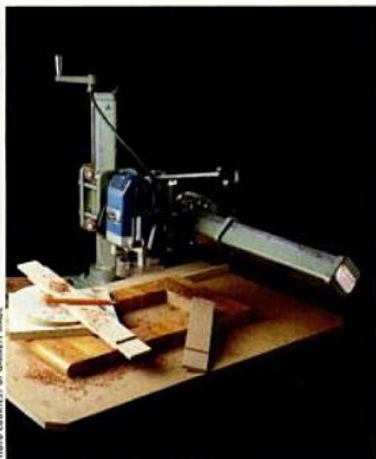
▲ The RouterMaster is a sturdy mounting carriage for a heavy-duty router.
