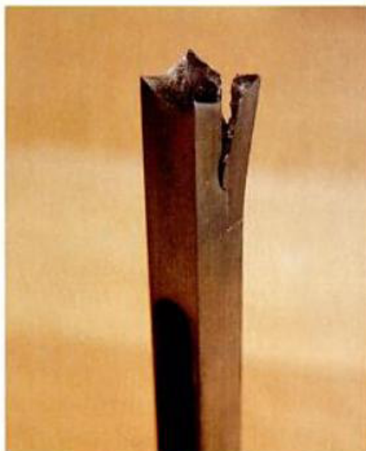
This hollow chisel split when the rotating bit was pulled up inside the chisel as the chisel was being withdrawn from the wood.
