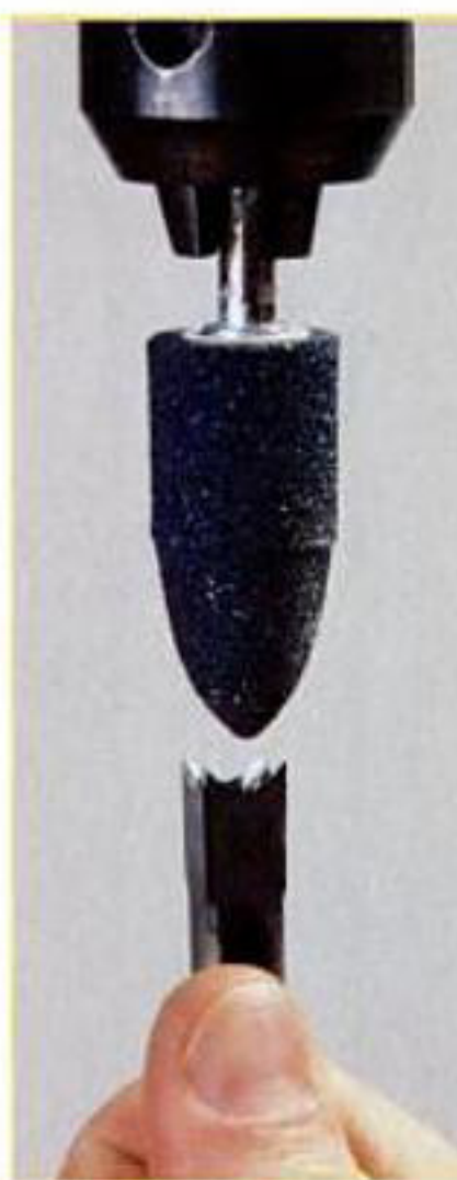
▲ To sharpen a hollow chisel, hold the end up against a cone-shaped stone until you feel a burr on the outside edges.
