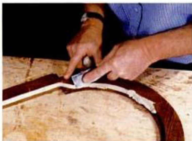
The door glass fits into a \frac{3}{8} -in. rabbet and is held in place with glazier's points and putty.
