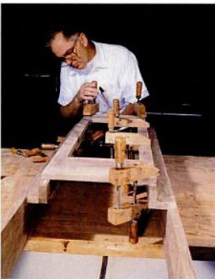
The waist frame is glued to the other waist parts with butt joints. Extra-long waist sides will be trimmed to length after the bonnet is complete.
