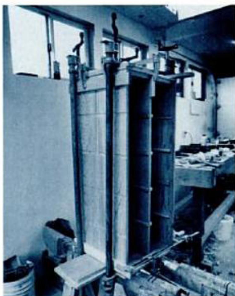
After making all the parts for the main tower and attaching the cleats for the floor panels, apply glue and assemble, as shown here.
