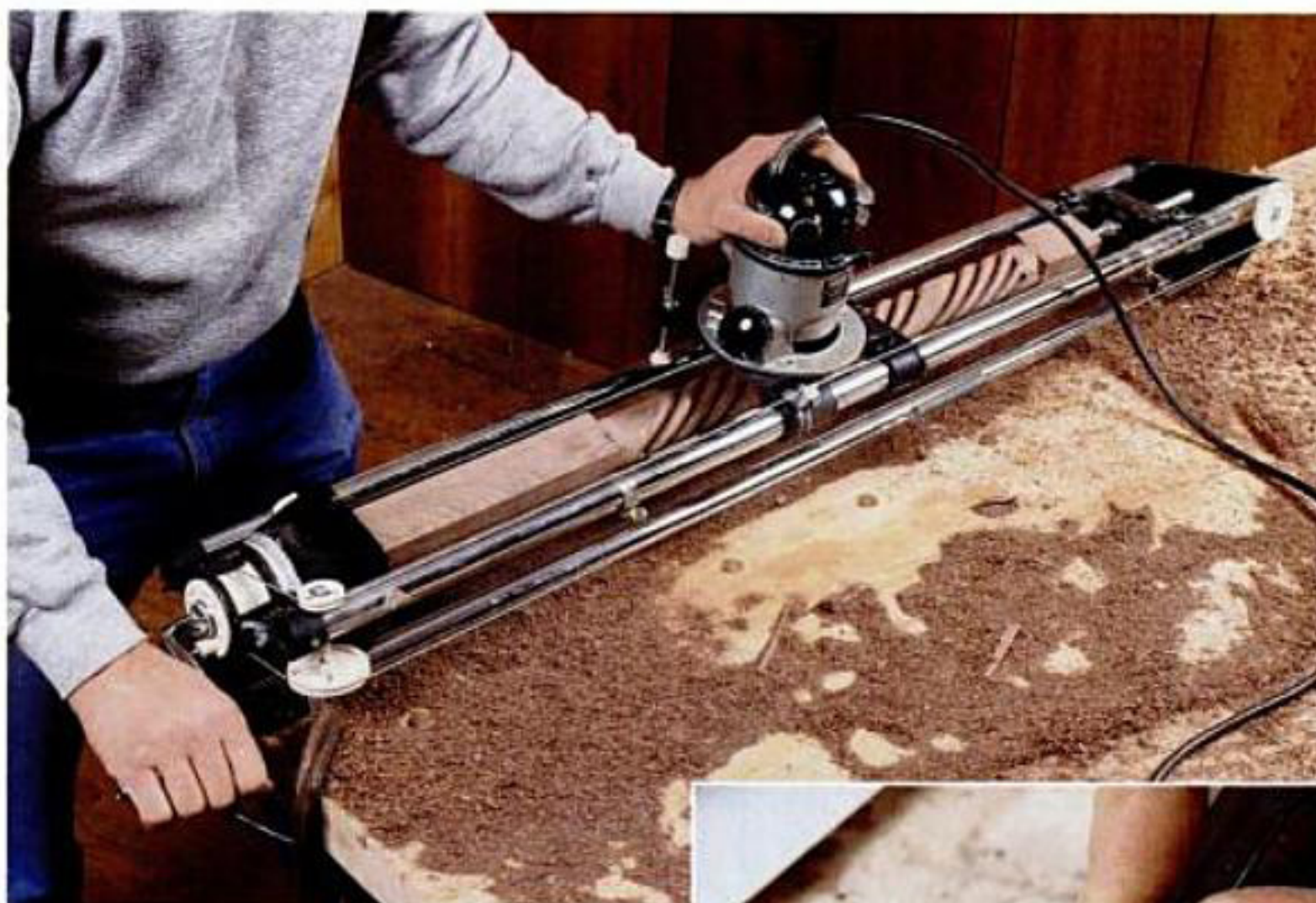
Author cut the spirals on the columns with a Craftsman Router Crafter. The spirals on the columns turn in opposite directions.
