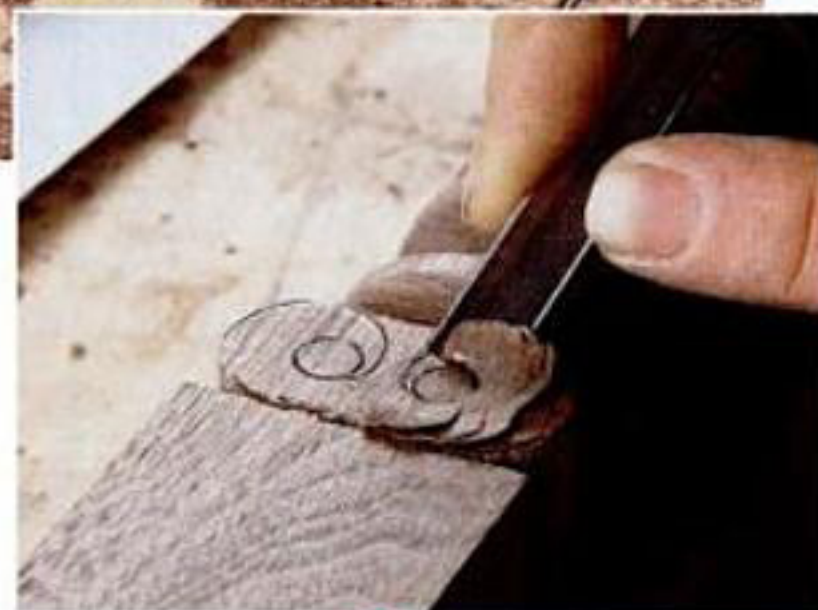
Author carves the scrolls at the top of a column with a gouge. He outlines the scroll with a vertical cut, then dishes out the scroll.
