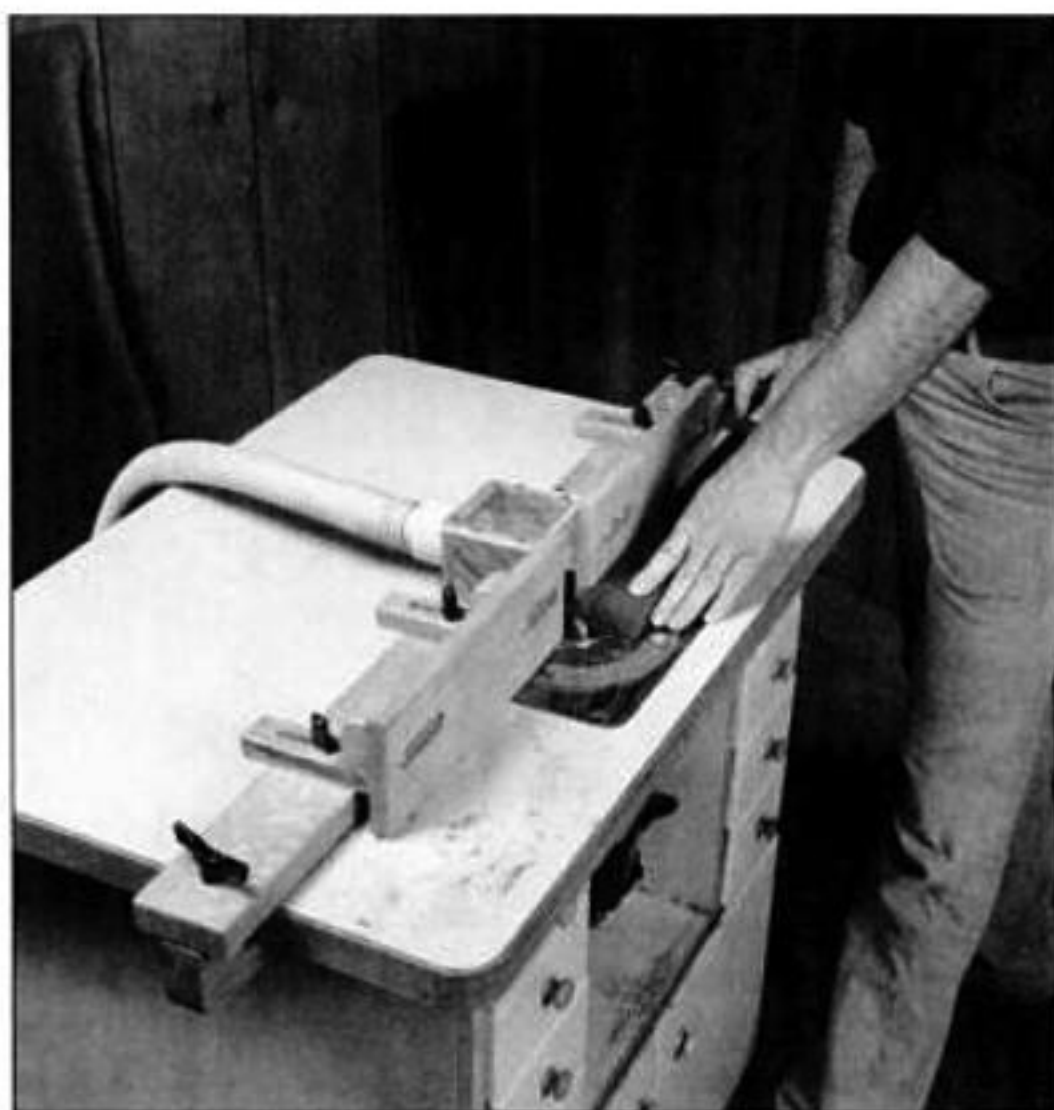
For shaping the edge of long pieces, rout with auxiliary fences in place. Fasten the small dust-collector box to the right-side fence with a screw.
