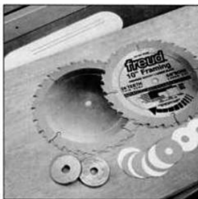
Two blades with accurately machined spacers between them cut the most accurate tenon cheeks.
