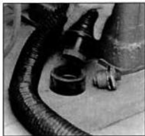
Richard Schneider's turned wooden plugs make effective blast gates for open-ended collection ducts.
