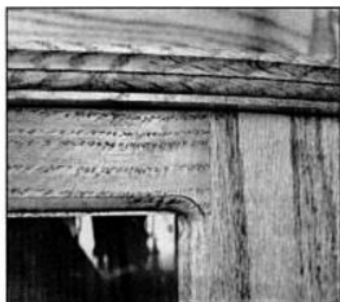
Rout the glass opening of the frames with a decorative \frac{1}{4} -in. beading bit and the outer edges of the top and bottom with a "classic" router bit.
