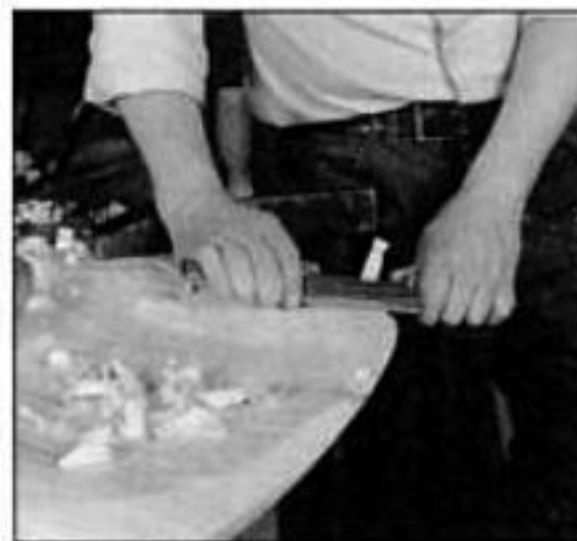
Blend the contour of the seat's edge into the dished saddle with a spokeshave. Complete the final shaping with a curved-sole compass plane or travisher.
