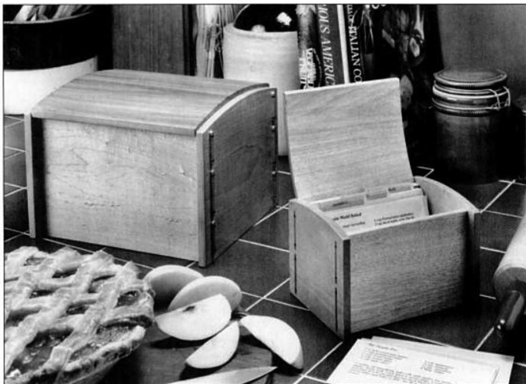
Wedged mortise-and-tenon joints decorate the sides of these curved-top recipe boxes.
