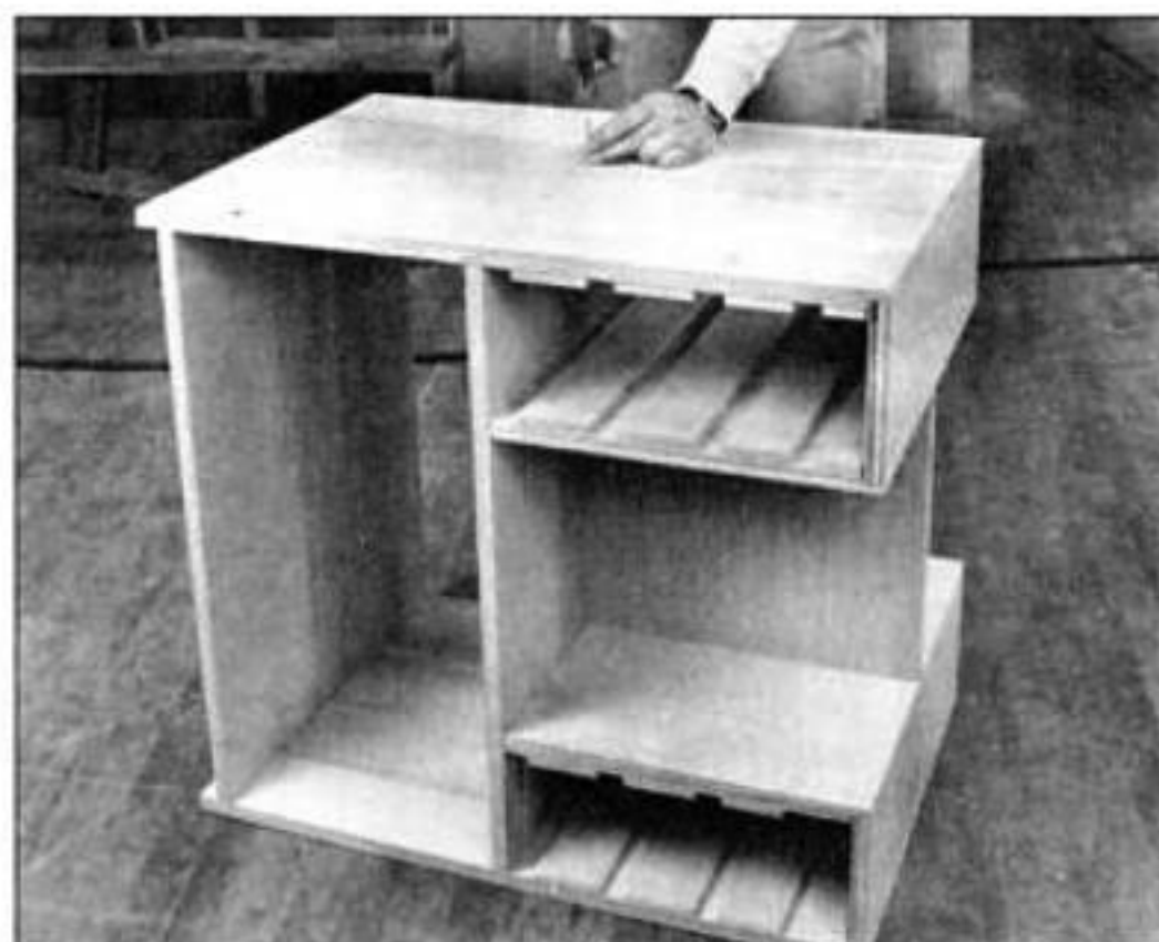
The birch-plywood cabinet is joined with dadoes and butt joints.
