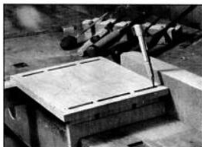
Mark out the rounded shape of the tenons by tracing through the mortises onto the tenon ends.
