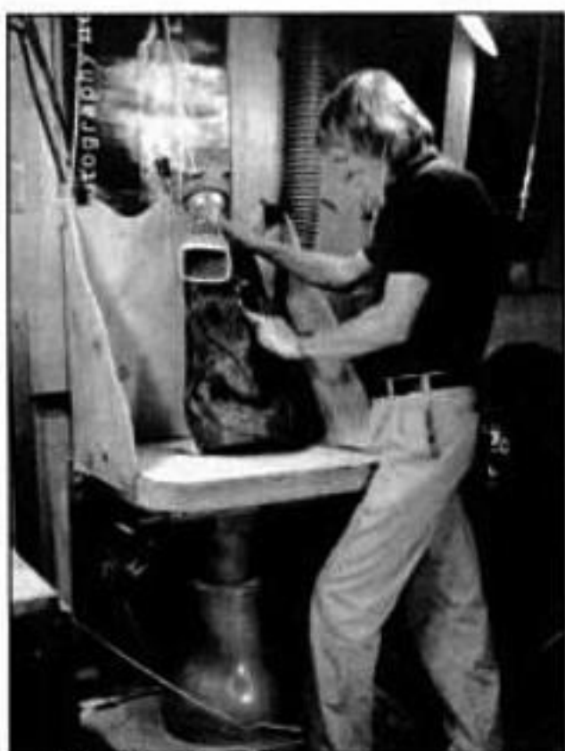
Sculptor Paul Perras maneuvers the sheet-metal nozzle of his carving-station dust collector into place.
