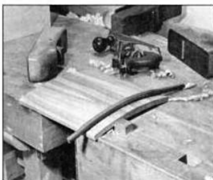
After bandsawing the lid's curve, hand plane it even. A flexible curve comes in handy when doing this.
