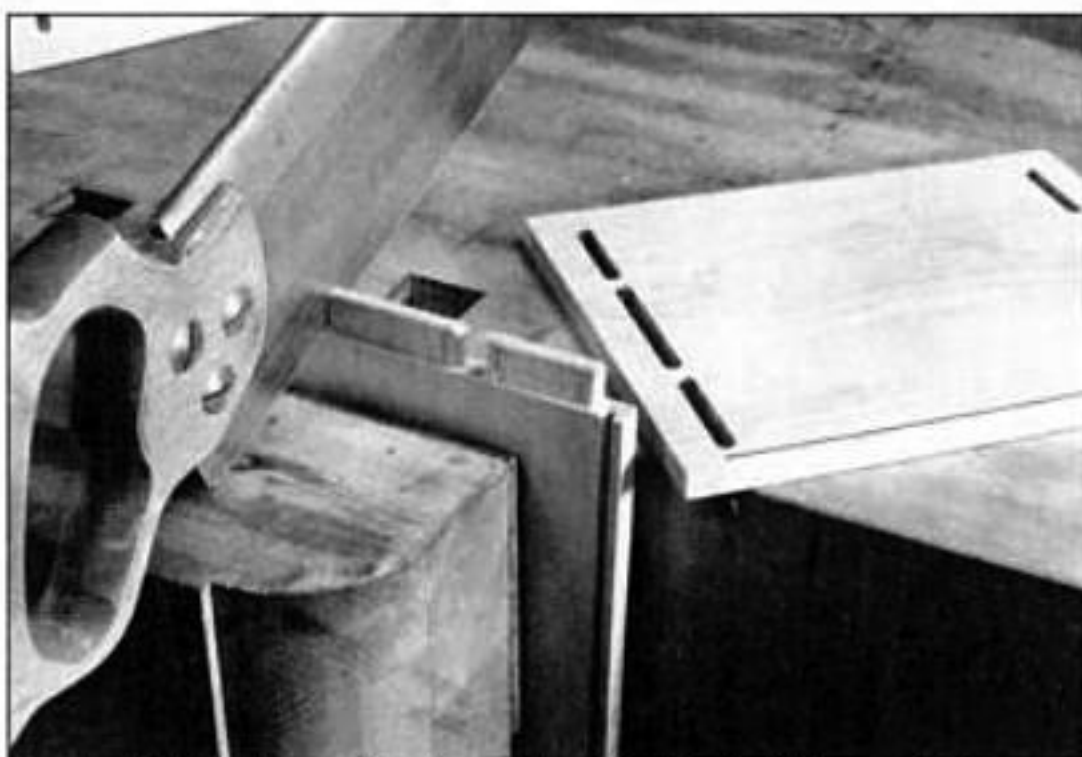
Saw kerfs in the tenons for the wedges. Don't cut all the way to the shoulder. Leave about \frac{1}{16} in. at the bottom of the tenon.
