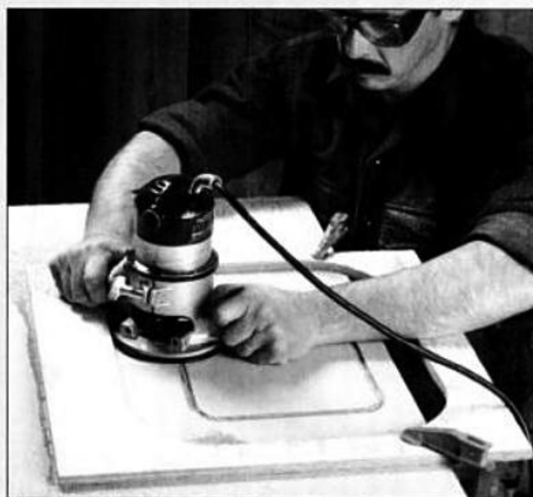
Shape the rectangular cutout in the top by routing a groove along a router template sized from the new plastic base plate.
