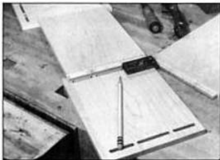
After sawing the tenon cheeks on the box front and back, mark the lengths of the tenons with a straightedge and pencil.
