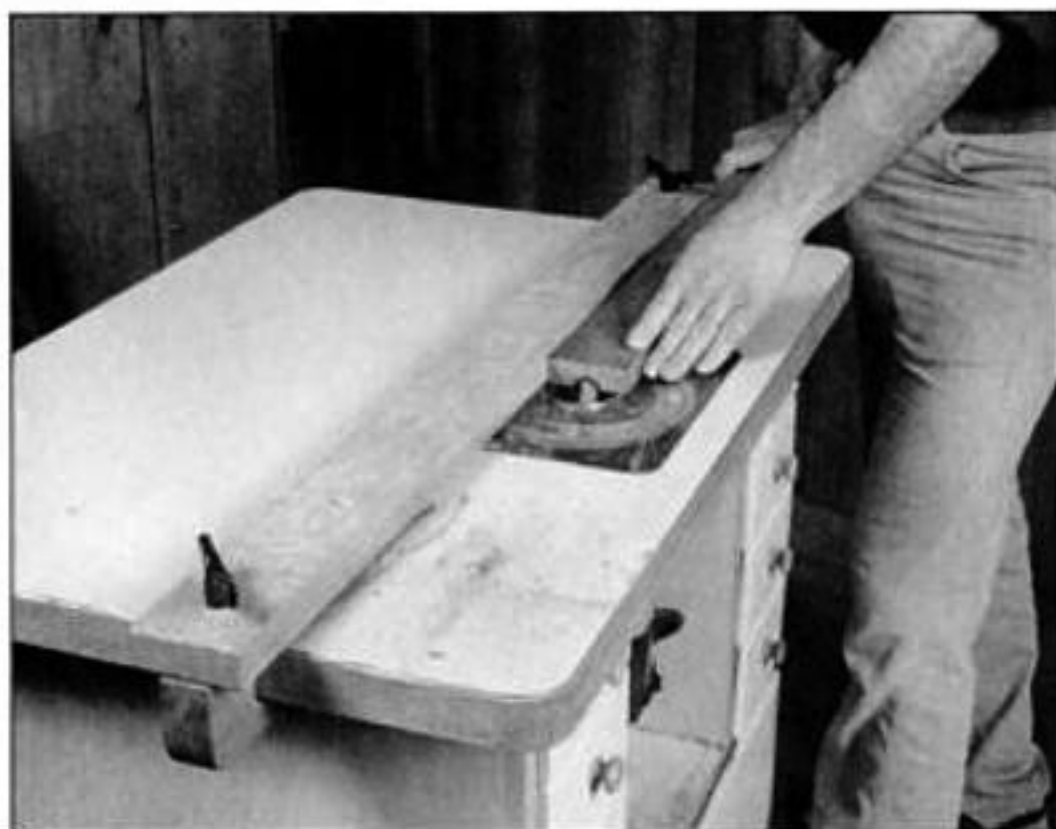
To rout grooves, dados and coves use the main fence alone.
