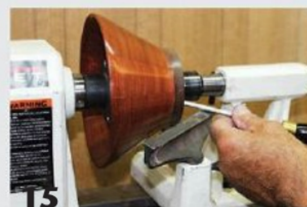
Turn your tapered-stave bowl. Foam tape is wrapped around the remains of the base and waste block to form a jam chuck for completing the bottom.
