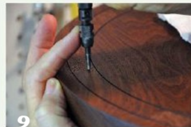
9 I often decorate the seat top with a defined, textured area. I use a flex-shaft tool with a hammering handpiece to create the texture.
