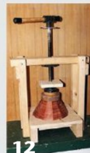
Sand the bottom smooth and flat prior to gluing on the base. I use a shopmade fixture to apply pressure, but an F clamp with a deep enough throat would also work.
