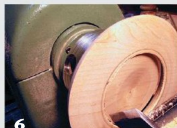
The piece is reverse-mounted so the rounded half-torus is facing the headstock, and what will be the inside gluing surface can be reduced to the desired radius ( \frac{5}{8} " in this case). This face must be dead flat, verified with a straightedge, to ensure a good glue joint. I then parted the half-torus ring from the center material.
