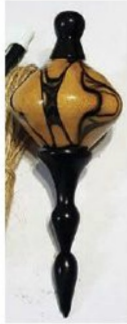
For further refinement, this hollow ornament body was remounted on a pen mandrel with soft duck-call bushings.
