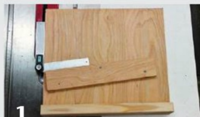
1 The author's shopmade table saw sled for cutting tapered staves, set for a miter angle of 7.6°. Since the digital protractor is aligned with the left edge of the sled, its angle is set to the complement of the miter angle: 90^\circ - 7.6^\circ = 82.4^\circ .
