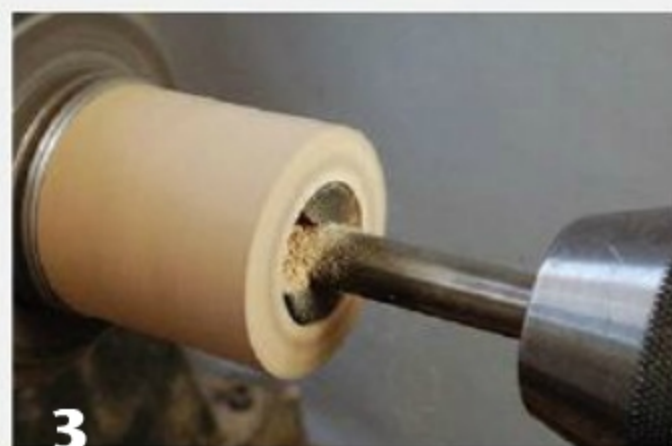
The lid section is held in the chuck for hollowing with a Forstner bit. The interior of the lid is then refined with a scraper.
