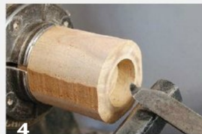
The lid section is held in the chuck for hollowing with a Forstner bit. The interior of the lid is then refined with a scraper.
