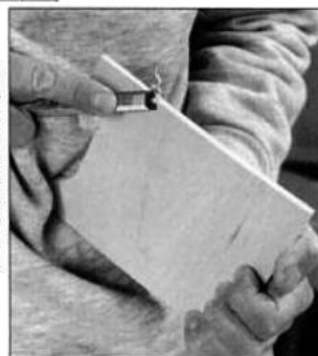
Chamfer the top and bottom edges of the letter-box dividers for an easier fit in the shelf dadoes. Note that the grain runs parallel to the shorter dimension of the divider.
