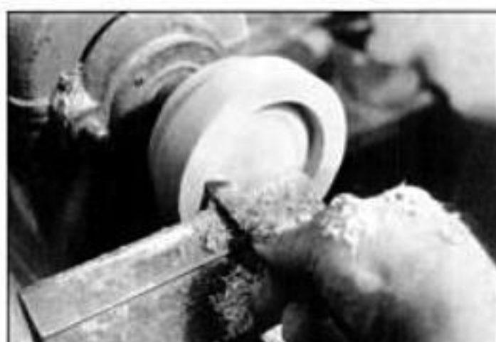
Cut the sides of the mirror recess straight and flat with a skew chisel in scraping position
