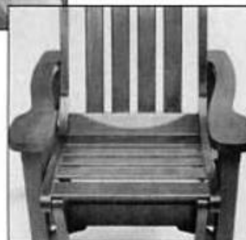
Tilting the bandsaw table and sawing a curve on the edge of the stock (above) produces the subtle arch in the lower rail of a chair (right).
