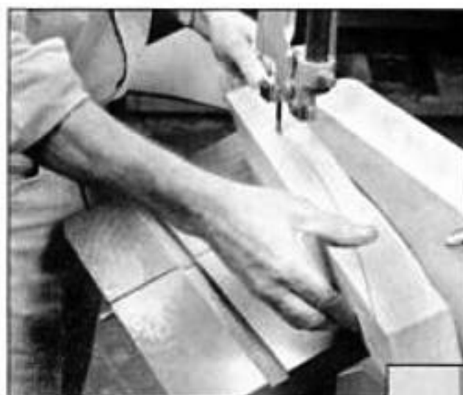
Tilting the bandsaw table and sawing a curve on the edge of the stock (above) produces the subtle arch in the lower rail of a chair (right).
