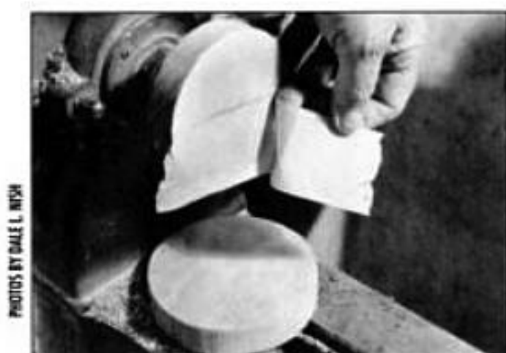
Fasten the lid piece to the waste block with glue or double-sided tape (shown here).
