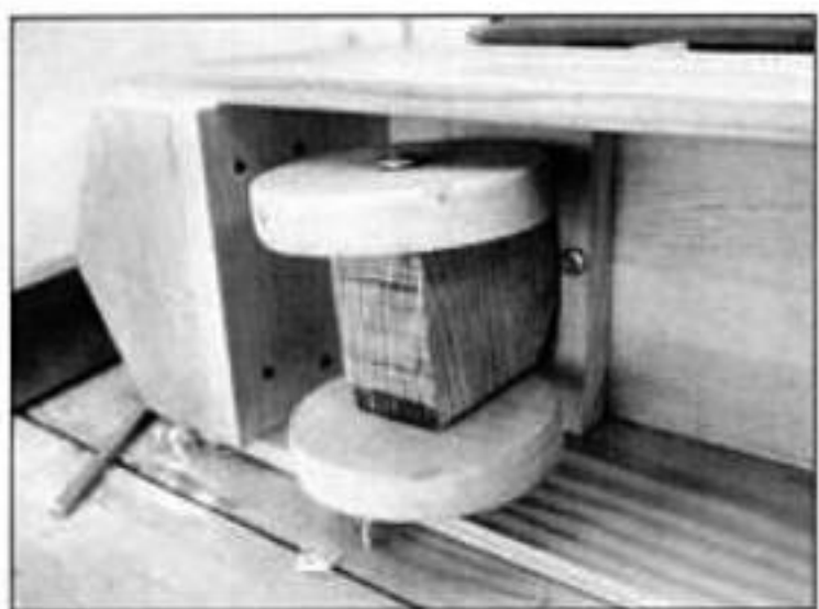
Glue the boiler block to the cab front, boiler support block and locomotive sides (above). Reinforce the glue joint between the cab front and the boiler block with finish nails.
