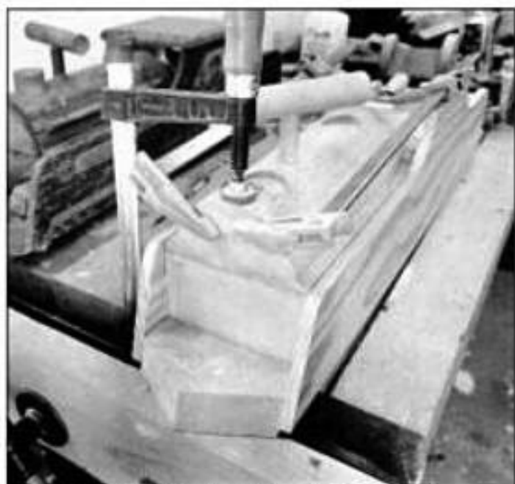
Glue the boiler block to the cab front, boiler support block and locomotive sides (above). Reinforce the glue joint between the cab front and the boiler block with finish nails.
