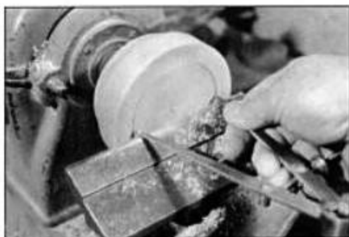
To mark the mirror recess, set a pair of dividers to the diameter of the mirror. Center the dividers on the spinning lid and push the downhill point of the dividers into the lid.
