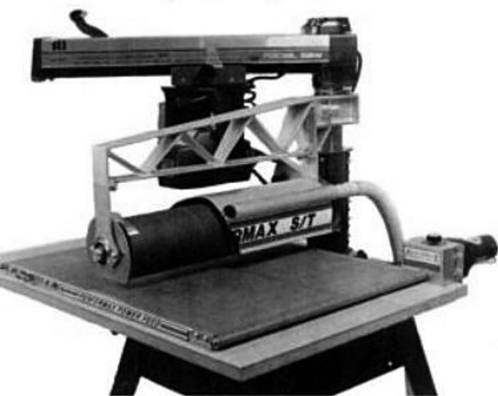
The Performax ST is the least expensive way to get drum-sanding capability in your shop. The sander mounts on a radial arm saw column and uses the saw's motor for power. This setup also shows the optional Performax power feed accessory.
