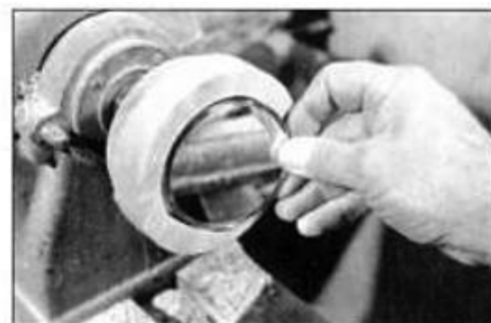
Check the fit of the mirror in the recess. The recess should be about \frac{1}{16} in. larger in diameter than the mirror.
