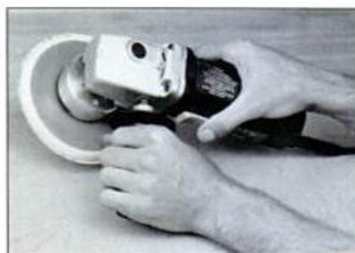
Most right-angle random-orbit sanders come with side handles (AEG VSR 600 shown). These sanders convert to angle grinders by mounting a grinding wheel and guard in place of the sanding head.
