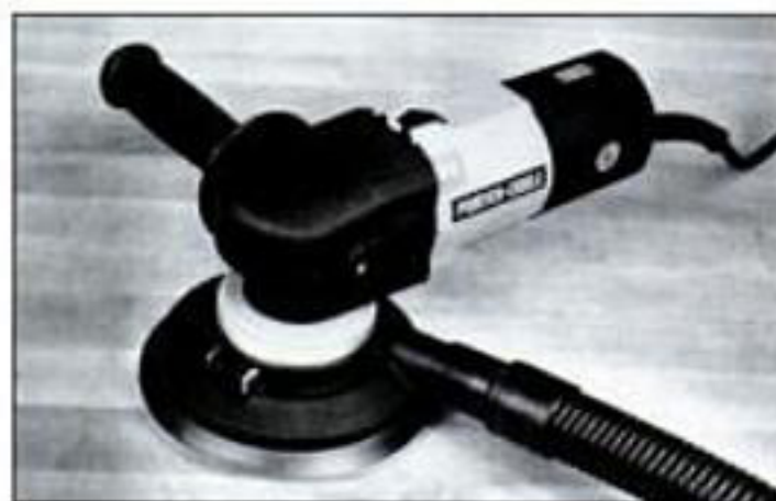
Optional dust-pickup hood on the Porter-Cable sander does a good job of dust collecting when connected to a standard shop vac.
