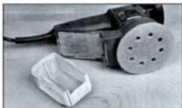
Detachable dust box on Ryobi fits neatly under the rear handle. The box slips on and off easily, but fills up with dust faster than bags do.
