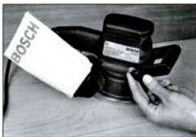
The front bail-type handle on Bosch 3283 DVS adjusts to different positions, though it's a bit small for large hands to grip comfortably.
