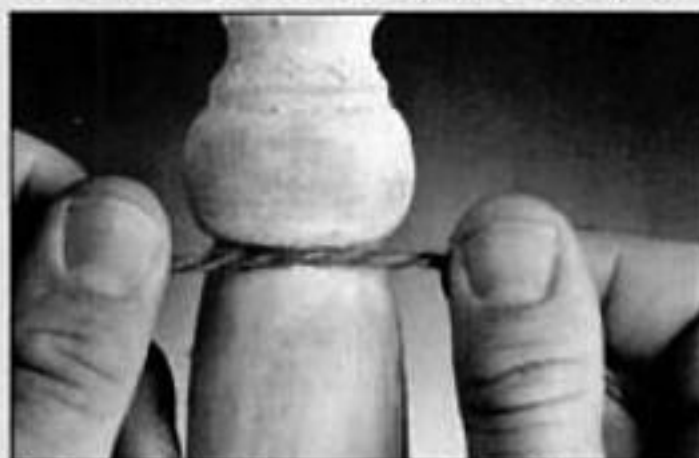
Pull a coarse string or rope around the recesses of turnings to work out blistered paint or finish.
