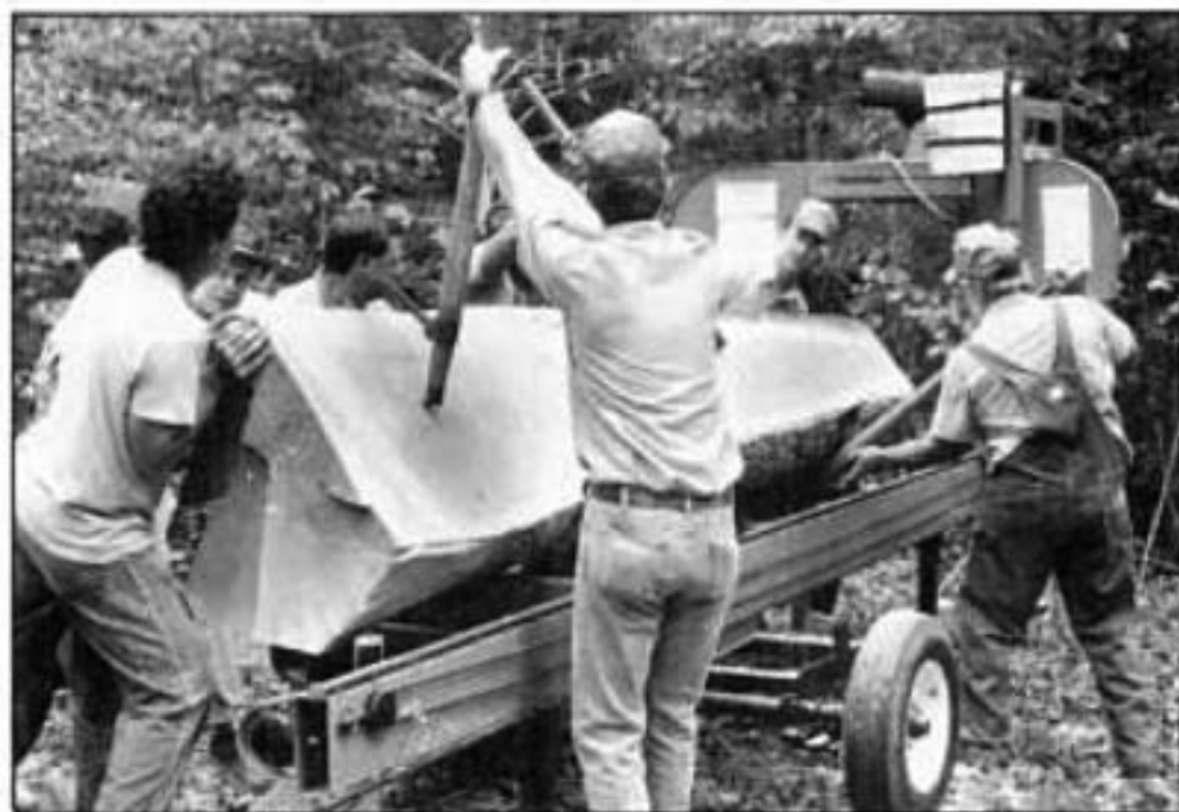
Turning a 28-in. dia. oak log without hydraulic log-handling equipment is not a one-man operation.
