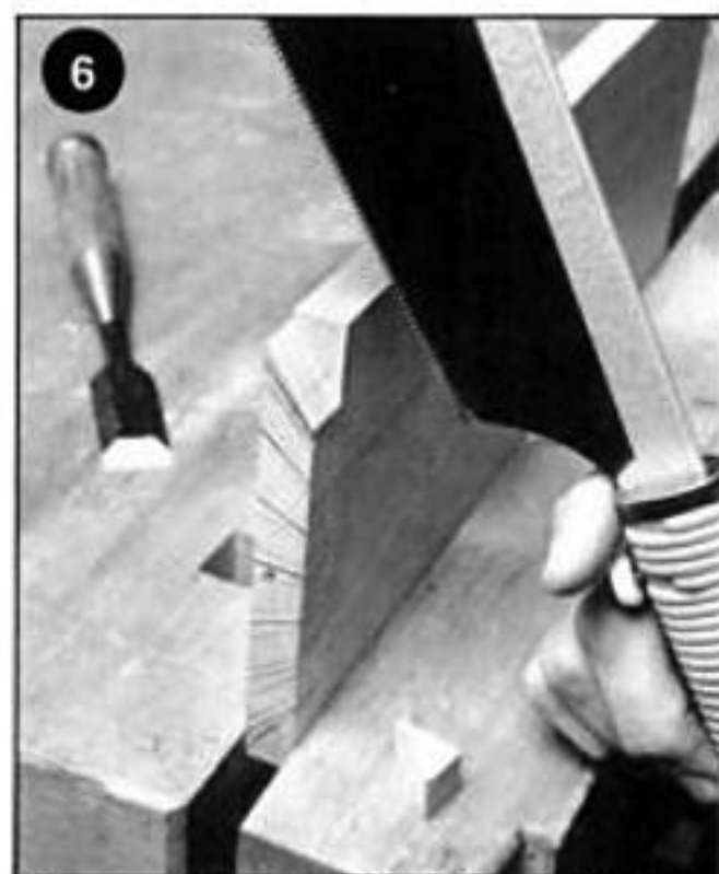
6.) Saw on the waste side of the scribed line (very carefully)!
