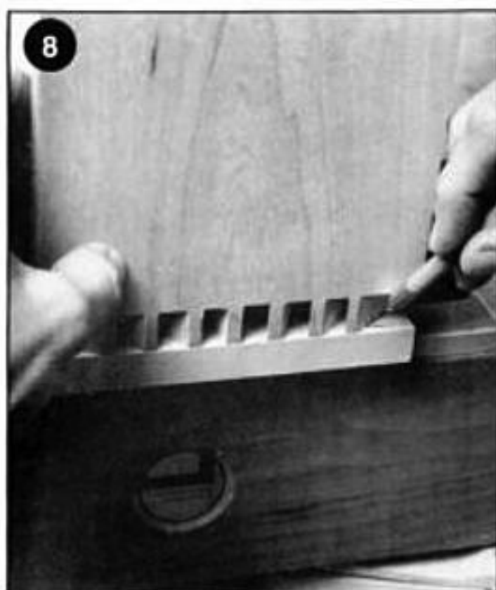
8.) With a very sharp pencil, trace the outline of the pins onto the other board.
