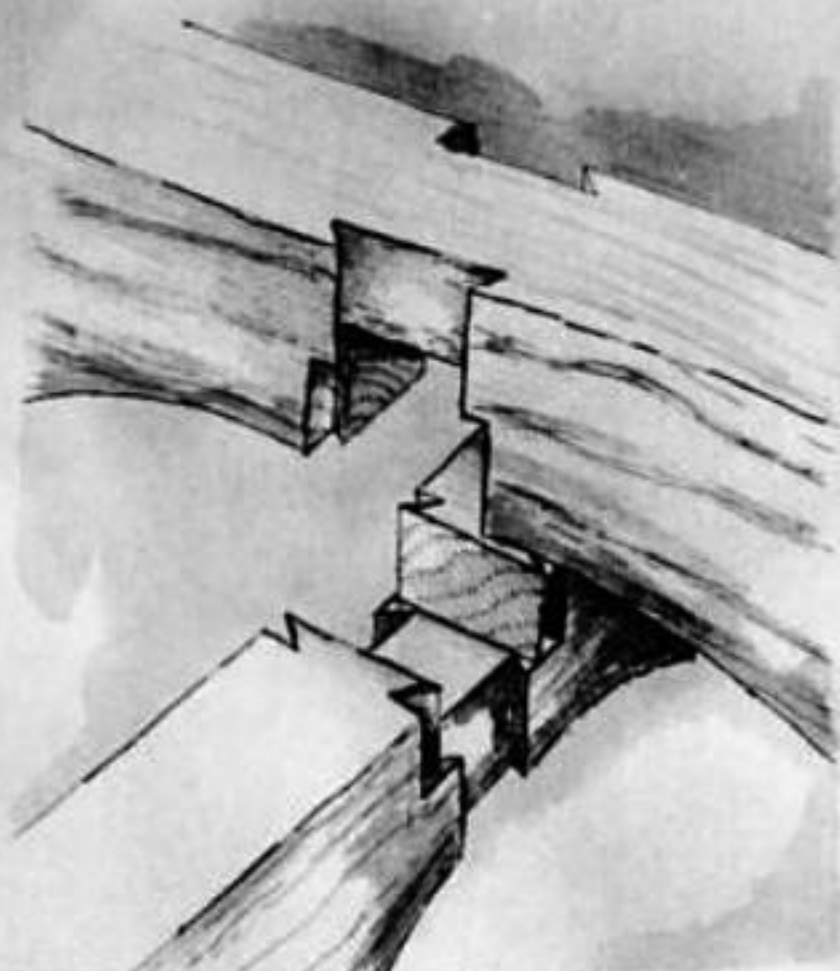
DOUBLE-DOVETAIL HALF LAP STRENGTHENS THE HALF LAP AGAINST TWIST AND INCREASES GLUE SURFACE.
