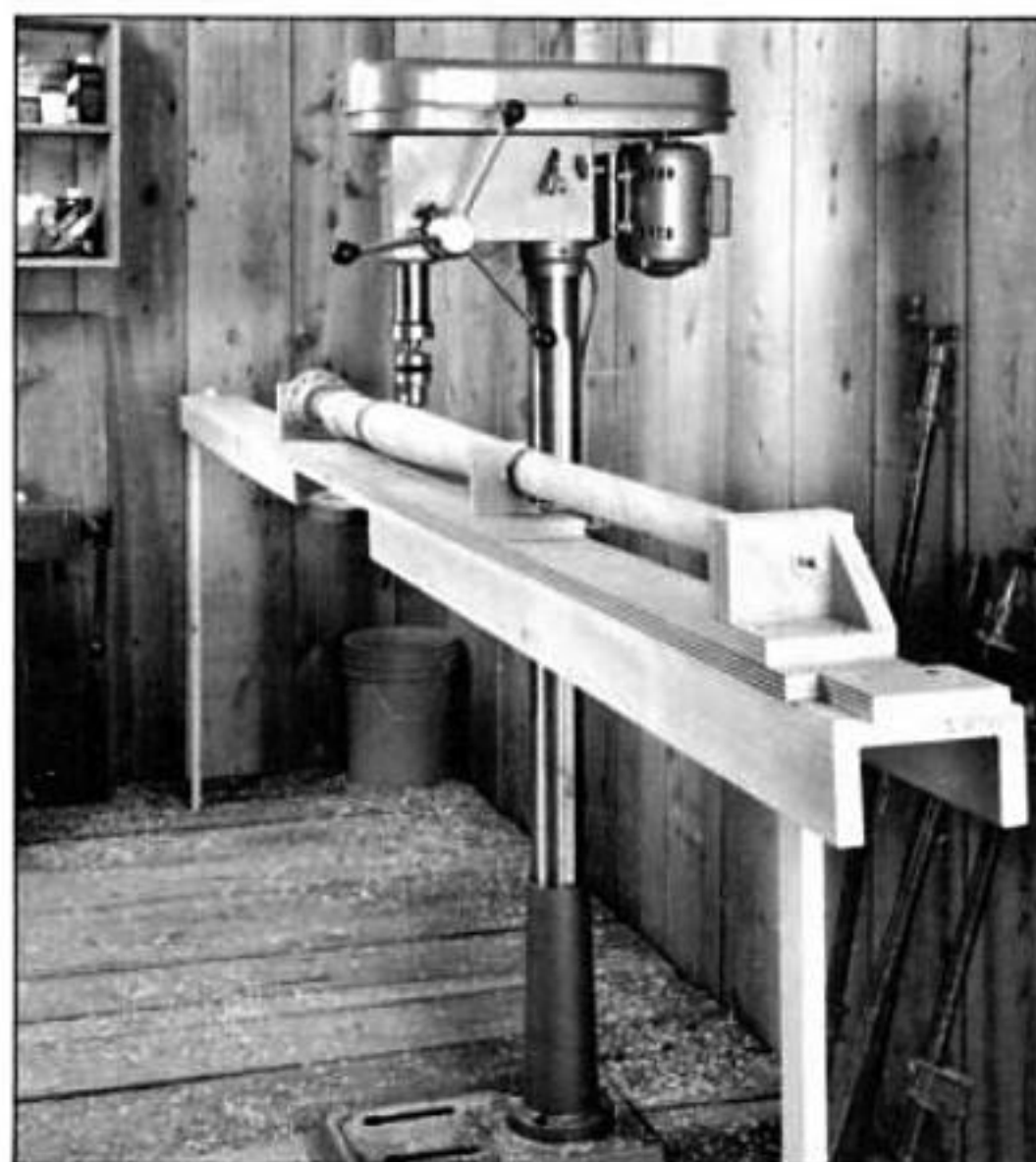
A temporary table extends the drill-press table to support the sliding jig.
