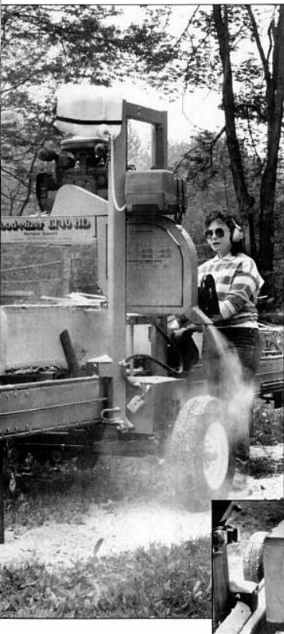
Mobile bandsaw mills slice boards off the top of the log. To get edged boards, square the log before sawing it up.
