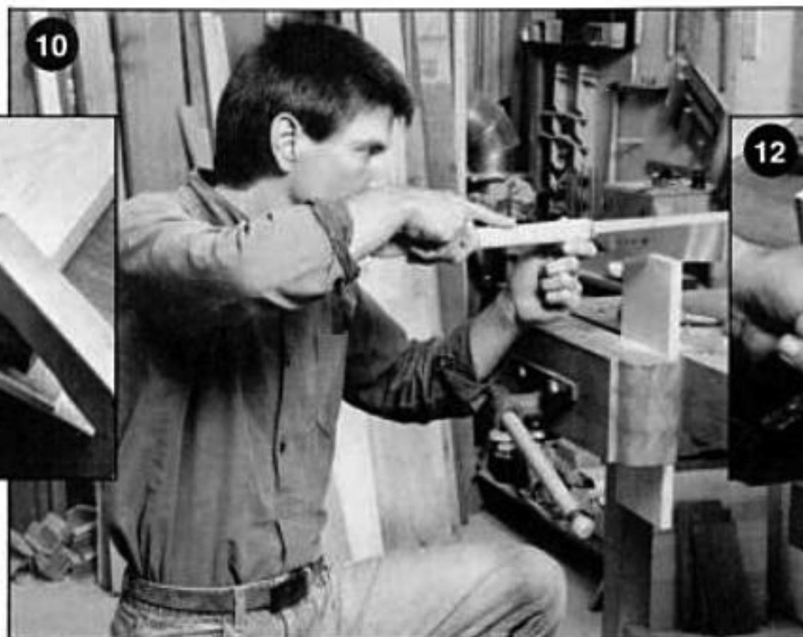
10.) Here's where ultimate care pays off. Saw the waste exactly to the line. Kneel down so you can see what you're doing, and say a little prayer to the spirit of dovetails. (It couldn't hurt.)
