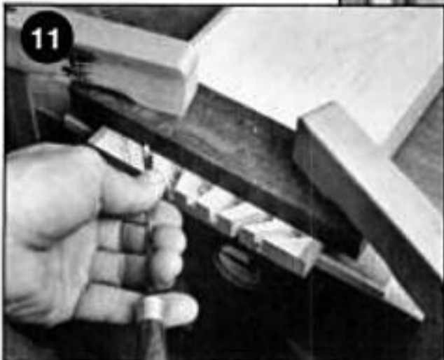
11.) Again, chop out the waste from both sides. This is where a really narrow chisel comes in handy.
