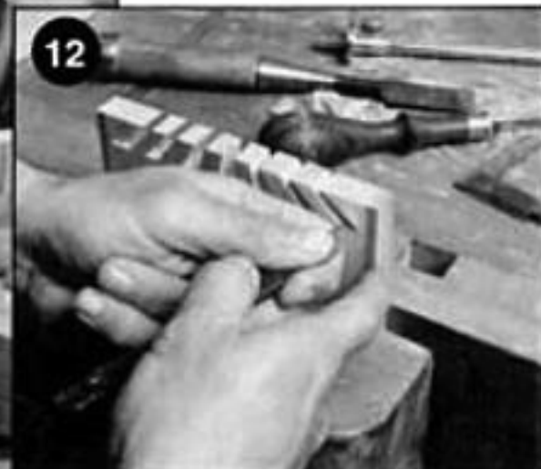
12.) Clean up the tight corners with a knife, and fit the joint together.
