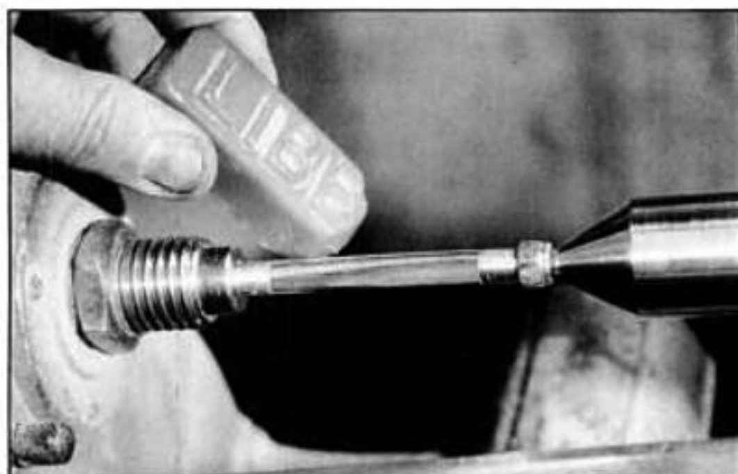
A light coat of carnauba wax from a wax stick puts the final touches on a finish of lacquer or padding lacquer.
