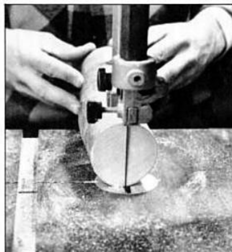
The best spoons start with a slightly curved branch. Begin by splitting the branch down the pith with an ax or on the bandsaw.
