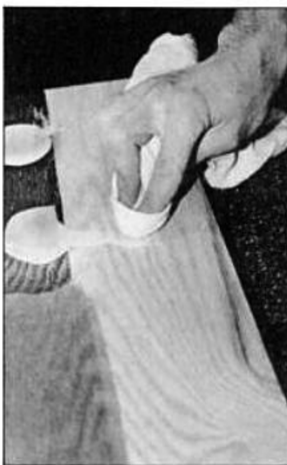
Sanding is the key to a perfect finish. Sand the sealer coat with 220-grit no-fill paper wrapped around a felt block or a blackboard eraser. Here, Camp sands a sample board on which he's applied finish over several different stains.
