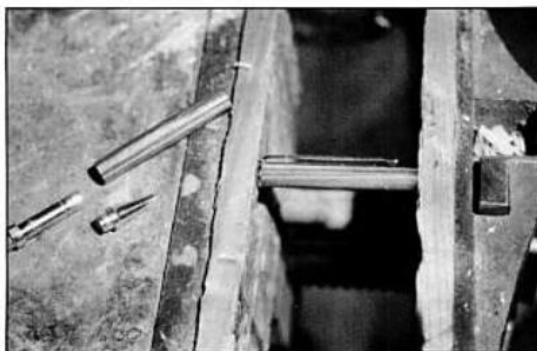
Press the pocket clip and end-cap assembly firmly into the end of the barrel with a vise.
