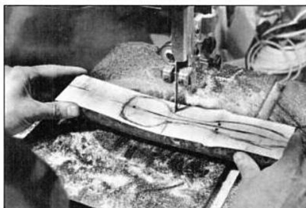
Before bandsawing the spoon outline, make a couple of relief cuts where the bowl meets the handle.
