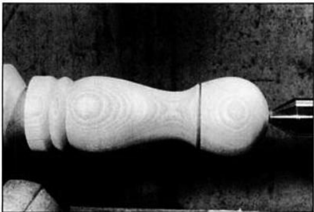
Turn the top of the mill to shape, and finish up any shaping of the body.
