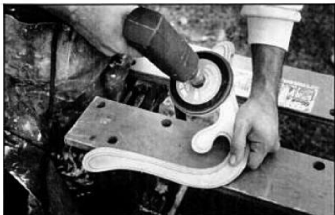
A disc-sanding attachment on your drill is good to rough out the airfoil shape on the wings of the boomerang.
