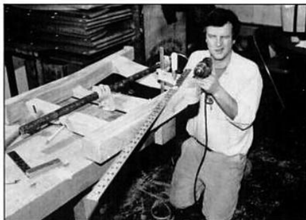
To drill the bolt hole in the bench's end assembly, aim a long bit carefully down a sight line at the center of the nut hole. Extend the sight line with a steel ruler if it helps you to aim accurately.
