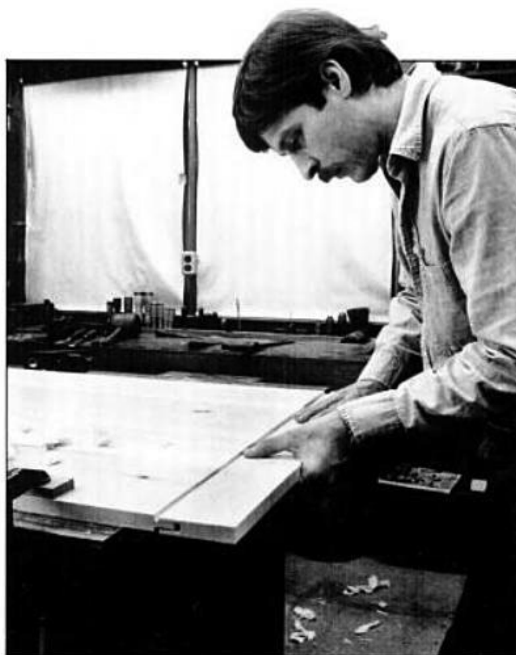
Glue the breadboard ends to the top at their center only. Peg the ends 6 in. on either side of the centerline for reinforcement.
