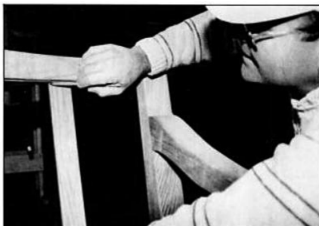
Mark the backrest slats for length by fitting them in their mortises at one end and marking the other end while the bench is temporarily assembled.
