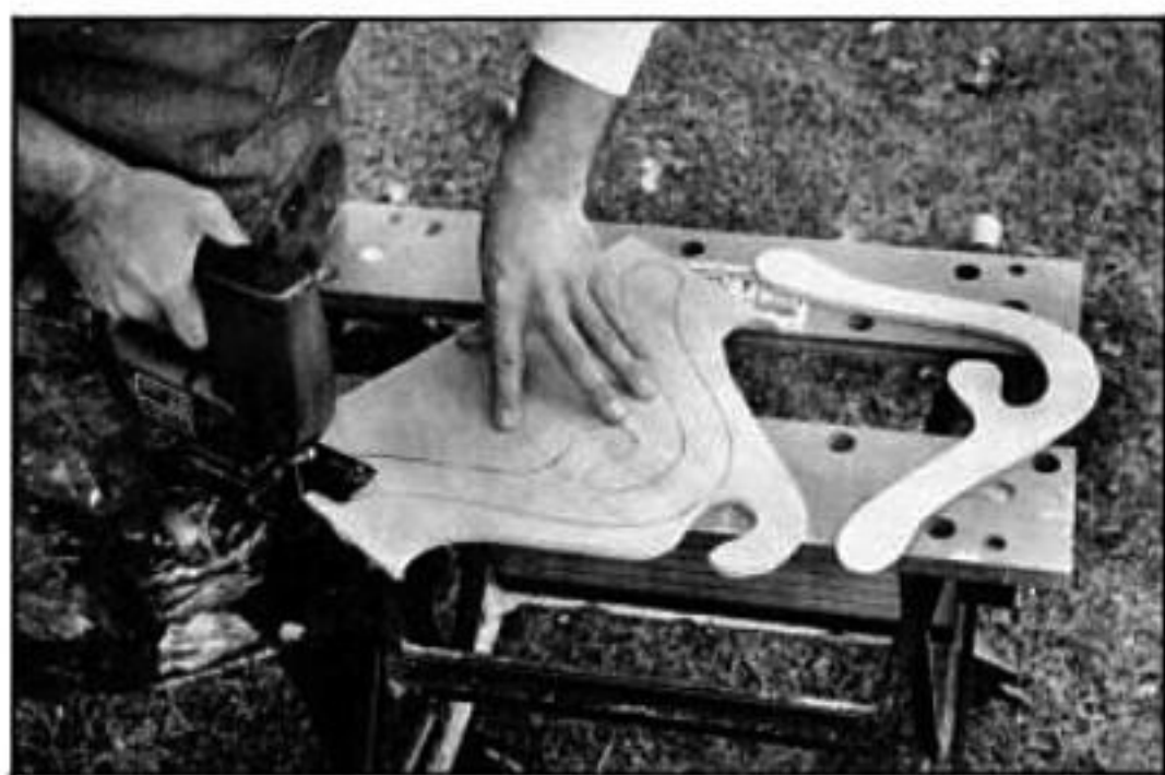
Draw the pattern of a boomerang on a sheet of thin plywood and cut out the blank with a saber saw.
