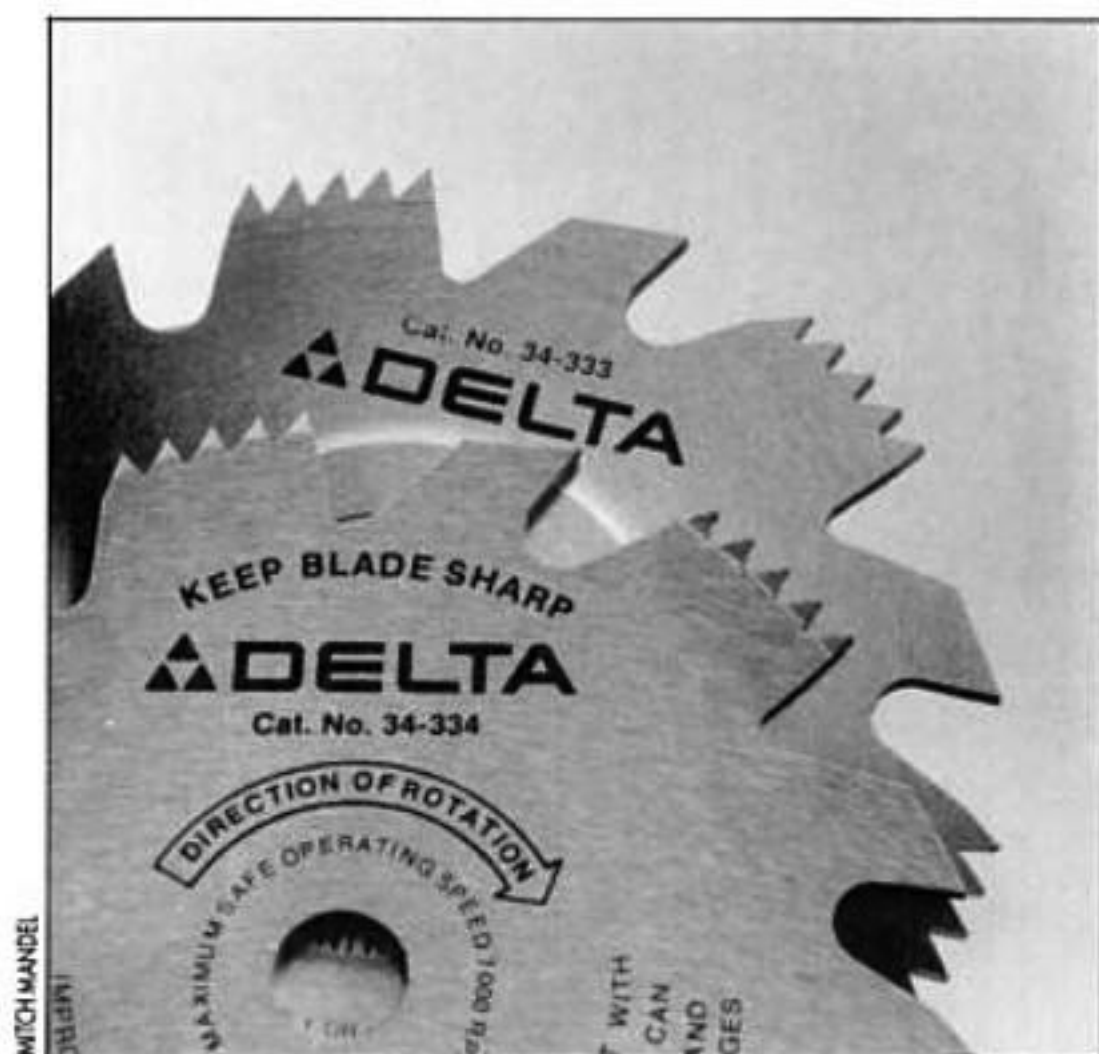
Less expensive 6-in. all-steel stack dados offer a choice of economy machine-set teeth (front) or higher-quality hollow-ground blades (rear). Delta dado sets shown.
