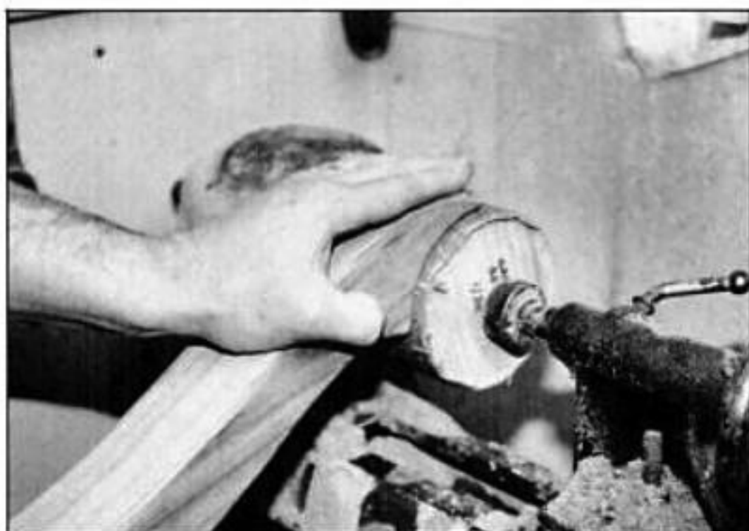
A turned wooden sanding drum covered with 80X abrasive paper or cloth grinds the front end of the bench arm to match the diameter of the balls.
