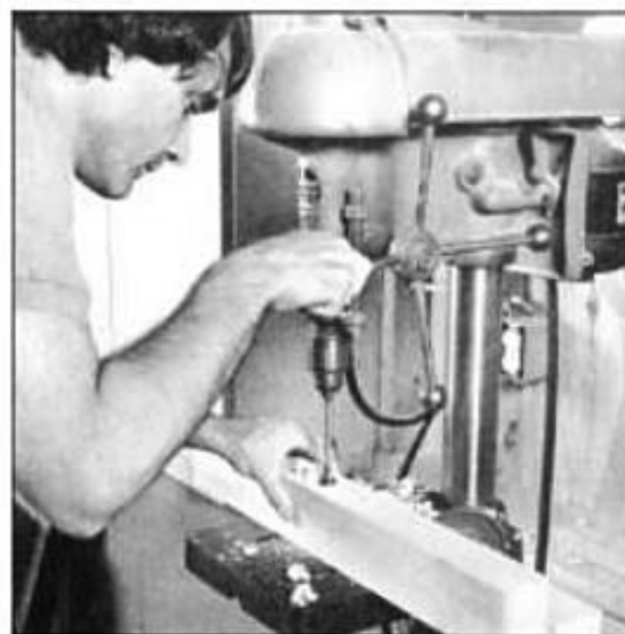
4. Remove the mortise waste on the drill press. Drill from both sides for a clean mortise.
