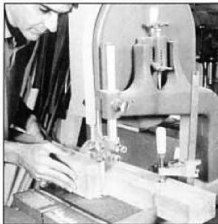
6. Cut the cheeks of the tenon on the bandsaw. Keep one working face of the stock against the fence and adjust the fence for the second cut.
