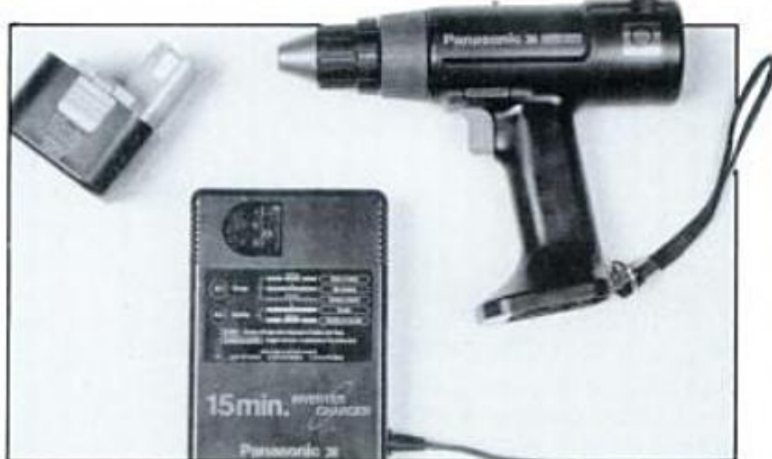
The Panasonic battery charger is one of the most sophisticated on the market: one LED indicates charging, another indicates if the battery is too hot to charge (standby) or if there's a malfunction in the battery or charger.
