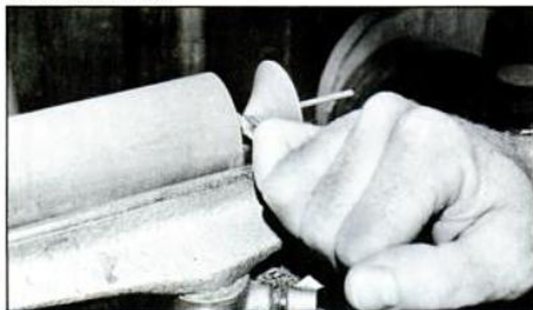
Carefully cut away the remainder of the hollow and then cut the top off with the tip of the gouge.
