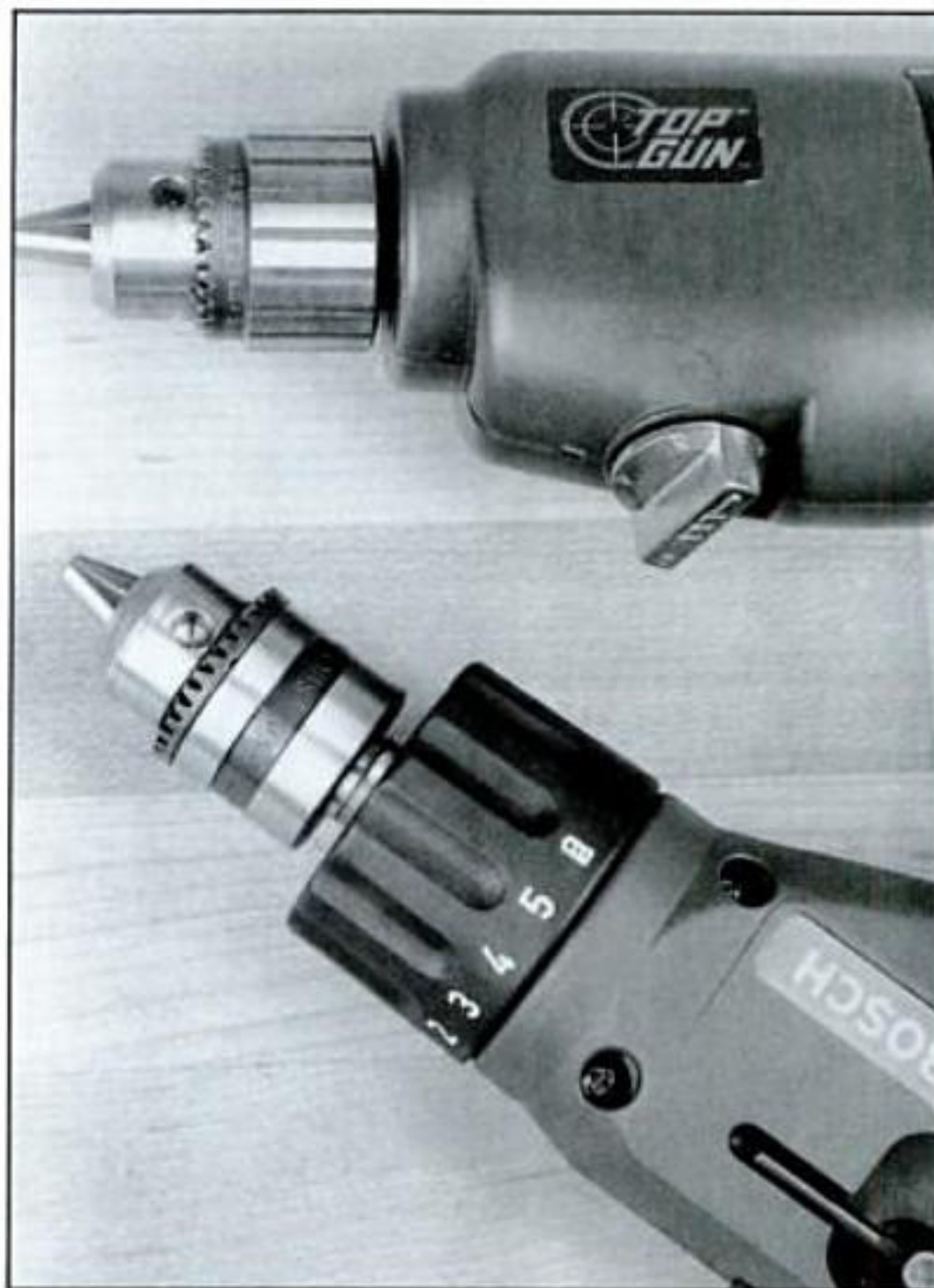
Collars (left) or knobs (right) adjust the torque limit of clutches on drill-drivers. Numbers on the collar are easily visible in operating position.
