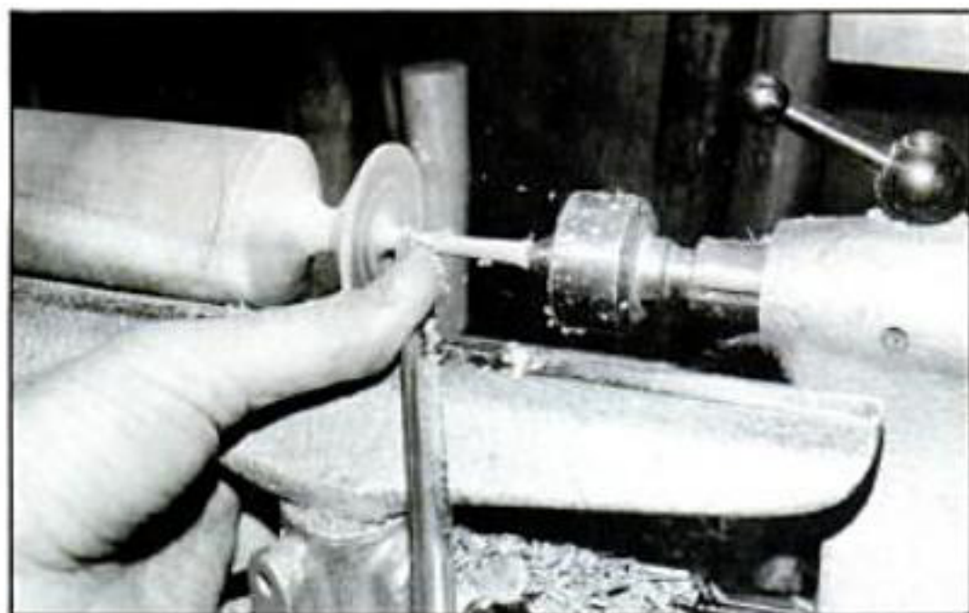
Turn the stem diameter as thin as possible with the gouge.
