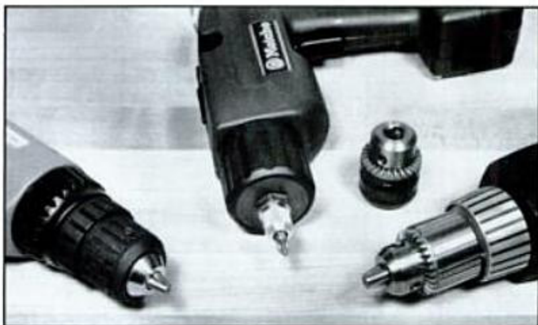
Three different chuck arrangements: keyless (Hitachi, left); a drill chuck that interchanges with a hex collet (Metabo, center); and a chuck that will hold the tiniest bit made (Porter Cable, right).
