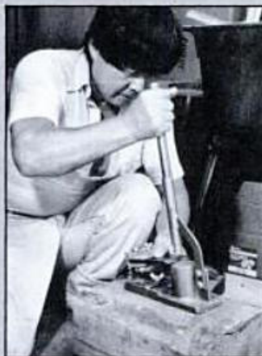
To re-create the flat spot on the back side of a plane blade, tap across the bevel with the corner of a hammer. The point of impact for each blow must line up with the corner of the block underneath.
