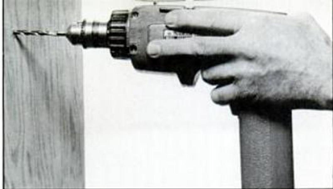
Good body design allows a comfortable in-line grip as an alternative to the conventional handle grip. Switching grips can reduce wrist fatigue and provide better control for fine work.
