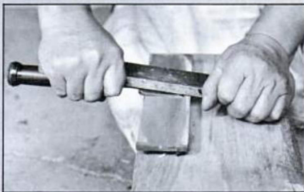
▲ ▼ You don't need to tap out the backs of chisels. Rub the back flat on the lapping plate with a little more pressure toward the edge. On narrow chisels, you only need to apply pressure with your fingers. Hold narrow chisels at an angle so they don't rock.
