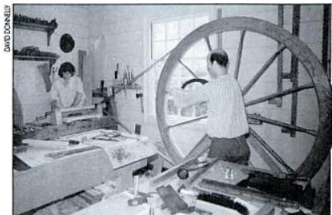
At Colonial Williamsburg's reconstructed Anthony Hay Cabinet Shop, an apprentice powers a great-wheel lathe, while master craftsman Mack Headley turns a spindle for an 18th-century reproduction.
