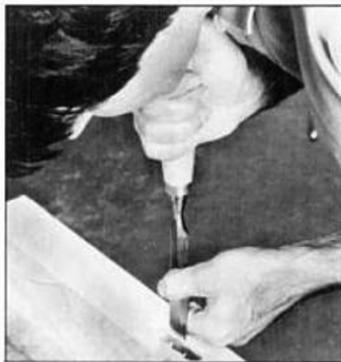
5. Once you've removed the major portion of the waste from the mortise on the drill press, pare the excess away with a chisel.
