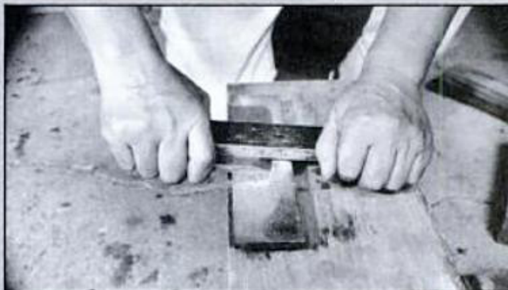
◀ When the flat spot is even, gather the carborundum paste in the center of the plate, add a few drops of water and continue rubbing as hard as you can until the plate is dry.
