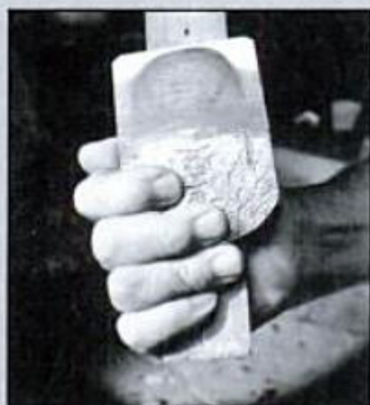
◀ The flat back of the blade should shine like a mirror when you wipe off the carborundum paste.
