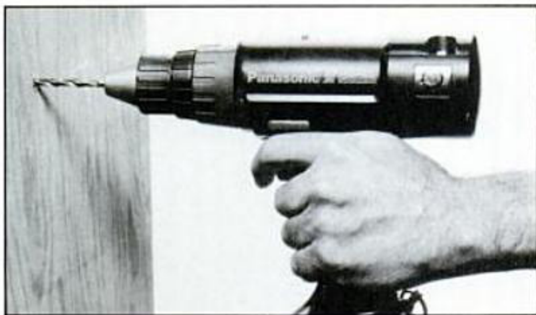
T-handle designs with the battery below the handle provide good balance and weight distribution. This Panasonic (the author's favorite) also has a convenient sliding forward-reverse switch above the trigger.
