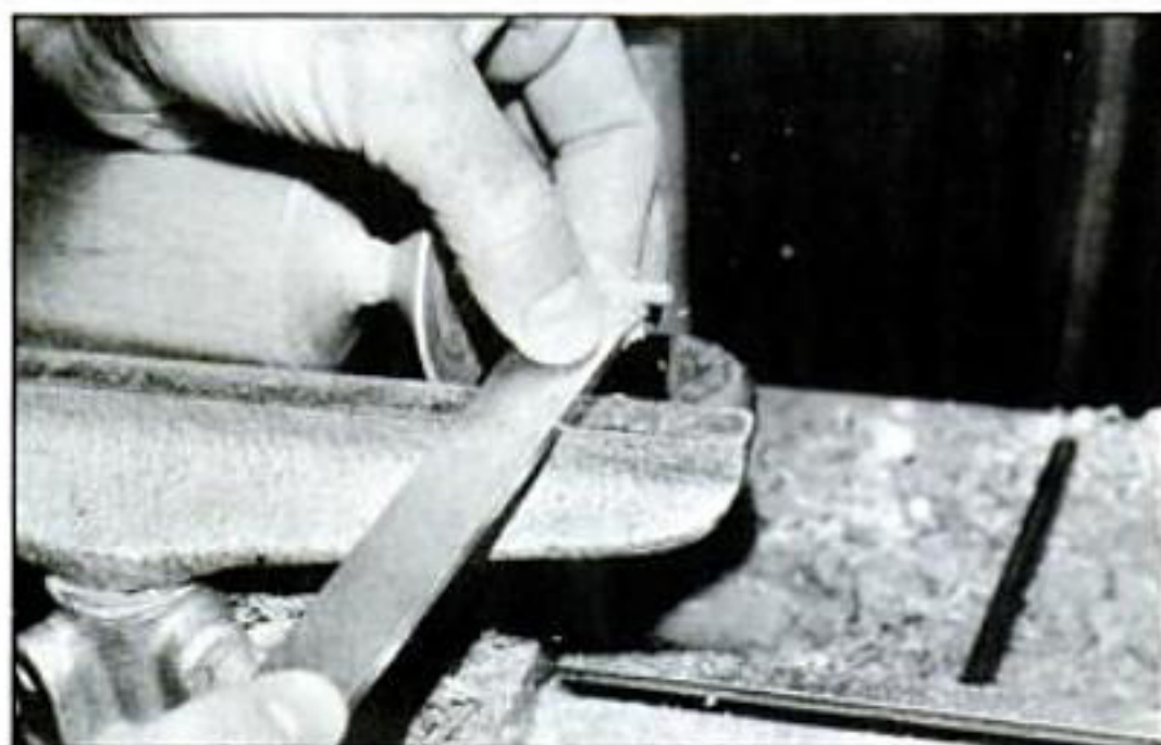
Remove the tailstock and finish the stem with a freshly sharpened skew chisel. Wrap your index finger around the stem and pinch the skew against it lightly.
