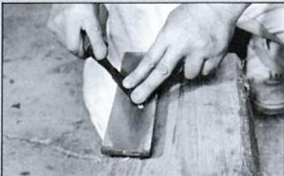
▲ ▼ You don't need to tap out the backs of chisels. Rub the back flat on the lapping plate with a little more pressure toward the edge. On narrow chisels, you only need to apply pressure with your fingers. Hold narrow chisels at an angle so they don't rock.
