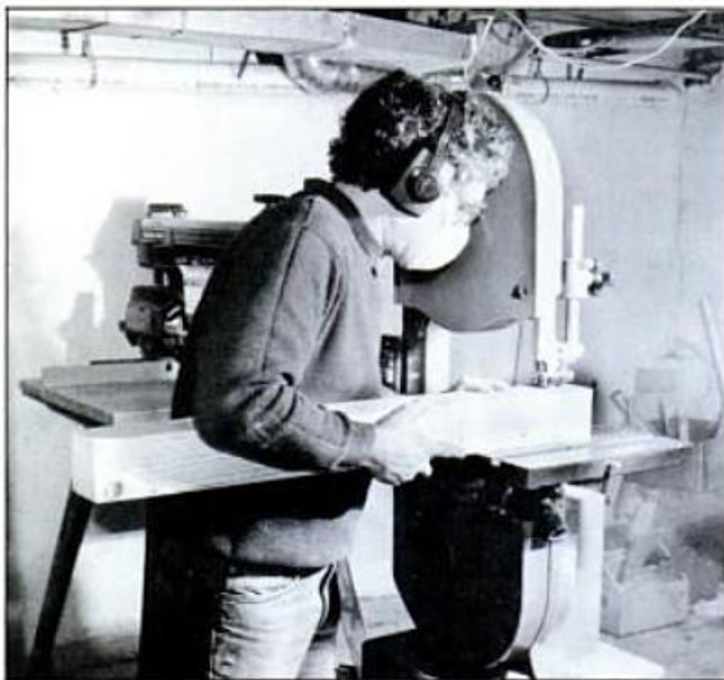
A ½-in. bandsaw blade comes in handy for cutting tenon cheeks and the slot for the slip joint at the top of the legs. Cut both sides of the slot, then make rough cuts in between, like the teeth of a comb. Clean out the waste with a chisel.
