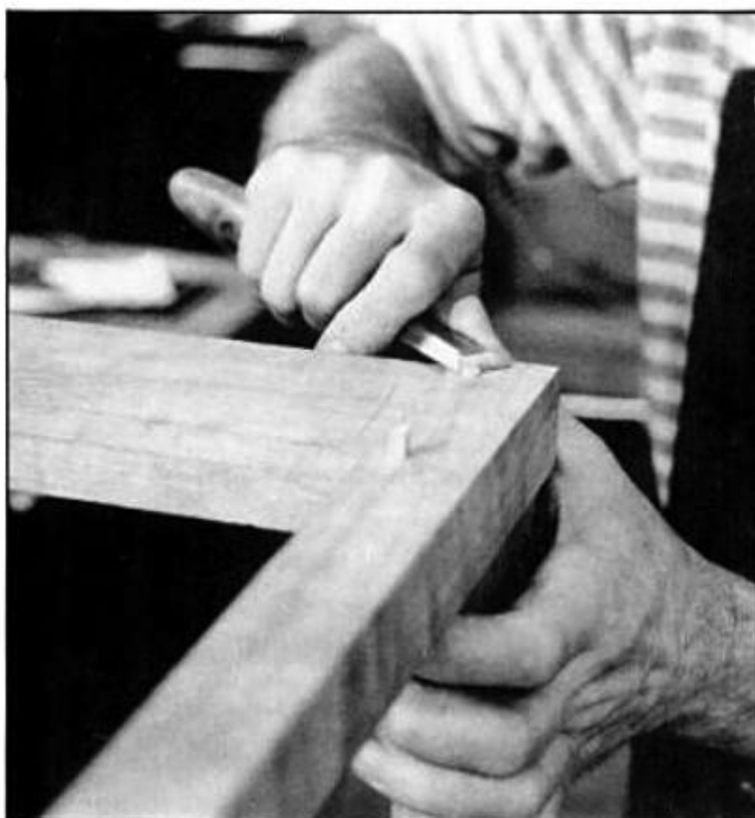
Peg the apron tenons into the leg mortises. First saw, then chisel the protruding peg to bring it down flush with the leg.
