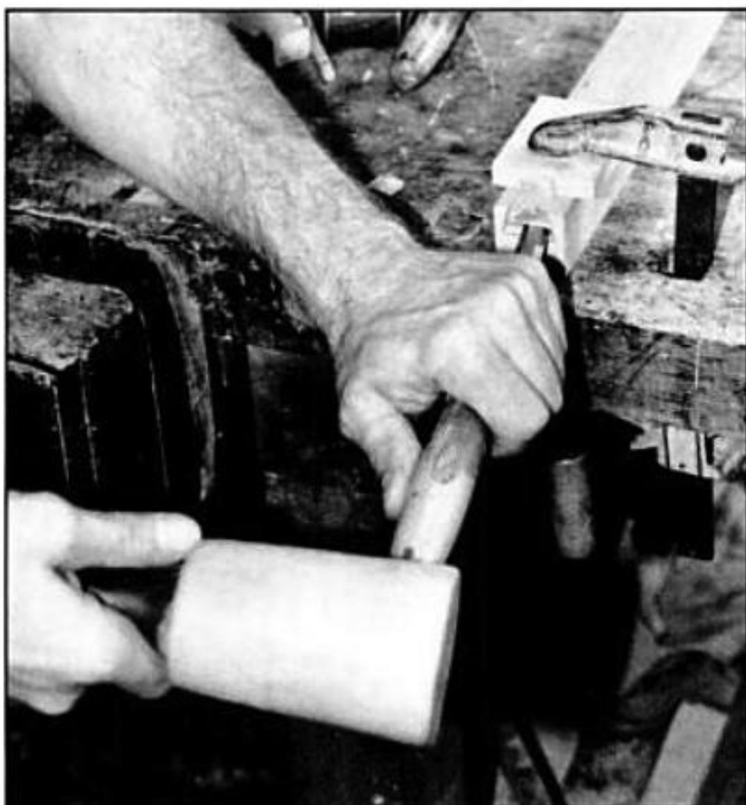
The flat dovetail mortises in the front leg tops are strictly a tap, tap, chop, chop operation. The only secrets are a sharp chisel, a secure hold-down, a good eye, and patient care.
