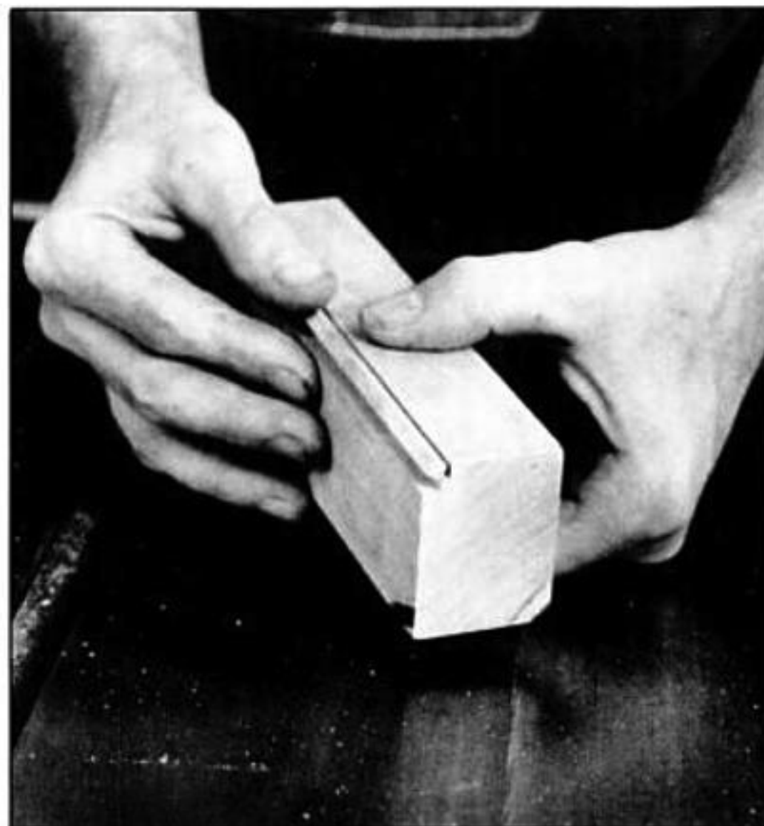
Saw the small square pegs for the leg joints from the corners of scrap stock. To cut them safely, adjust the blade almost high enough for the two cuts from opposite sides to meet, then break the corner out.
