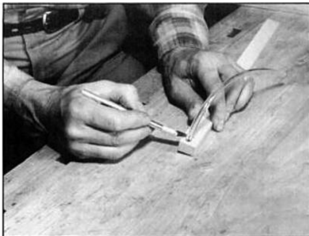
Cut the vinyl tubing sleeves that line the screw holes by running the tubing through a hole in a \frac{9}{16} -in. thick strip of wood and slicing the ends off flush.
