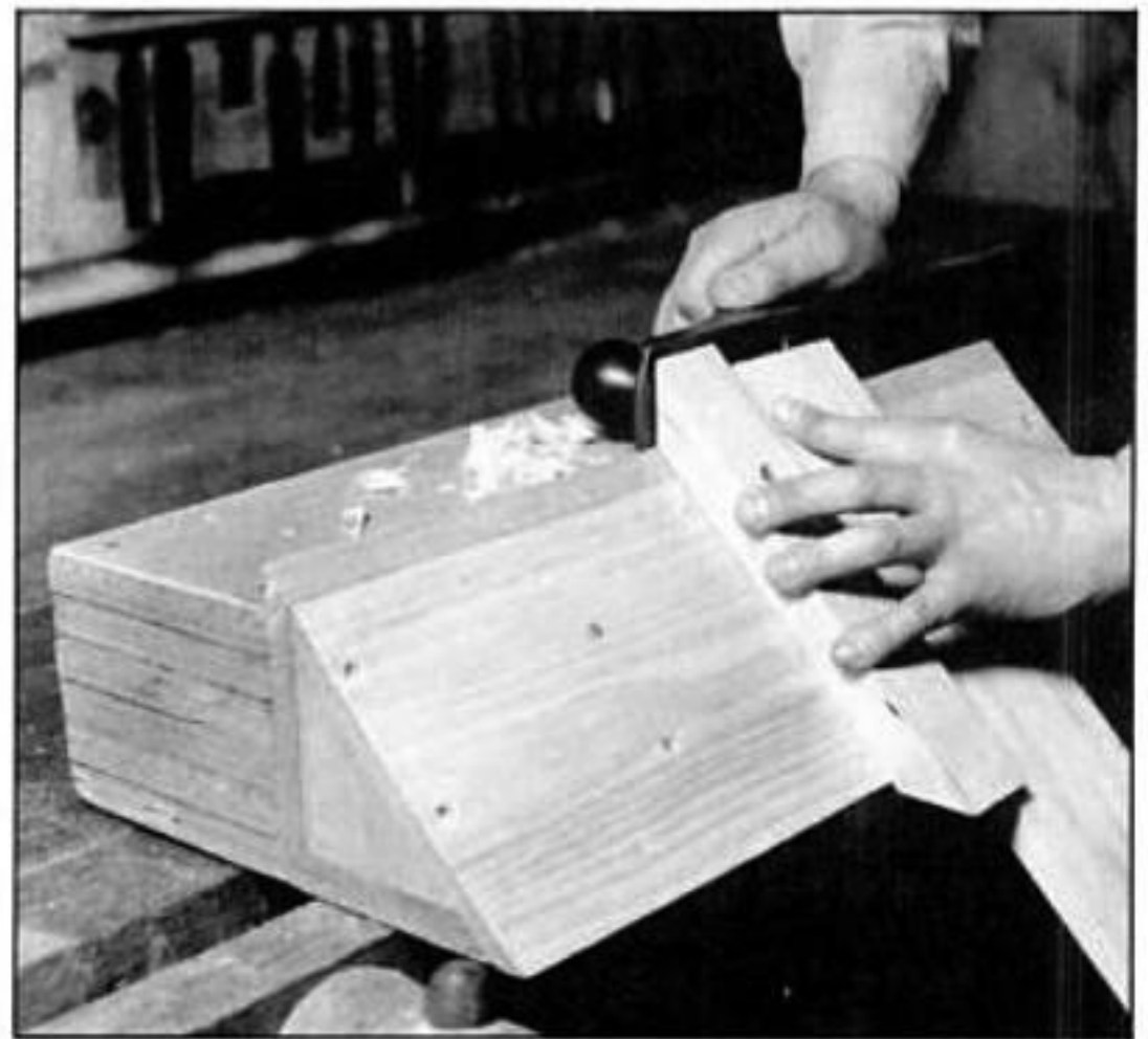
The donkey's ear shooting board is for trimming box or carcass miters.
