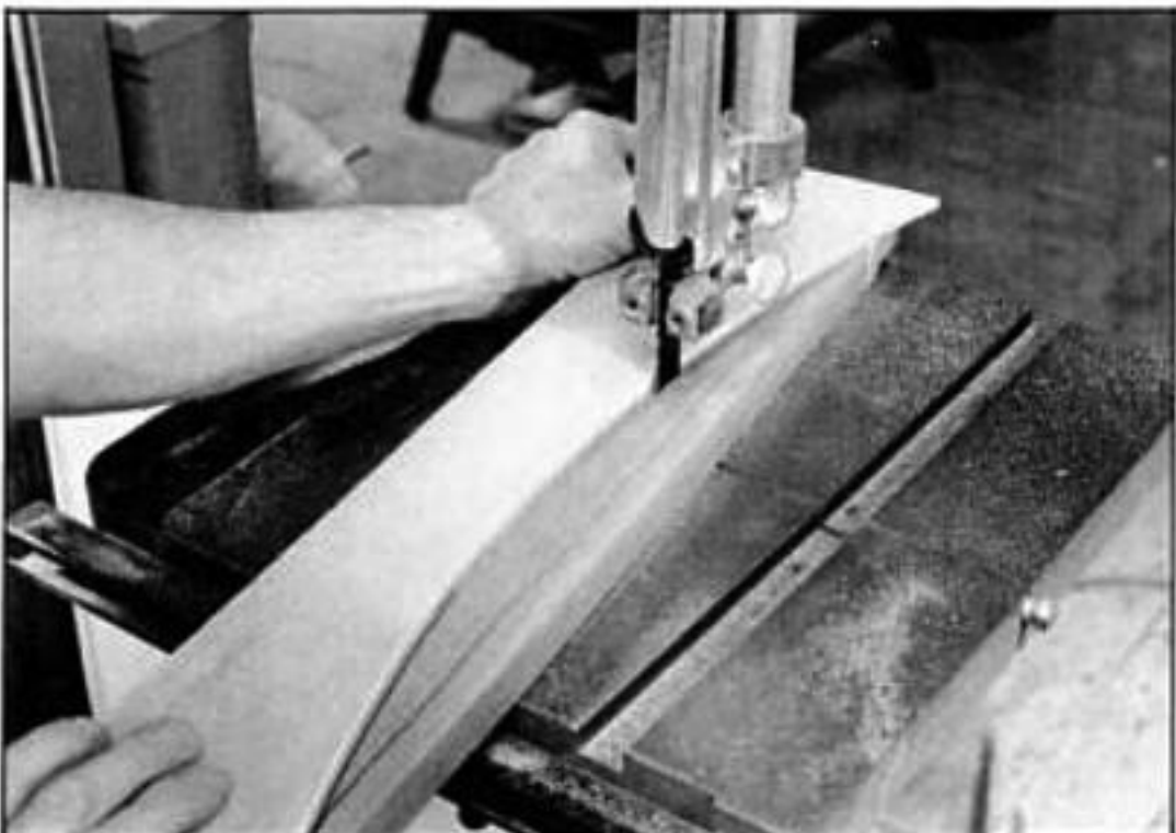
A template speeds the process of curving the aprons. Bandsaw close to the template (above left), then finish up with a flush-trim bit in a router table (above right). The pilot bearing rides the edge of the template.
