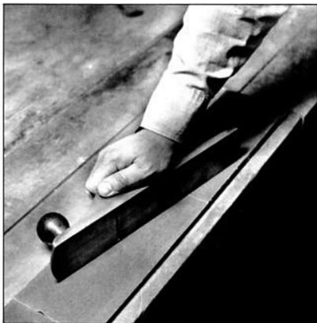
For accurate shooting, the sides of your plane must be square to the sole. You can grind the plane body on emery cloth on a piece of glass.
