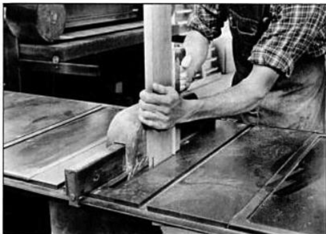
A tenoning jig makes short work of sawing the apron tenons on the tablesaw.
