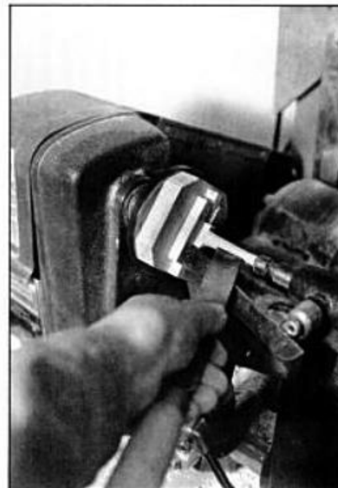
This homemade jig holds the tuning pegs while they are tapered on a lathe. It's easy to remove the pegs to test their fit in the tapered peg holes.
