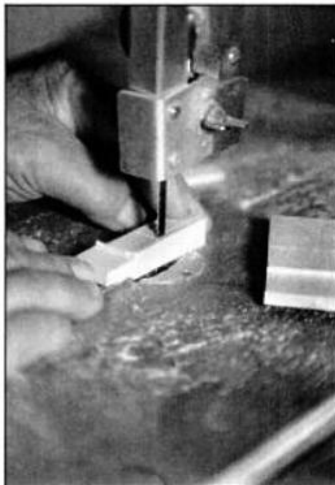
Bandsaw the individual tuning pegs from the rough peg block.
