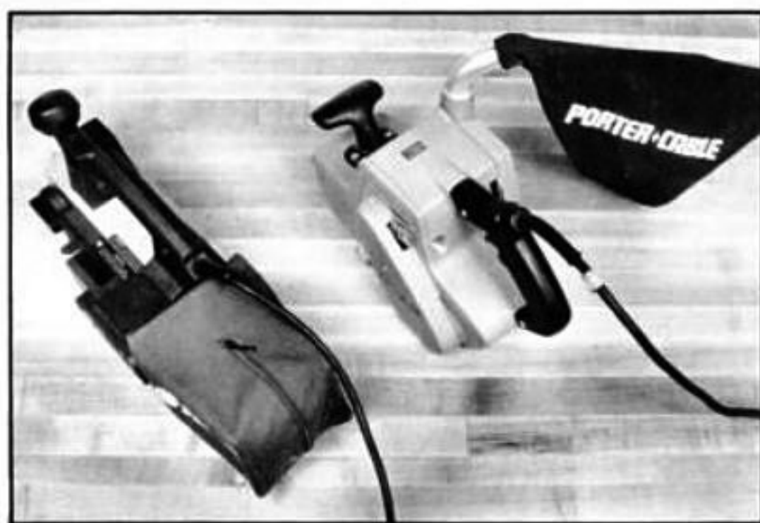
A well-designed sander captures the dust but keeps the dust bag out of the way. The Metabo (left) uses a rear-mounted bag; the Porter Cable bags (right) can be pivoted.
