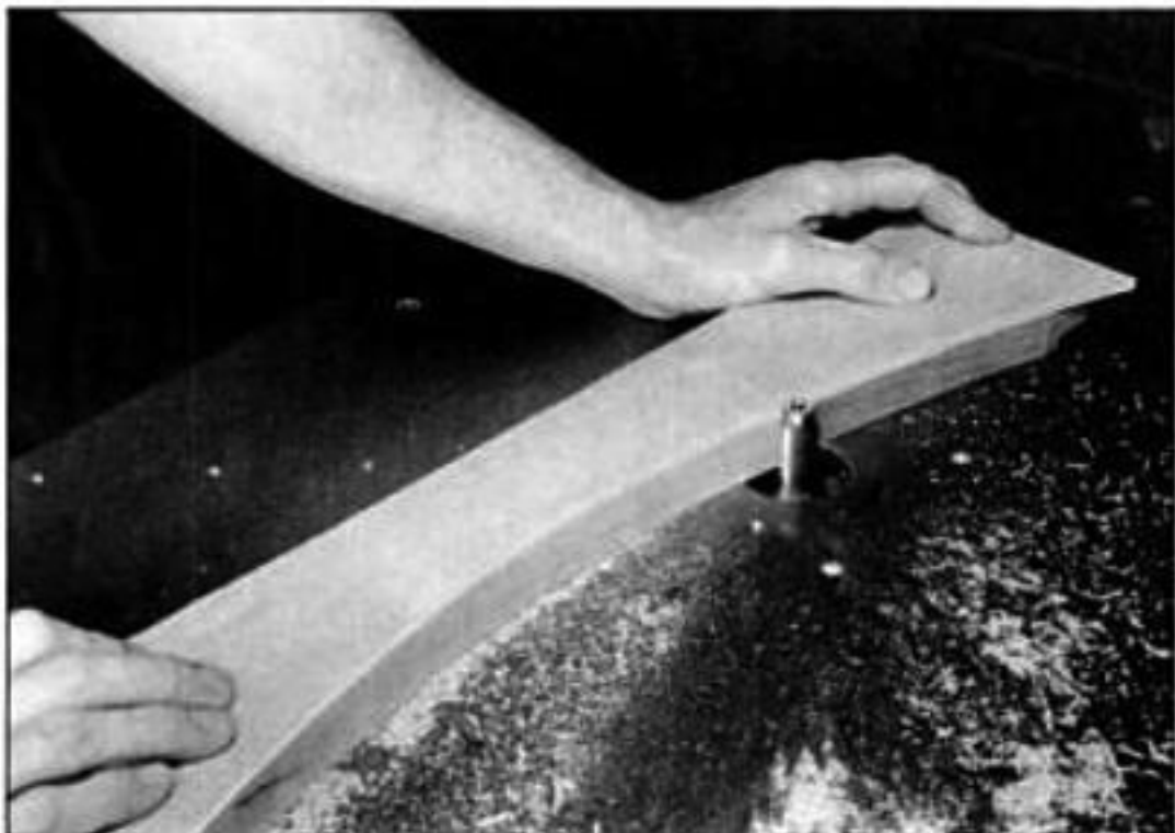
A template speeds the process of curving the aprons. Bandsaw close to the template (above left), then finish up with a flush-trim bit in a router table (above right). The pilot bearing rides the edge of the template.
