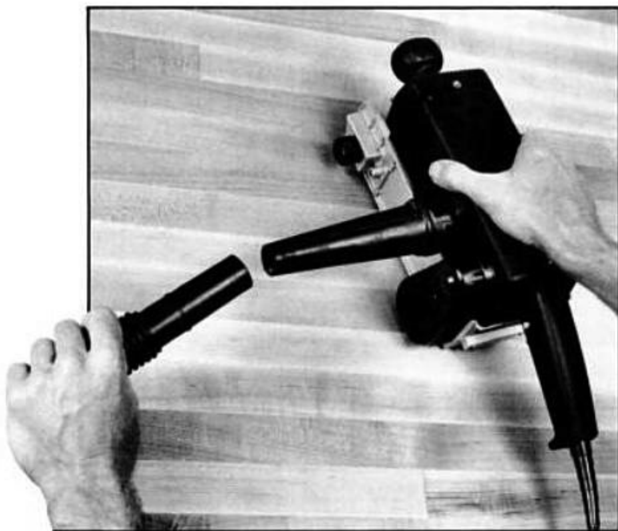
A shop-vac hookup such as this AEG tapered universal-hose connection captures more dust than a dust bag but can be cumbersome to work with.
