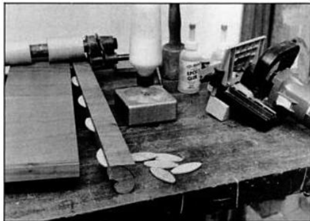
Attach the end pieces with epoxy and plate-joiner biscuits.
