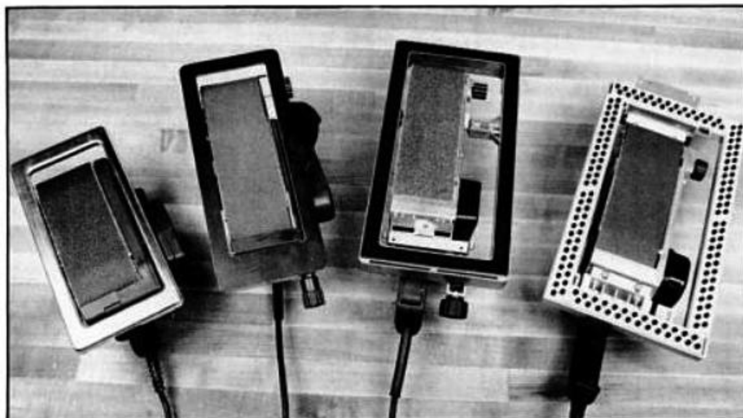
A sanding frame tames the beast; it prevents the sander from tipping, gouging, or excavating valleys in your work. Shown, from left to right, Skil, Elu, Bosch and AEG.
