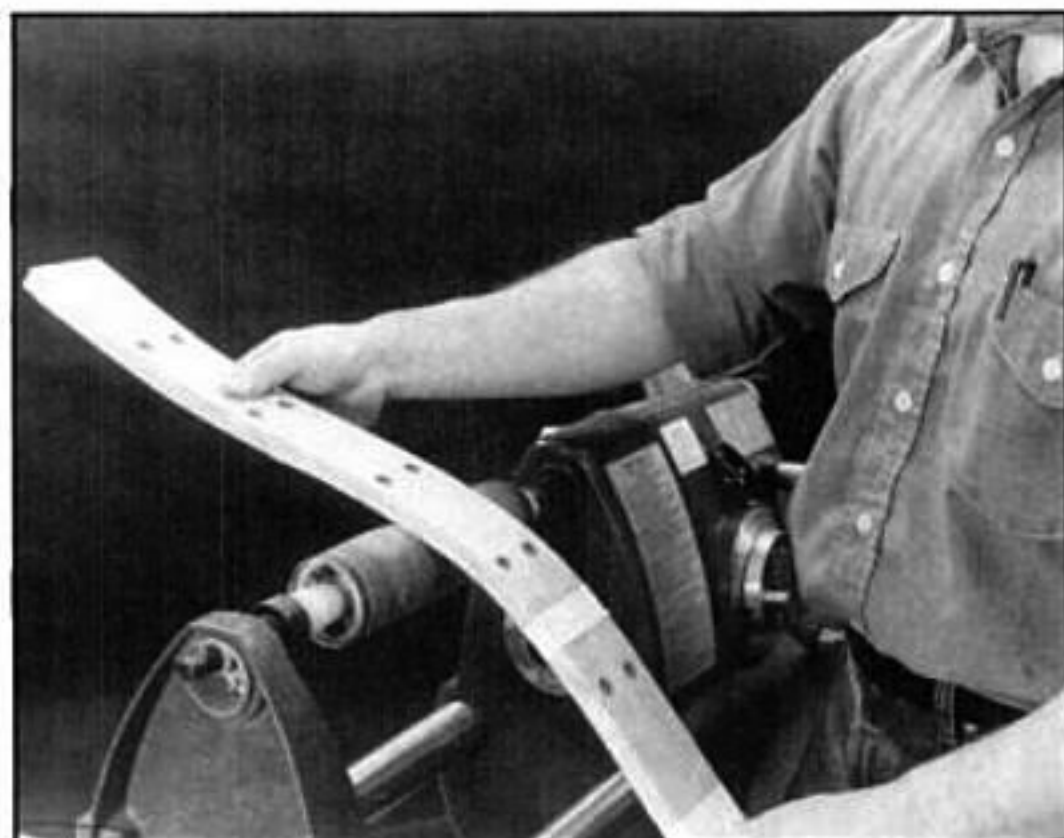
To make certain that the arches match, tape them together edge to edge when you sand them.
