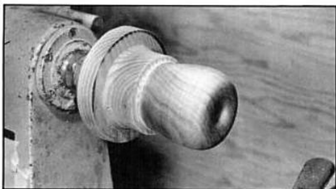
Remove the tail stock, and finish shaping the top of the apple.
