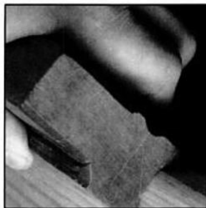
When making a thumbnail profile, start in the middle of the curved profile. You will gradually round the corner of the board. Eventually the drop will form, and the stop will make contact with the board's surface.
