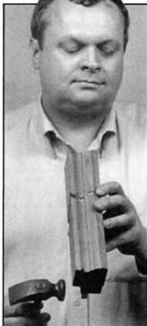
Before honing the bezel of a moulding-plane cutter, flatten it on a lapping table, and polish it on a honing stone.
