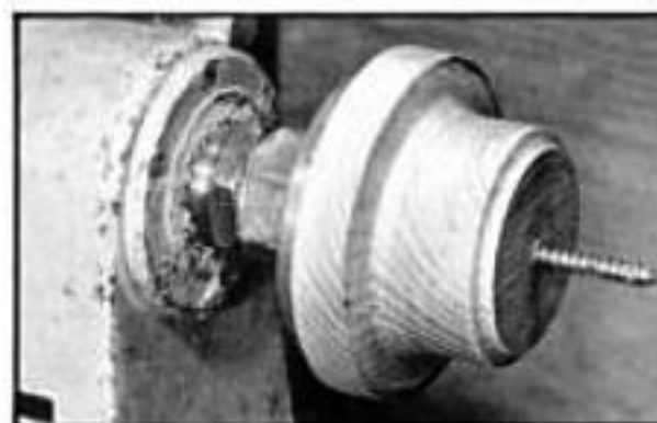
This shop-built screw chuck is easy to make—it's nothing more than a lag screw threaded into a piece of wood.
