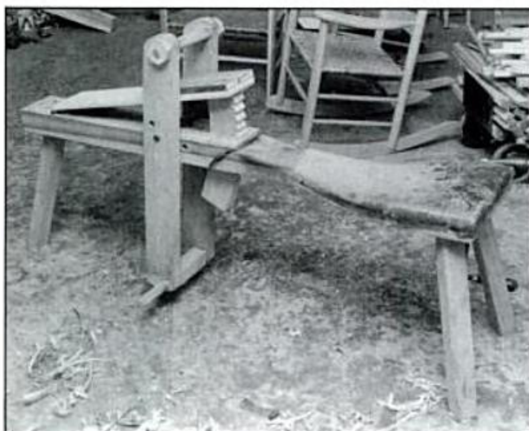
This shaving horse, made by Berea, Kentucky chair maker Brian Boggs, has a ratcheting riser block, to make adjustments more convenient.
