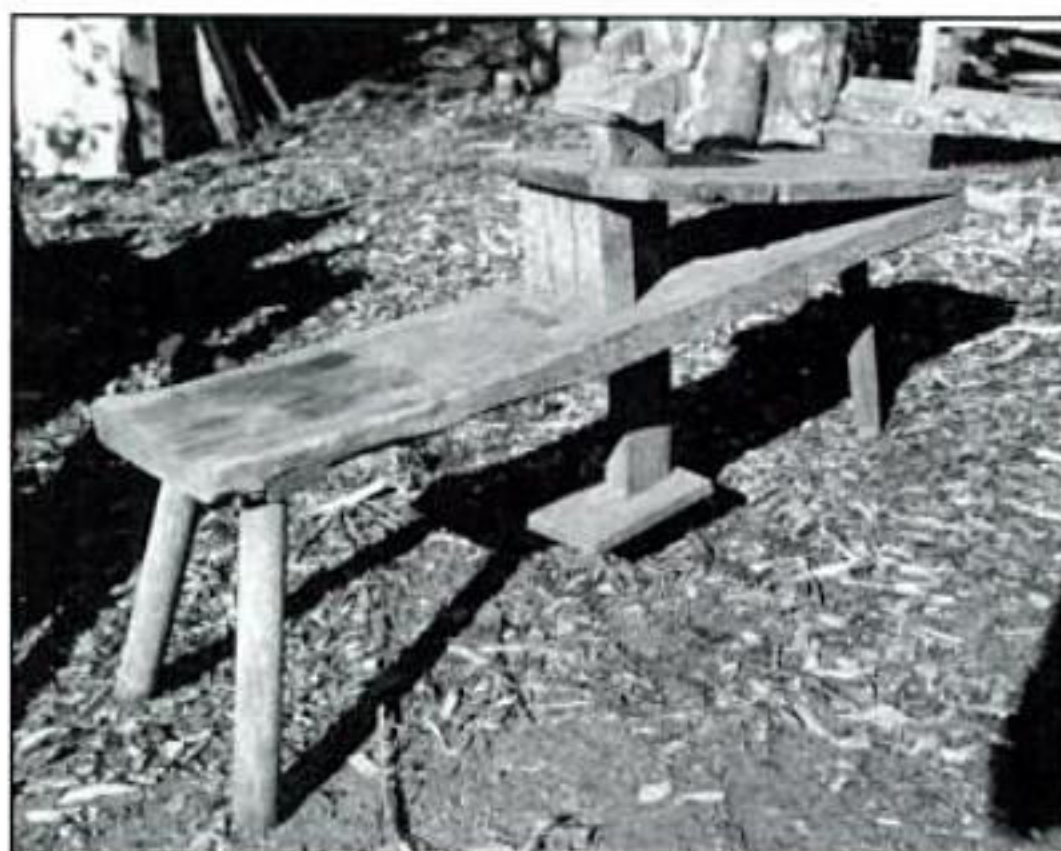
This German-style "dumbhead" shaving horse has a single pivot arm. It's used with longer stock, such as oars or rake handles.
