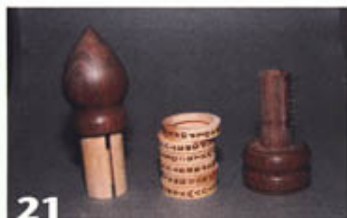
21 Test fit the backbone tube into the top. (All the parts in this photo are ready for assembly.)
