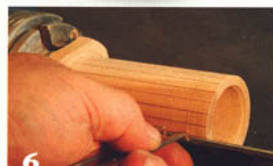
Starting from the tailstock end and using dividers, make a mark every \frac{1}{2} " (12mm). You should be able to mark off six or more rings.
