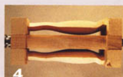
4 Turn the new outer faces to achieve something as shown. Each of the 1" x 3" (25mm x 75mm) workpieces has now been reshaped by turning the two broad faces of the boards. These faces have been thermed.
