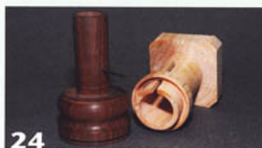
24 The first pin is fitted into the box tube. The code ring on the adjacent backbone tube is used to gauge how long to cut the pin.
