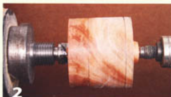
Mark the bowl blank with two lines, one for turning a tenon at the tailstock end, and the other to indicate the eventual transition from straight sides to a hemispherical bottom. At this point, the cylinder's headstock end is sanded to 320 grit.
