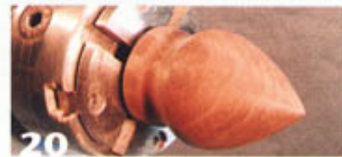
20 Reverse the top and remount it into the chuck and shape the rest of its profile.
