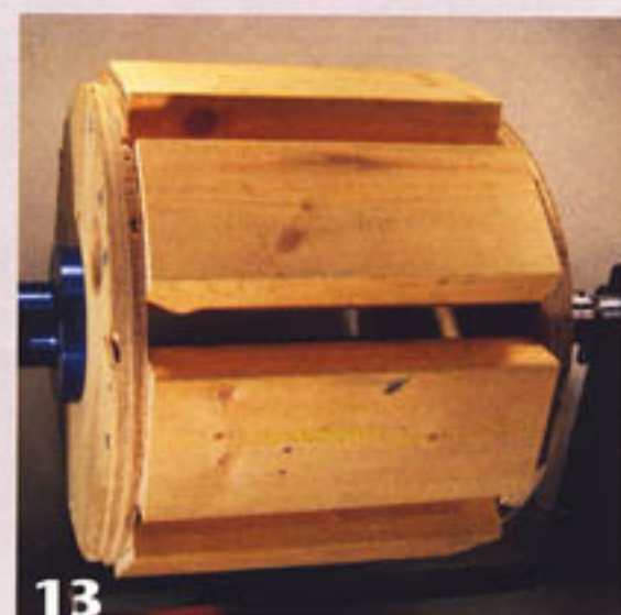
13 The barrel-shaped assembly is mounted to the lathe and is ready for turning the first face of each workpiece.
