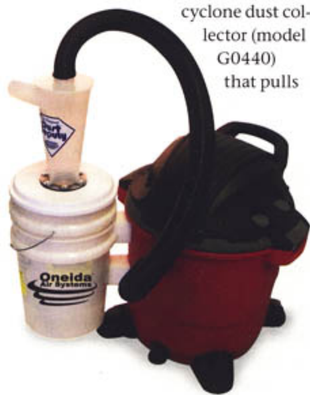
The Dust Deputy from Oneida turns an ordinary shop vacuum into a two-stage unit, where the larger particles are sent to the bucket and the fines are trapped and collected in the unit's standard bin.
