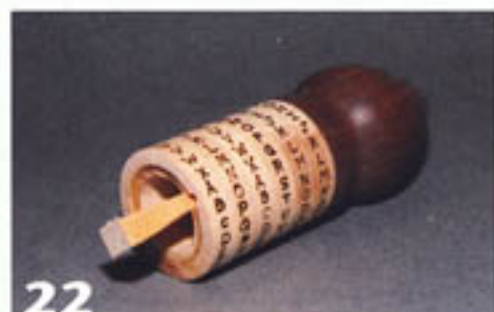
22 Verify that the backbone tube is long enough to come out even with the stacked rings. Use one of the wedges to expand the backbone to make sure that ring 1 can be successfully glued onto the backbone tube.
