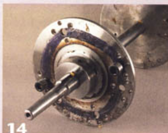
14 The custom-made mounting jig is shown from the Morse taper end. There are two locating pins mounted opposite each other for accurately holding two workpieces for turning.
