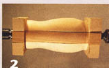
2 The assembly looks like this after turning the outer faces.
