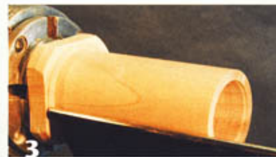
3 The wood is drilled, turned, and sanded and is ready for laying out the segments.
