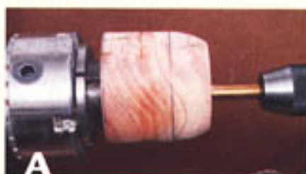
A With the cylinder attached into a chuck, shape the upper part of the spherical bowl form, then drill the interior.
