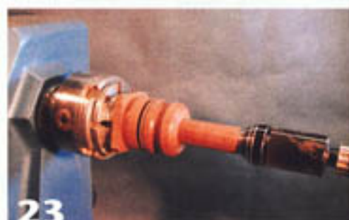
23 Remount the box tube/base into the chuck and turn the base to its final shape.
