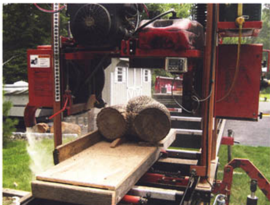
A horizontal cut through this ash crotch required a bit of wedging to stabilize the log. The sawmill delivered precise placement of cuts, which resulted in wood that was easier to process and also minimized waste.
