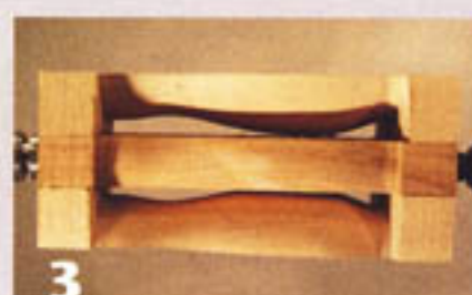
3 After turning the outer faces, dismantle the assembly and reassemble with the workpieces flipped over.
