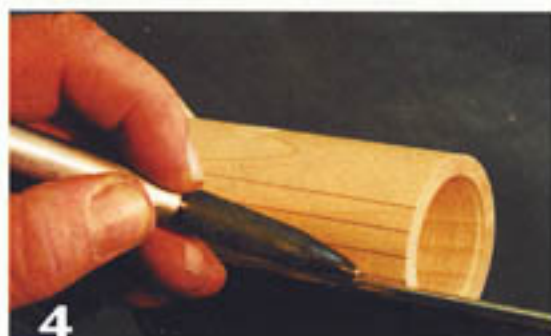
With the lathe's index pin engaged, draw the lines for the segments. Use a soft-lead pencil and run it along the toolrest.
