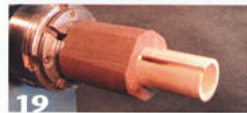
19 Test fit the backbone in the recess. The goal is to achieve a light friction fit to prevent squeezing out all of the glue.
