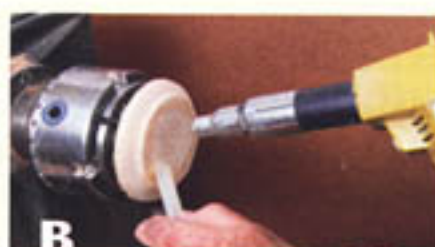
B First apply a thin layer of hot melt adhesive to an auxiliary blank using a heat gun. Hot melt adhesive will also be applied to the rim of the bowl blank.
