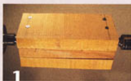
1 Two 1" x 3" x 9" (25mm x 75mm x 230mm) workpieces are screwed to a 1" x 3" (25mm x 75mm) carrier (the middle layer). The assembly is mounted between centers.
