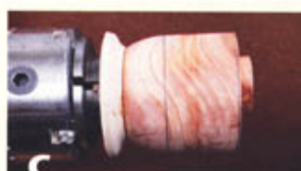
C The bowl blank is attached with hot-melt adhesive. To achieve a strong bond, the tailstock was used for pressure during the curing process.
