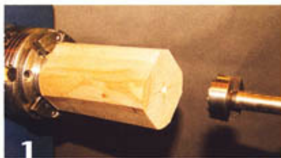
1 With the blank for the code rings mounted into a chuck and a Forstner bit mounted in a Jacobs chuck, drill out the inside of the wood to form the code rings.
