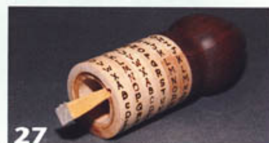
27 Use one of the wedges to expand the backbone so that ring 1 will be successfully glued onto the backbone tube.
