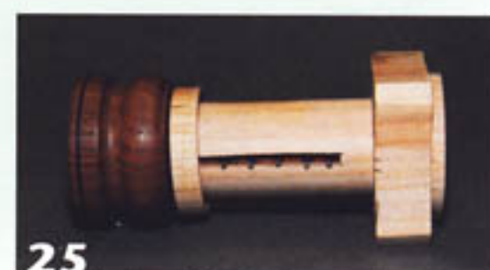
25 Trial fit the box tube, backbone tube, and code ring to verify the correct lengths of the locking pins. Check for binding of the pins within the slot.
