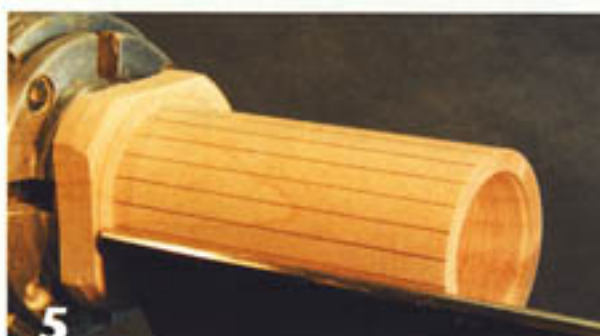
The wood is ready to mark for the code rings.
