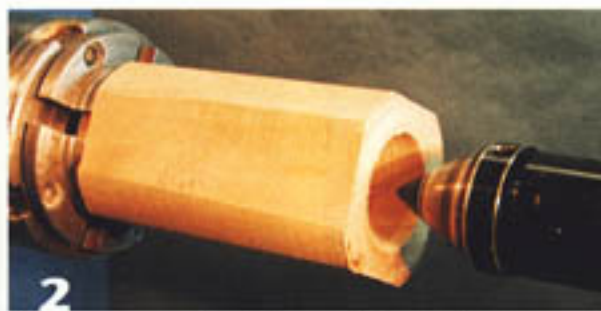
2 Use a cone center to help minimize flexing and vibration and to help compensate for any offset errors created in the drilling process.
