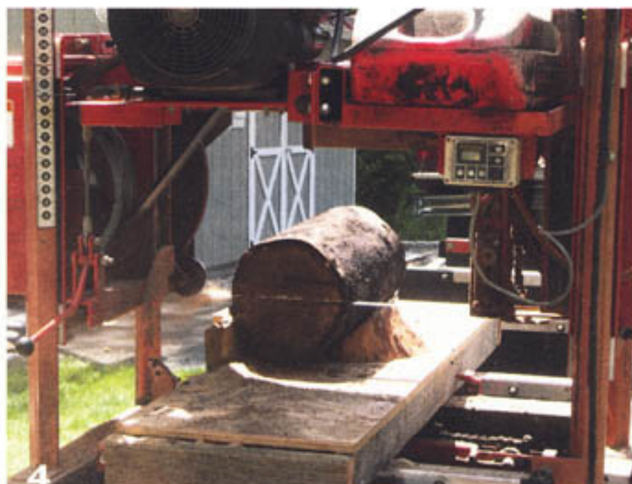
Our sawmill setup consisted of a wooden platform with a fence and wedges to hold the logs in place.
