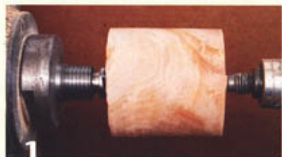
A cherry-wood bowl blank is turned between centers to a diameter of about 3½" (90mm). When the piece is mounted on the lathe, the wood grain runs vertically, as is the case with most turned bowls.
