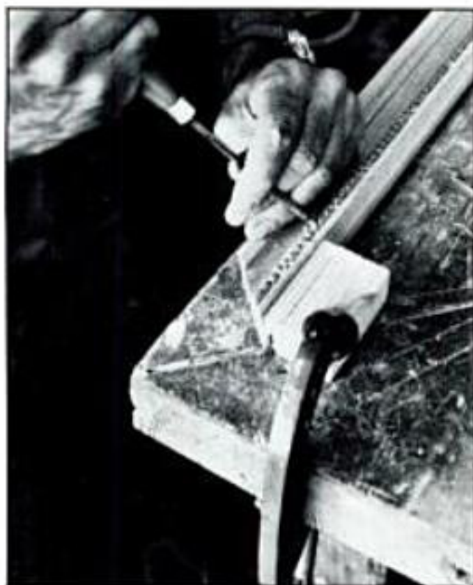
Define the perimeter of each berry by rotating the gouge around the base, cutting to the depth of the flat on either side of the bead.
