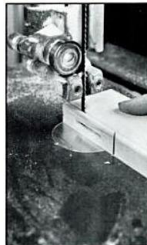
First, miter the door-frame beads at the inside corners where the stiles and rails meet. Then, remove a section of the beading by cutting down the bead groove to the miter on the door stiles and rails.
