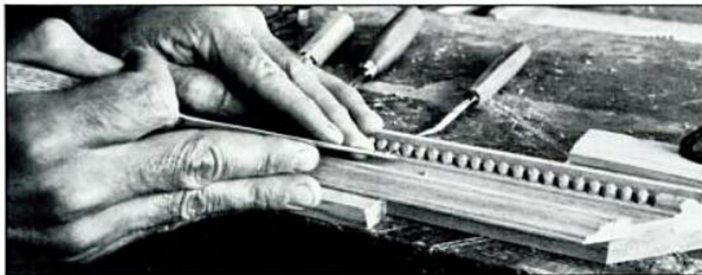
Run along the edge of the berries with a fishtail gouge to pop out the waste from between the berries. Use a pick, or your smallest gouge, to pop out the waste on the opposite side of the berries.
