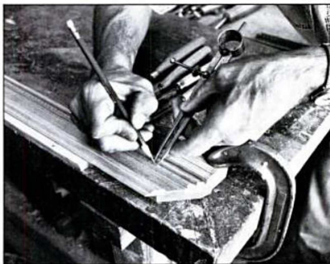
Mark out a half berry at either end of the molding, and divide the space between into groups of three berries. Then, go back and mark the center of each individual berry.
