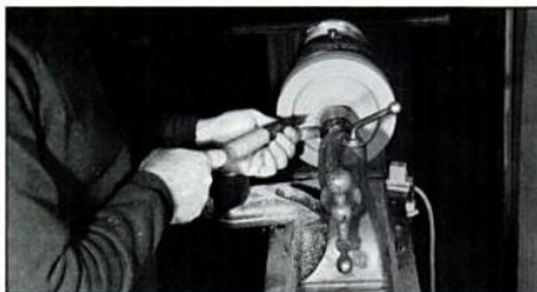
Part off the roof rings holding your parting tool at a consistent angle. It helps to shift back and forth between the cuts to do this.
