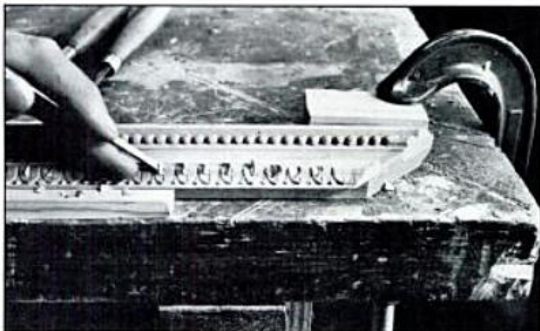
Round over the tops of the leaves with a #5 gouge, bevel-side up.
