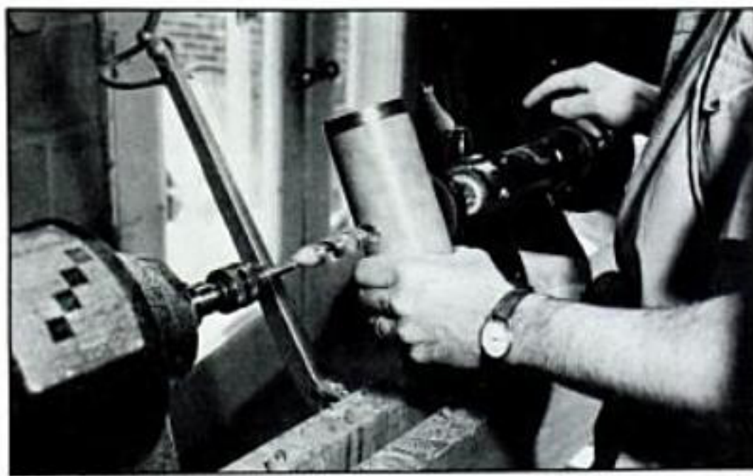
Drill a 1-in. hole through the mallet head for the handle tenon. Here, the author uses a "crotch center," a V-block device that fits into the tail stock for boring round shapes on the lathe.
