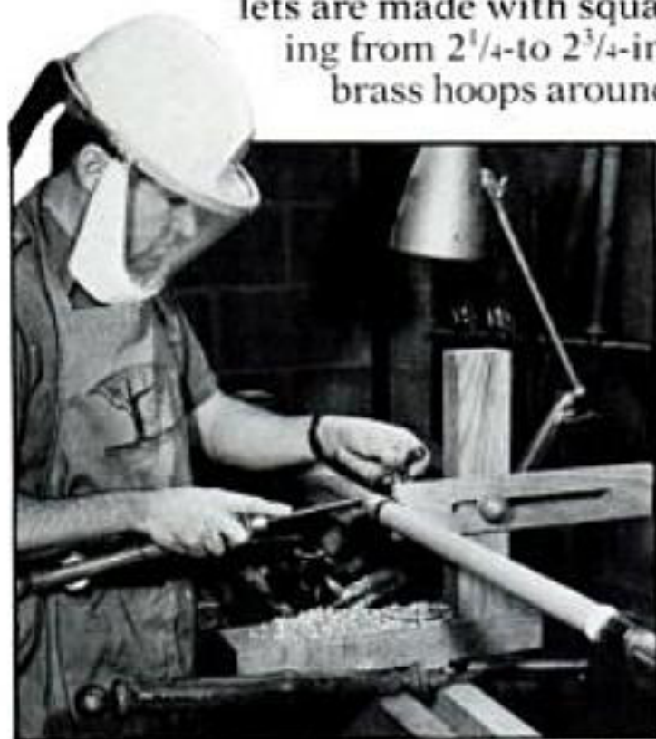
Support the handle with a steady rest at the center. Turn to either side, then reposition the steady rest to finish the center of the handle.
