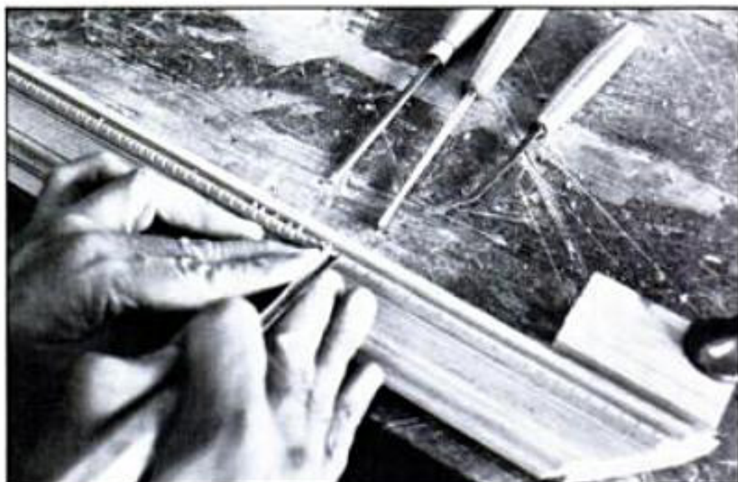
The first step to carving the berries is to make a V-cut between the berries with a parting tool.
