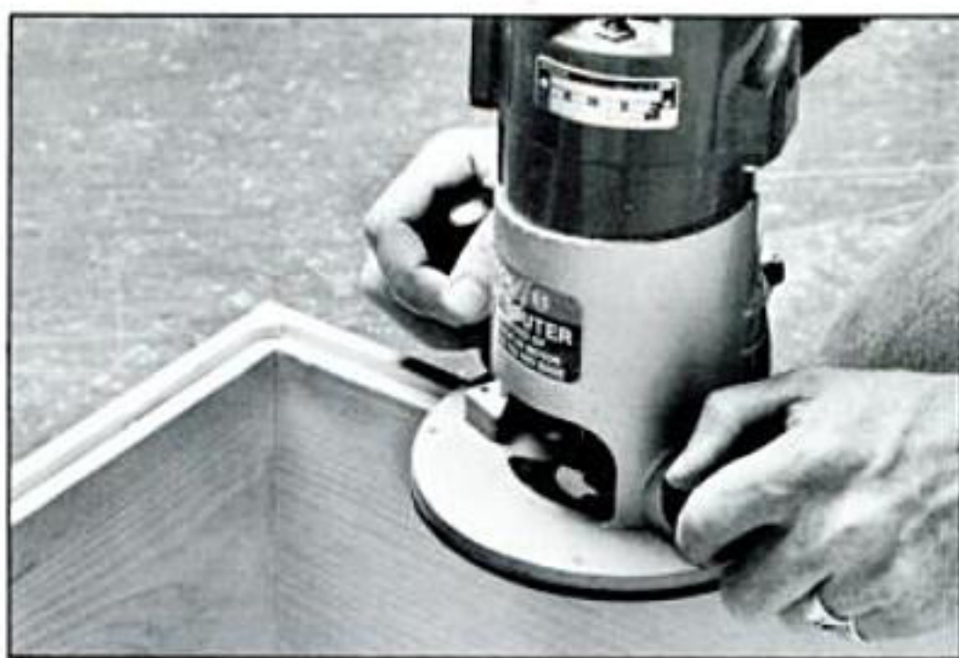
A \frac{3}{8} -in. rabbeting bit, set for \frac{1}{4} -in. depth-of-cut, makes a perfect recess for fitting cabinet backs. Rounded corners left by the bit can be squared up with a chisel.
