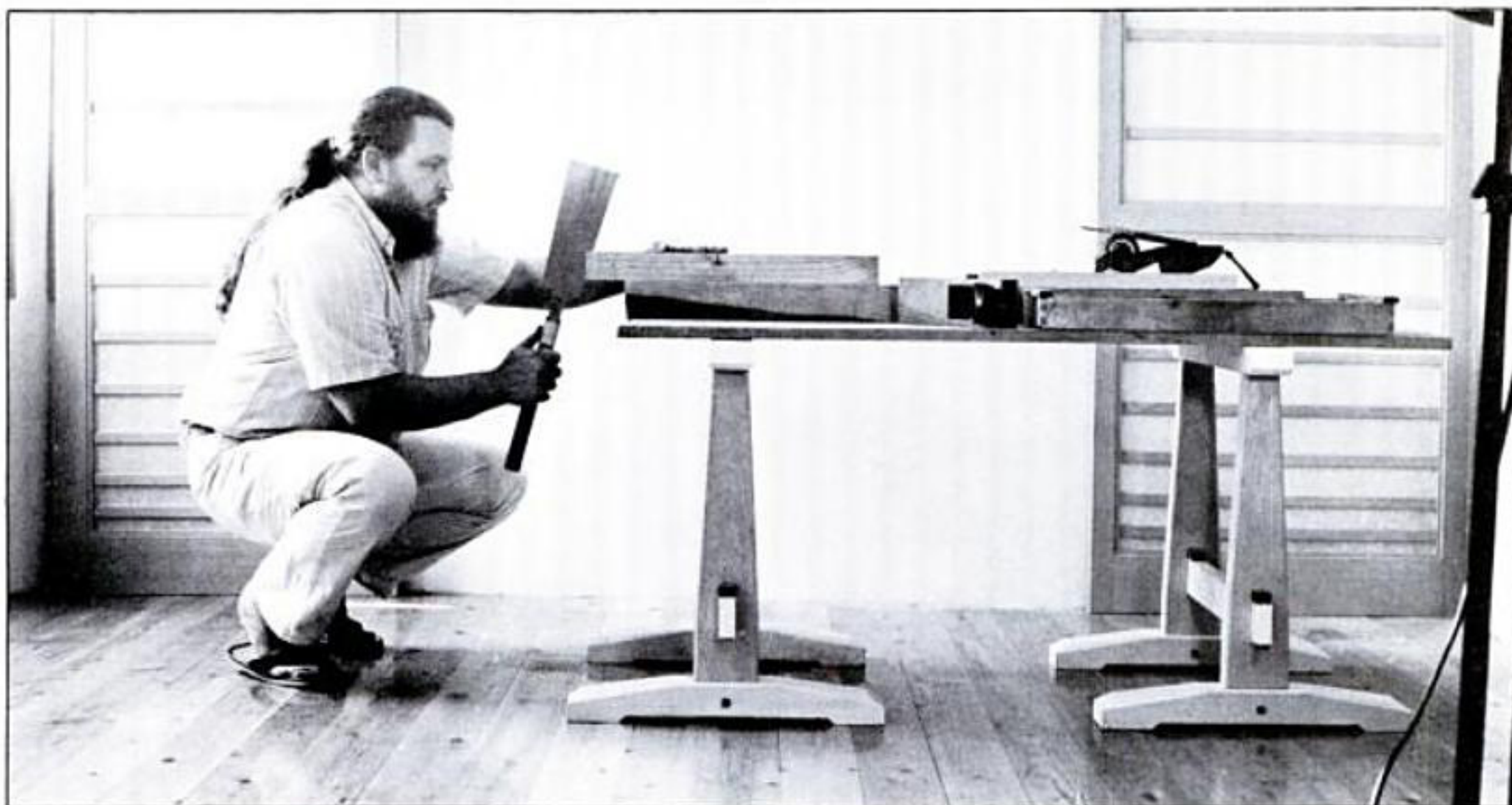
Cut the sawhorses' leg tenons carefully, letting the saw kerf take half the layout line. The Japanese saw cuts on the pull stroke, making it easy to hold the work by hand.
