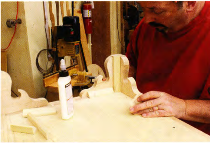
22 Strengthen the feet with blocking. A vertical block actually carries the load of the chest.
