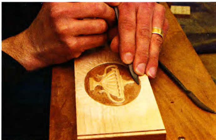
12 Rifflers are handy for filing odd shapes and hard-to-reach areas. Use a riffler with a simple curve to flatten the ground and define the wall of the oval surrounding your sgraffito design.
