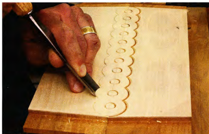
9 Use stab-and-relief cuts with a single gouge to create the guilloche pattern while exposing the dark substrate.
