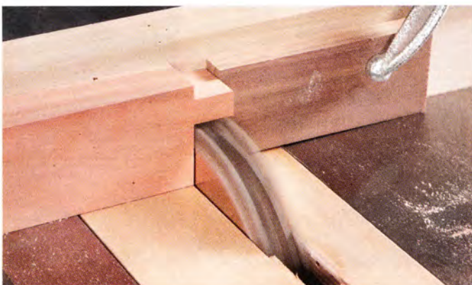
6 Cut both sides of the tenons using a dado stack.
