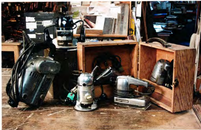
6 Herman's multi-generational company has been around so long, he owns some of the original power tools from when they first came out. The "Take About" sander allowed the worker to bring the sander to the project rather than vice versa.
