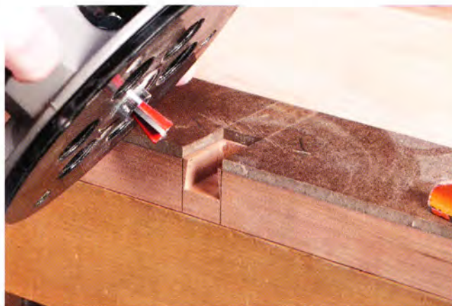
1 Rout the joint's socket using a shop-made template.
