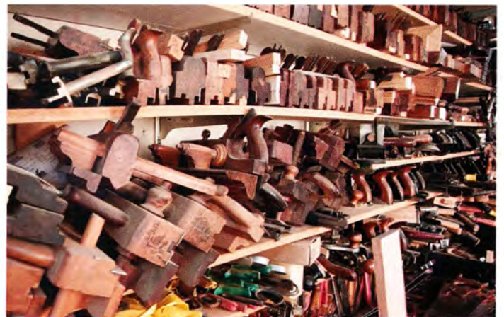
4 For small production runs, Herman still prefers molding planes over routers and shapers. "I can make 20 feet of molding by the time you get your router set up."
