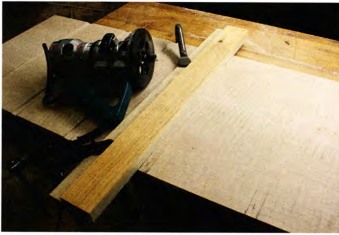
5 A piece of plywood with a narrow second piece stacked and attached on top makes a great fence to guide my router and top-mounted pattern bit when cutting the dados.
