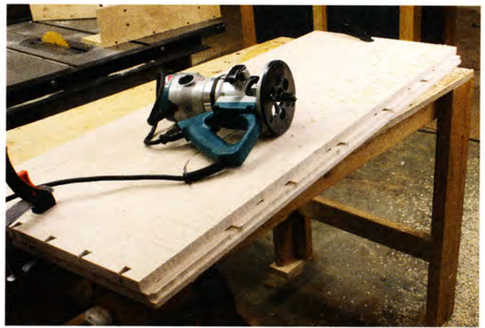
6 Cut rabbets for the backboards using a pattern bit. Climb-cut the first pass, then finish the cut moving left to right as you work.
