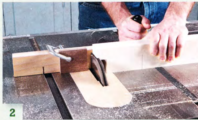
2 Notch the upper end of each leg to receive the bench's top.
