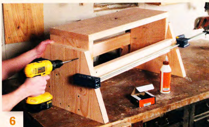
6 Fasten the legs to the lower unit. When the two units are stacked, the flared legs provide a wide, stable base.
