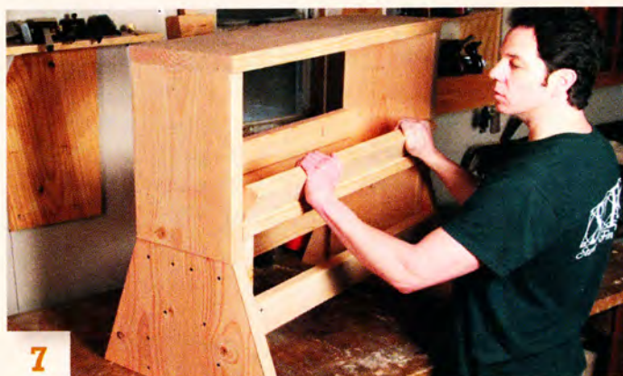
7 Place the upper unit on the lower unit, then fasten stretchers to the upper unit. They stiffen the upper unit and form a tool tray.
