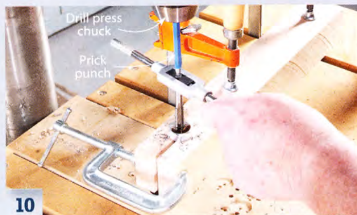
10 Tap the hole. Use the drill press to keep the tap vertical.
