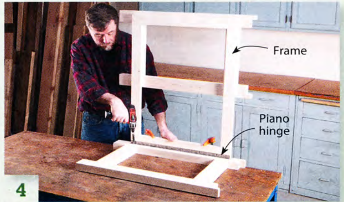
4 Connect the two ends with a rectangular frame. Fasten the frame with piano hinges.
