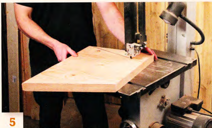
5 Saw the legs of the lower unit from two 2x12s glued together. Freehanding is OK—the cut doesn't have to be perfectly straight.
