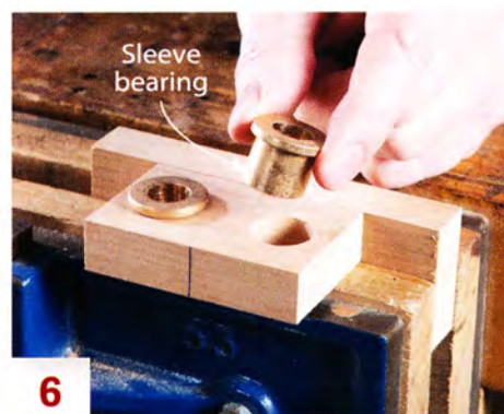
6 Push the sleeve bearings into the holes.
