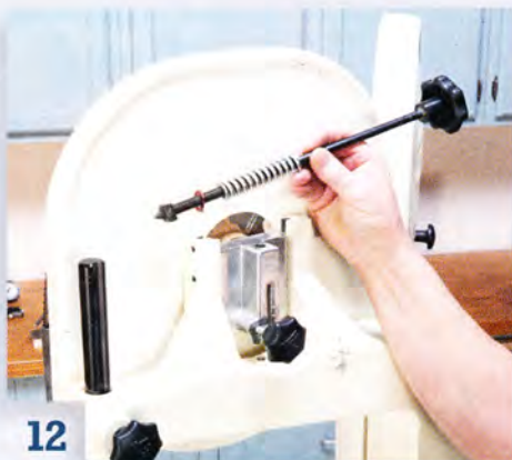
12 Remove the existing tensioning system from your saw. Unscrew these pieces and remove them separately.
