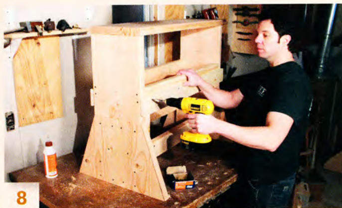
8 Fasten battens to the stretchers. The battens lock the upper unit in place by preventing it from shifting side to side.
