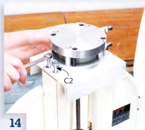
14 Secure the mounting plate to the riser assemblies with lag screws (C2).
