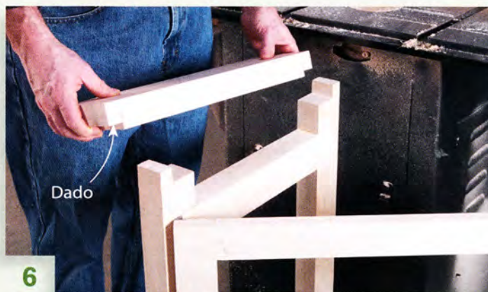
6 Cut dados up to the marks in both breadboard ends. Test the fit of these pieces—they should fit snug in the notches.
