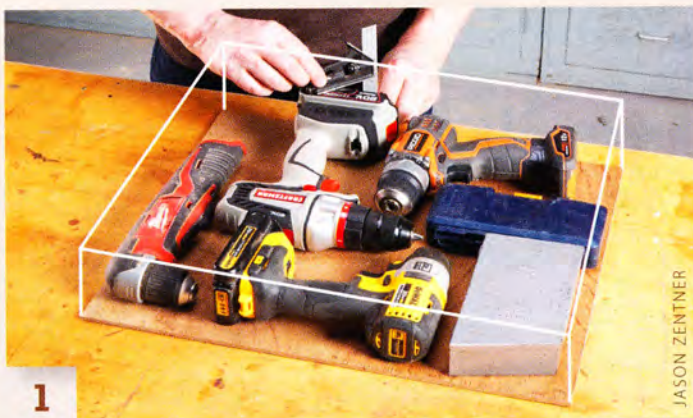
1 Size the drawers to hold the tools you have. A piece of plywood or cardboard the same size as the drawer bottom helps.
