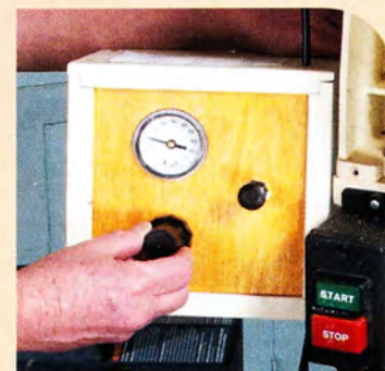
Blade Tension in PSI*
