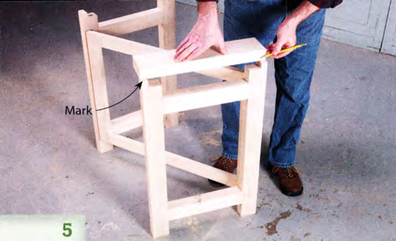
5 Mark the distance between the leg notches on one of the top's breadboard ends.
