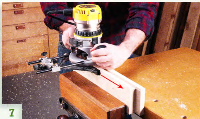
7 Rout a groove in each breadboard end to receive a spline. Glue the main part of the top together and rout similar grooves across both ends.
