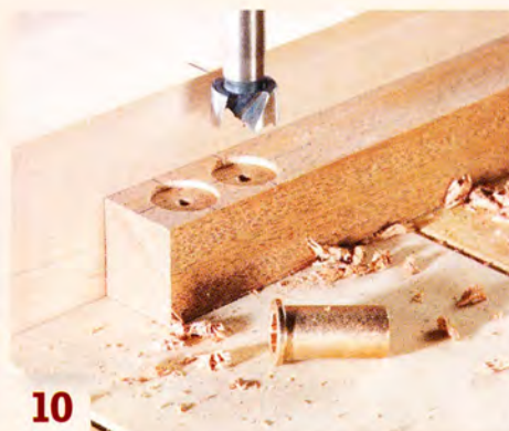
10 Counterbore shallow holes first, then drill all the way through with a smaller bit.
