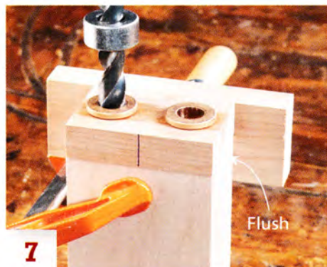
7 Clamp the jig flush with each side of a rail.
