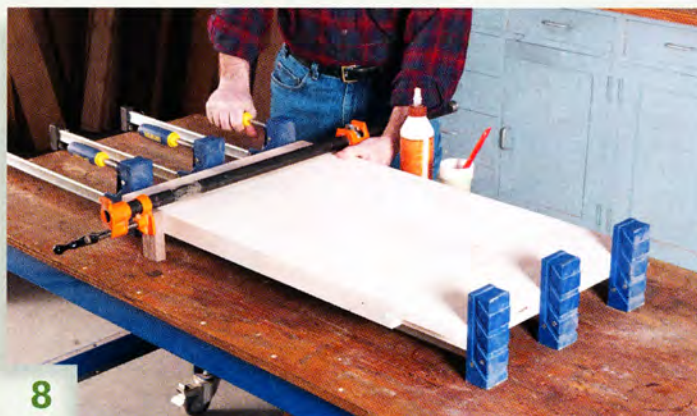
8 Glue the breadboard ends to the top. Use an extra clamp to make sure that the ends are flush, side-to-side, with the top.
