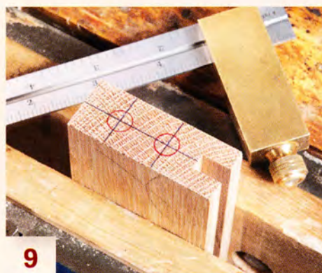
9 Lay out the dowel holes. They can be spaced any way you wish.
