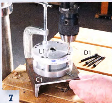
7 Center the air cylinder (L1) on a mounting plate (C1). Drill holes for attaching the cylinder with cap screws (D1).
