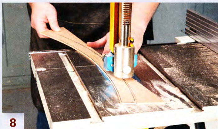
8 Bandsaw 1/8" thick hardwood caps to cover the drawer front's laminations and to protect the veneer. Glue and clamp the caps to the top and bottom edges of the drawer front.
