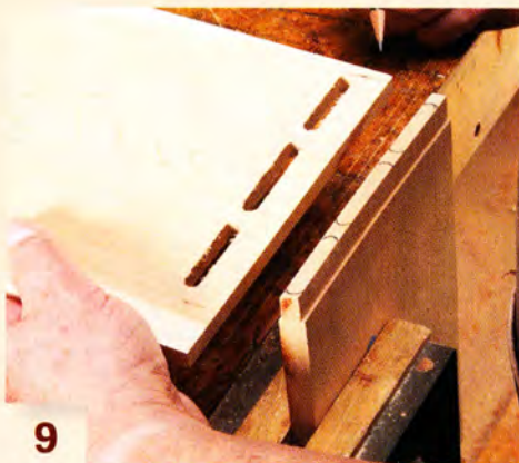
9 Use the mortises in an end piece to mark the rounded tenons on the adjacent side piece.
