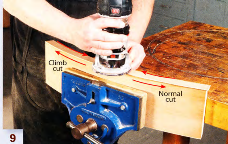
9 Trim the caps flush. Climb-cut half of each edge to keep the wood from splitting. (Climb-cutting means pushing the router in the same direction as the bit is spinning. Please be careful.)
