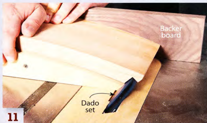
11 Cut rabbets to receive the drawer's sides. This three-sided drawer required rabbets tilted at 45°. For a standard rectangular drawer, the rabbets would be cut at 90°.
