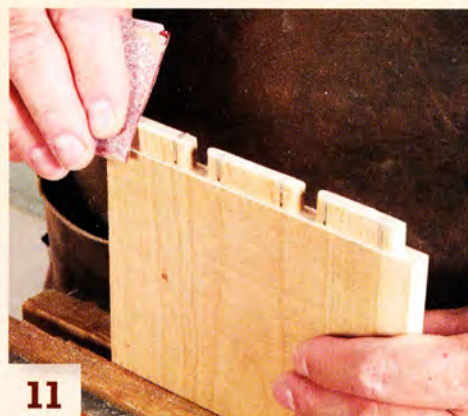
11 Slightly round the ends after shaping the tenons to fit the mortises in the sides.
