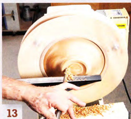
13 Use this chuck to create a hollow base with a rim, add lines or beads, remove screw holes and chuck marks or fully round the bottom.
