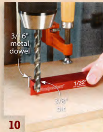
10 Set up a drilling jig with a group of setup blocks or a single shop-made block.
