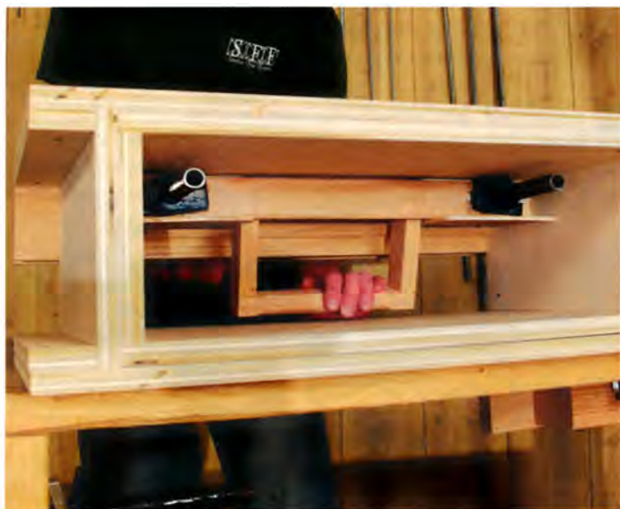
Pull the handle towards you to release the clutch plates for quick adjustment of the front jaw.
