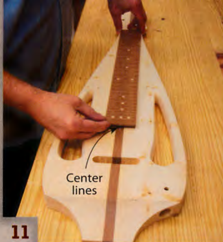
11 Glue the fretboard on the body, making sure it's perfectly centered and flush with the base of the headstock.
