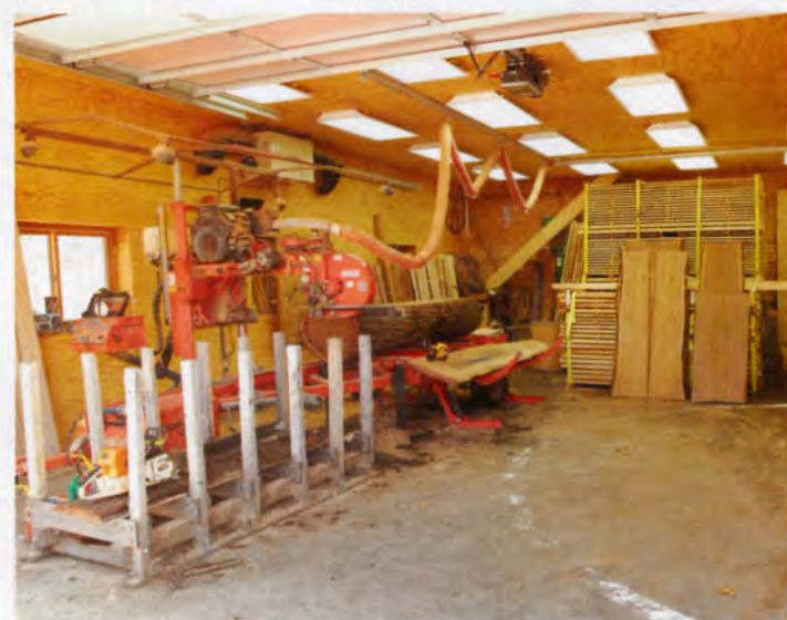
Brian's Wood-Mizer handles logs up to 42" in diameter.
