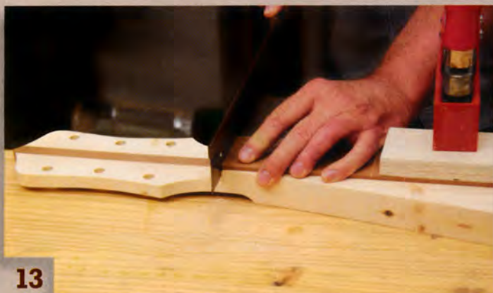
13 Cut a groove for the nut at the end of the fretboard. Register the saw against the fretboard to cut the groove's inside shoulder.
