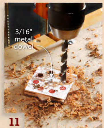
11 Rotate the blank on the jig and drill. Align the bit in each hole's center by eye.
