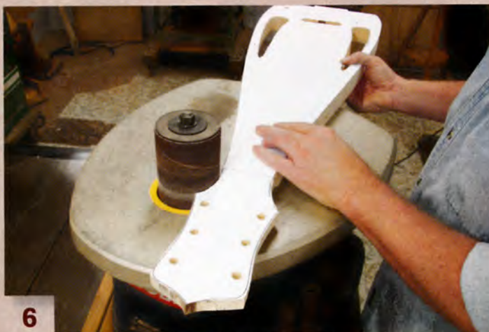
6 Smooth the saw cuts and refine the body's shape using a spindle sander.
