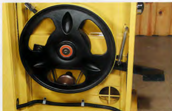
The foot brake shuts off the motor electrically and stops the drive wheel mechanically within five seconds.
