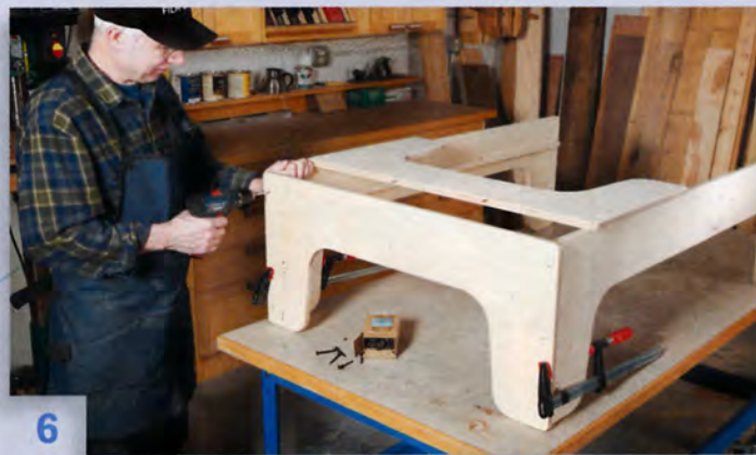
6 Fasten the table together. Place the second end piece on top of the sides to hold the table square. The end pieces have dados that lock the side pieces in position.
