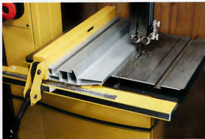
An extruded aluminum faceplate that can be positioned vertically for resawing or horizontally for narrow cuts in thin stock maximizes the versatility of the T-square-style fence.
