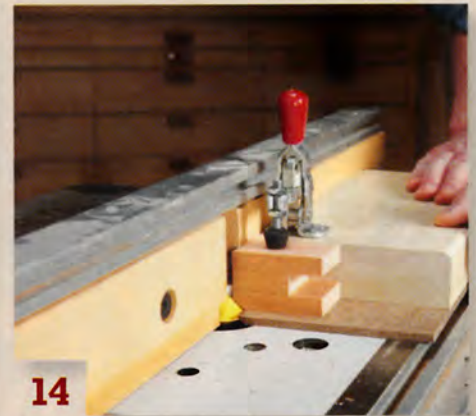
14 Use a sled to chamfer the sliding jaw. Make the sled by gluing a squared block onto 1/4" hardboard and attaching a toggle clamp.
