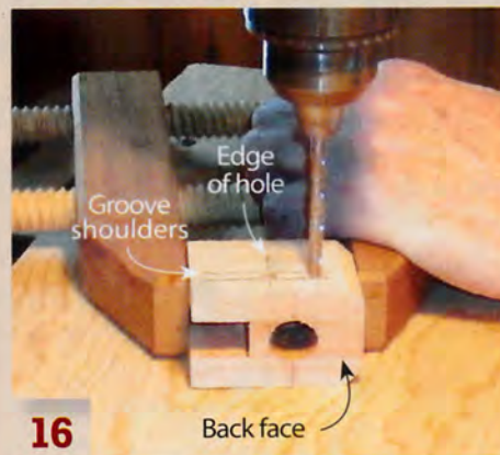
16 Drill holes in the sliding jaw for the pins that will capture the screw in the hole drilled to house it.
