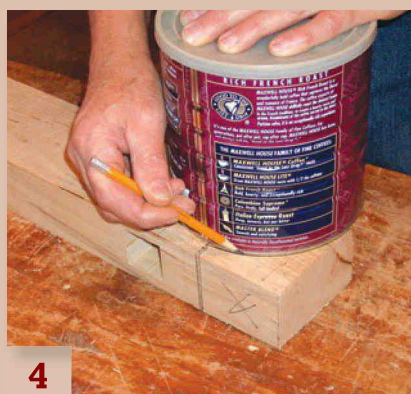
4 Use a coffee can to lay out the curves on the top of each foot after cutting a notch to establish its shoulder.
