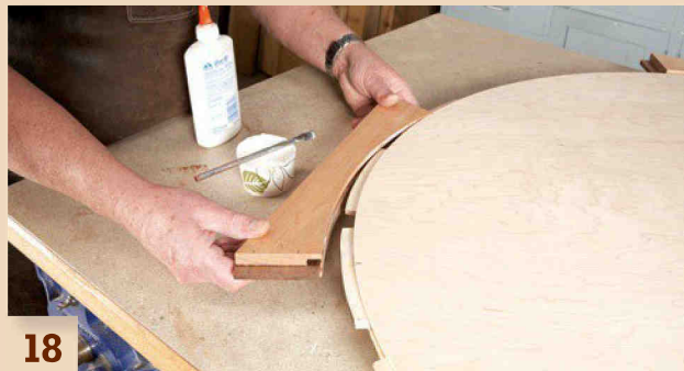
18 Glue just one segment onto the top. Let the glue dry before proceeding.
