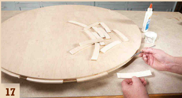
17 Glue the splines into the top.
