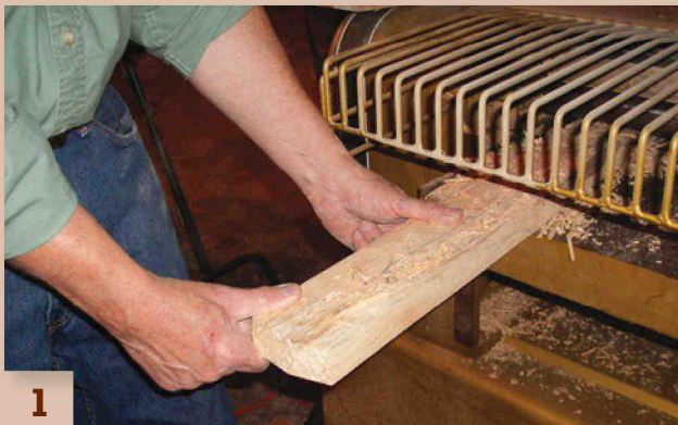
1 Mill 6/4 stock to make blanks for the trestle beams, feet and posts. These thick parts will be made by gluing together two blanks.
