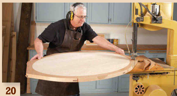
20 Saw the outer edge of the table. I use a circle-cutting jig for this operation, too. It leaves a smooth and even edge that's easy to clean up by sanding.
