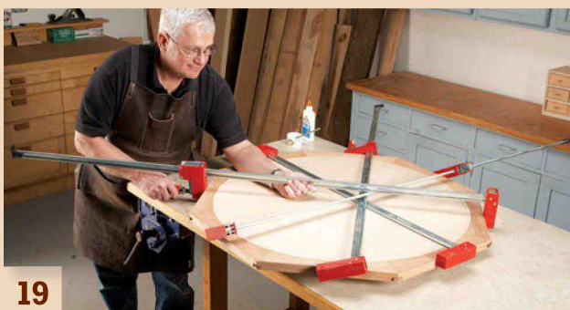
19 Glue two more segments, butting them up to the first piece. Add the remaining segments—without glue—to force the new pieces into position. Let the glue dry, then add two more, and so on.
