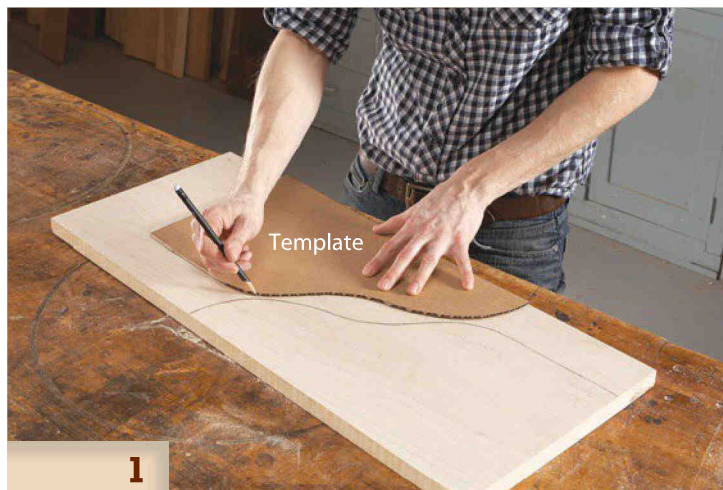
1 Lay out the sides of the box using a template. The curved profile comes from a magazine-storage box.
