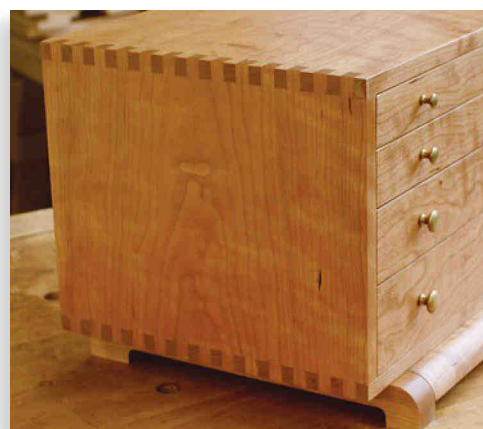
Box joints are ideal for joining thin boards at right angles, such as the 1/2" thick sides of this case.
