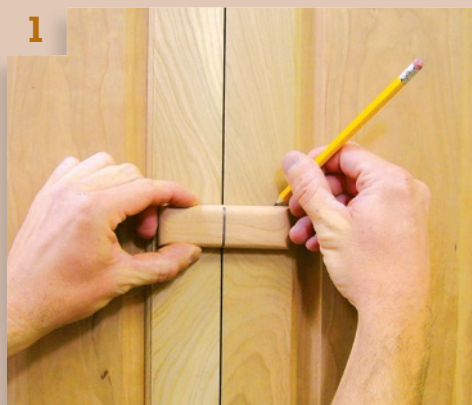
Position the handle on the cabinet and trace around it. At this point, the handle is a single block.
