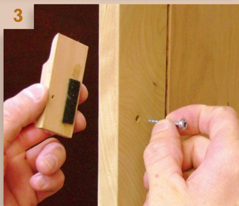
The left piece pivots on a screw. The right piece is fixed to the door.
