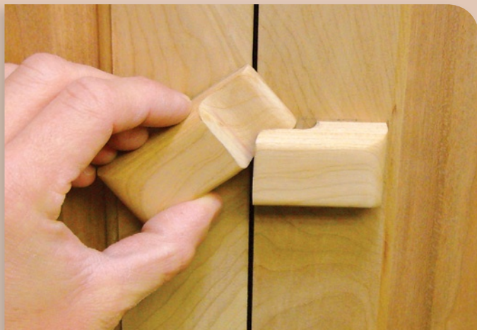
Position the handle on the cabinet and trace around it. At this point, the handle is a single block.
