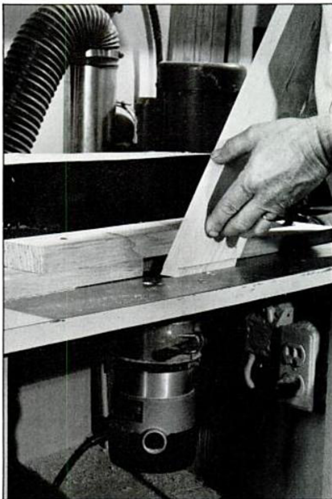
Cut the dovetails on the legs on a router table before you cut out the shape of the legs.
