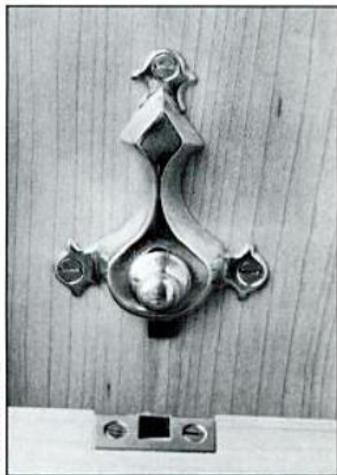
A brass catch fastens down the tabletop when horizontal and ornaments it when vertical.
