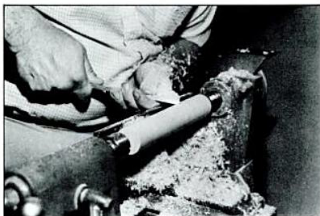
The planing cut shaves the long-grain surface smooth. Hold the skew long point up and angle the tool slightly in relation to the wood's axis. Cut between the center part of the edge and the short point, and keep the bevel rubbing as you cut.
