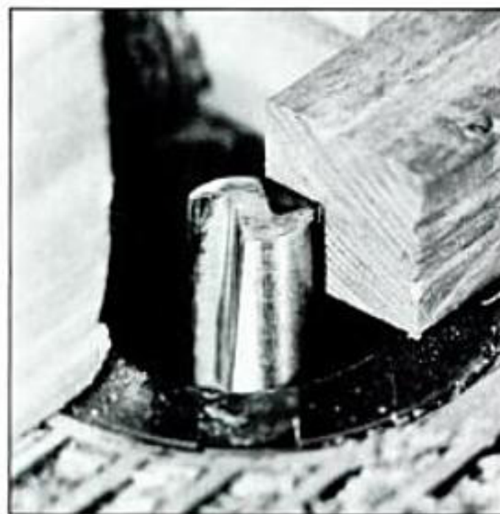
Cut the rabbet in the back of the frame pieces on a router table.
