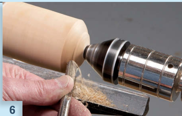
6 Form a dome on both ends of the cylinder. You're done with this part of the rolling pin.
