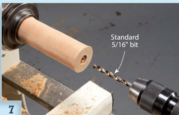
7 Rough out two blanks for the handles, then mount one in a scroll chuck. Drill a 5/8" dia. hole about 1/4" deep, then drill a 5/16" dia. hole as deep as your bit will go.
