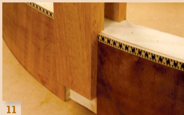
11 Trim overhanging veneer at the bridle joints. Make the legs and fit them to the apron.
