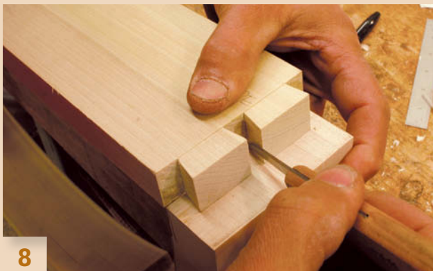
8 Cut large half-blind dovetails to join the back rail to the apron. Card tables of the Federal period were moved around a lot, so strong joinery was essential.
