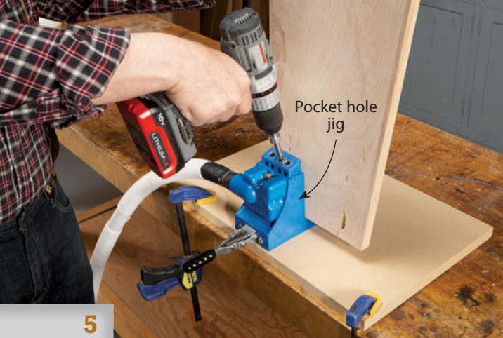
5 Drill pocket holes in the back legs and the back panel. Using both pocket screws and biscuits simplifies assembly.
