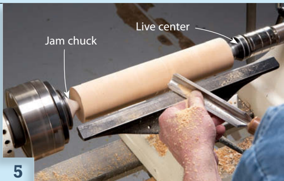
5 Mount the blank between the jam chuck and a cone-shaped live center, so it's perfectly centered on the drilled holes. Turn the blank into a true cylinder.
