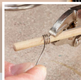
The "basket weave" design, first used by the turner Molly Winton, is made by coiling nichrome wire around a dowel or nail.
