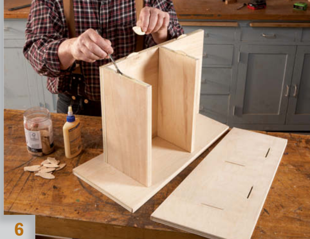
6 Assemble the bookshelf ends with biscuits and glue. Work on a flat surface and make sure the glued-up assembly is square.
