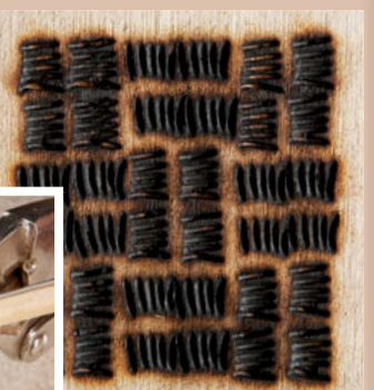
The "basket weave" design, first used by the turner Molly Winton, is made by coiling nichrome wire around a dowel or nail.
