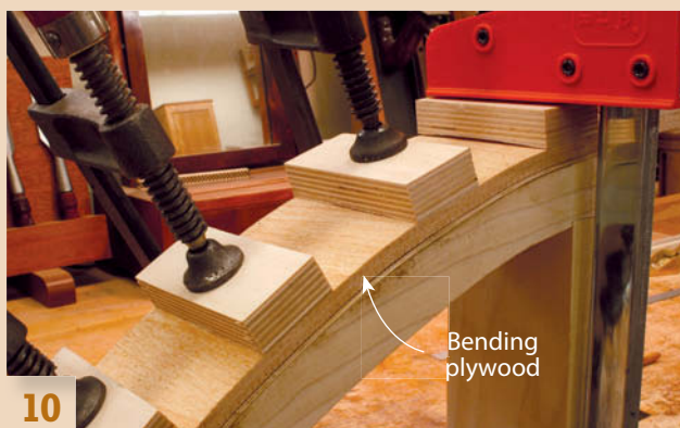
10 Glue the veneer to the apron using a caul made from bending plywood and glued-on blocks. The extra-thick veneer will form a smooth curve even if the apron has a small flat spot.
