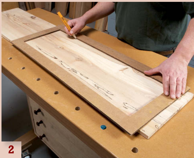
2 Outline the parts using cardboard "windows." These simple devices help you to visualize how the figure of each piece will look before crosscutting or ripping the boards.
