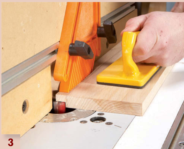
3 Rout a rabbet in the front edge of the sides. The door sits in these rabbets, making the sides appear thinner than they really are.
