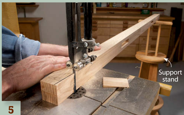
5 Taper the tops of the posts. The posts are almost 6 ft. long, so you'll need to support them with a stand that can be raised as high as your bandsaw's table.
