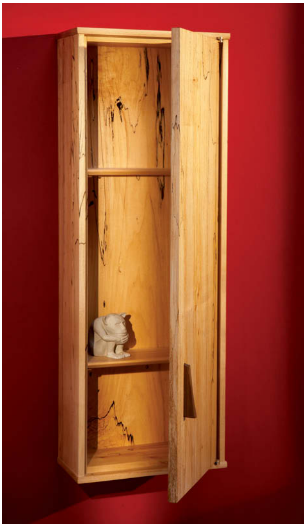
Measuring only 10" wide , this cabinet is designed to display the beauty of two wide boards: the door and the back.
