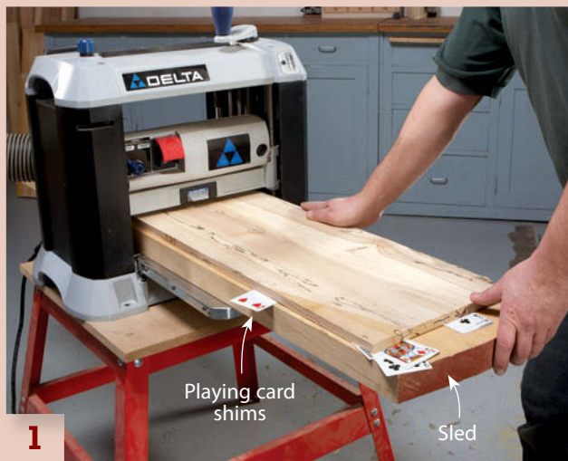
1 Flatten rough-sawn lumber as whole boards using your planer and a sled. This piece measures 10" across—wide enough for the cabinet's door, but probably too wide for your jointer.
