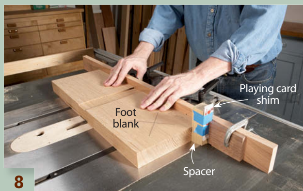
8 Cut dados on the feet to fit into the notches. The width of the dados must exactly match the thickness of the posts. Add playing cards, one at a time, to a spacer in order to gradually increase the dado's width.
