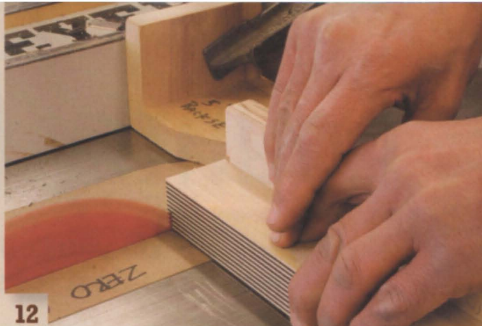
12 The bricks are then cut into chips. The 1/16" brick is sawn into 1/16" thick chips, the 1/8" brick into 1/8" chips. This produces a square, checkerboard pattern on the ends of the chips.
