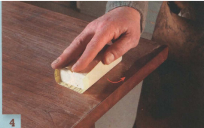
Sand to the ends using two or three short, light strokes, lifting at the end of each stroke so you don't cut through the edge.
