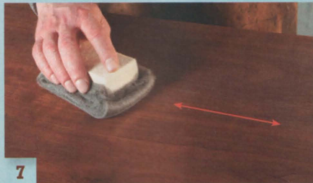
Remove the sandpaper scratches by working with the grain using the steel wool. Back the wool pad with the felt block to create a more consistent rubbing tool.
