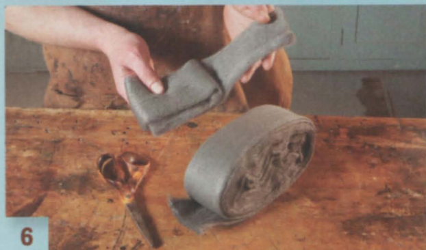
Carefully cut and fold good-quality #0000 steel wool to make a consistent abrasive pad. Folding the wool allows you to renew the cutting surface by unfolding fresh layers.
