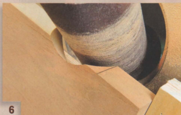
6 Stop sanding when the profile meets the line on the blank. Sanding the edge at 45° creates a cone-shaped profile.
