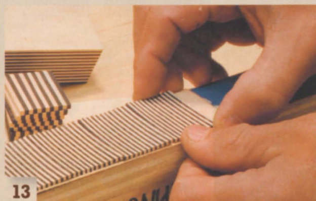
13 Glue the 1/16" chips on a strip of maple veneer and clamp the assembly between cauls. Make two of these.
