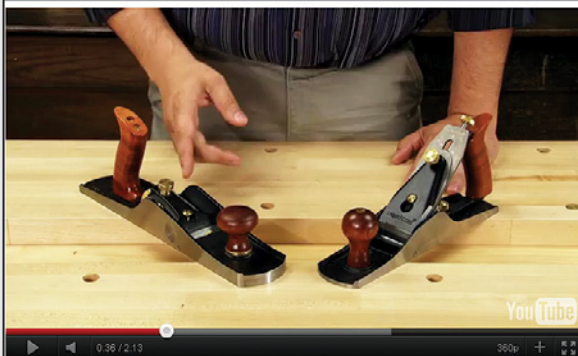
Bevel-Up Versus Bevel-Down Planes Explaining the difference between bevel-up and bevel-down planes
