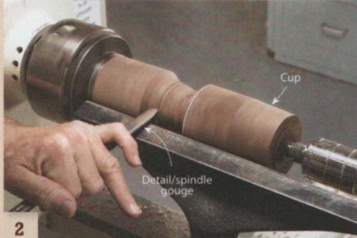
2 Cut in below a line marked to indicate the cup portion of the goblet to provide clearance for shaping the bottom of the cup.
