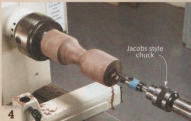
4 Drill the cup to within 1/2" of final depth, using a Jacobs style chuck mounted in the tailstock.
