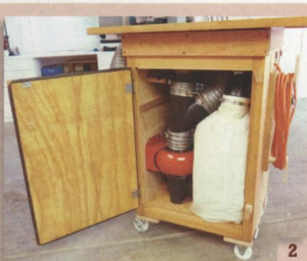
A mini dust collector resides inside the cabinet with ducting to the downdraft top and to an external port. Blast gates control the airflow.
