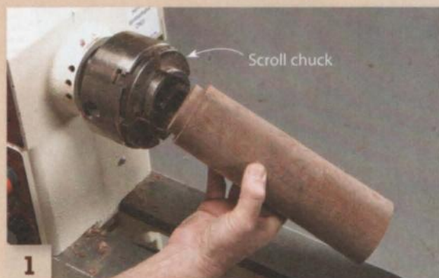
1 Securely mount a blank with a turned tenon into a scroll chuck. A secure mount comes from the tenon's large gripping surface and its shoulder, which rests on the top of the chuck's jaws.
