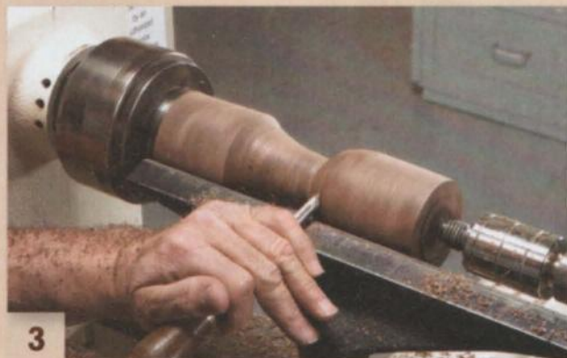
3 Shape the bottom portion of the cup with the detail/spindle gouge. Switch to the roughing gouge to refine the cup's flatter upper portion.
