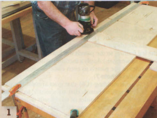
1 Begin by building a plywood box. Rout dados in its three vertical pieces to receive the top, bottom, shelf and back.
