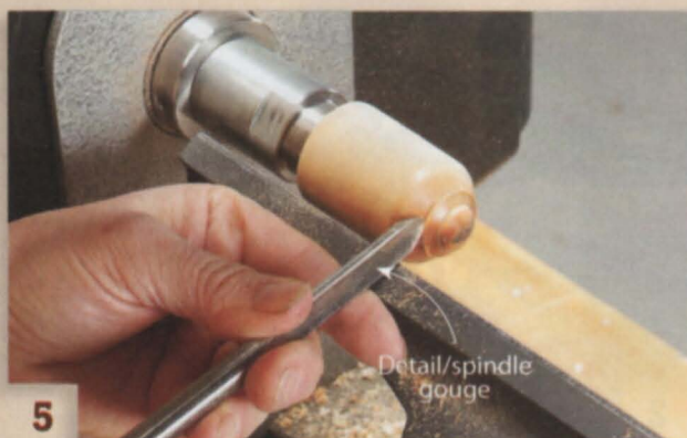
5 Shape the top of the blank using the detail/spindle gouge. A rounded top is comfortable to grip. Stepped details add interest.
