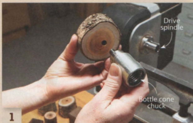
1 Mount the blank on a bottle cone chuck. Then mount the chuck on the drive spindle. This blank was cut from a buckthorn branch.
