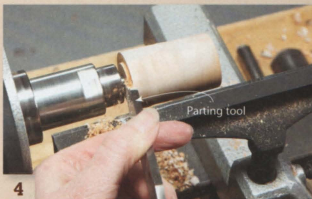
4 Cut the bottom of the blank at a slight angle using the parting tool. This creates a concave surface so the stopper's metal bottle cone will seat flush.
