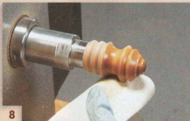
8 Use a soft cloth to apply three light coats of alcohol-resistant finish. Allow each coat to dry before recoating. Multiple light coats of finish always look better than one heavy coat.
