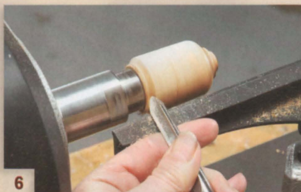
6 Round the bottom of the blank to meet the bottle cone chuck. This automatically matches the bottom of the blank with the top of the stopper's metal bottle cone.
